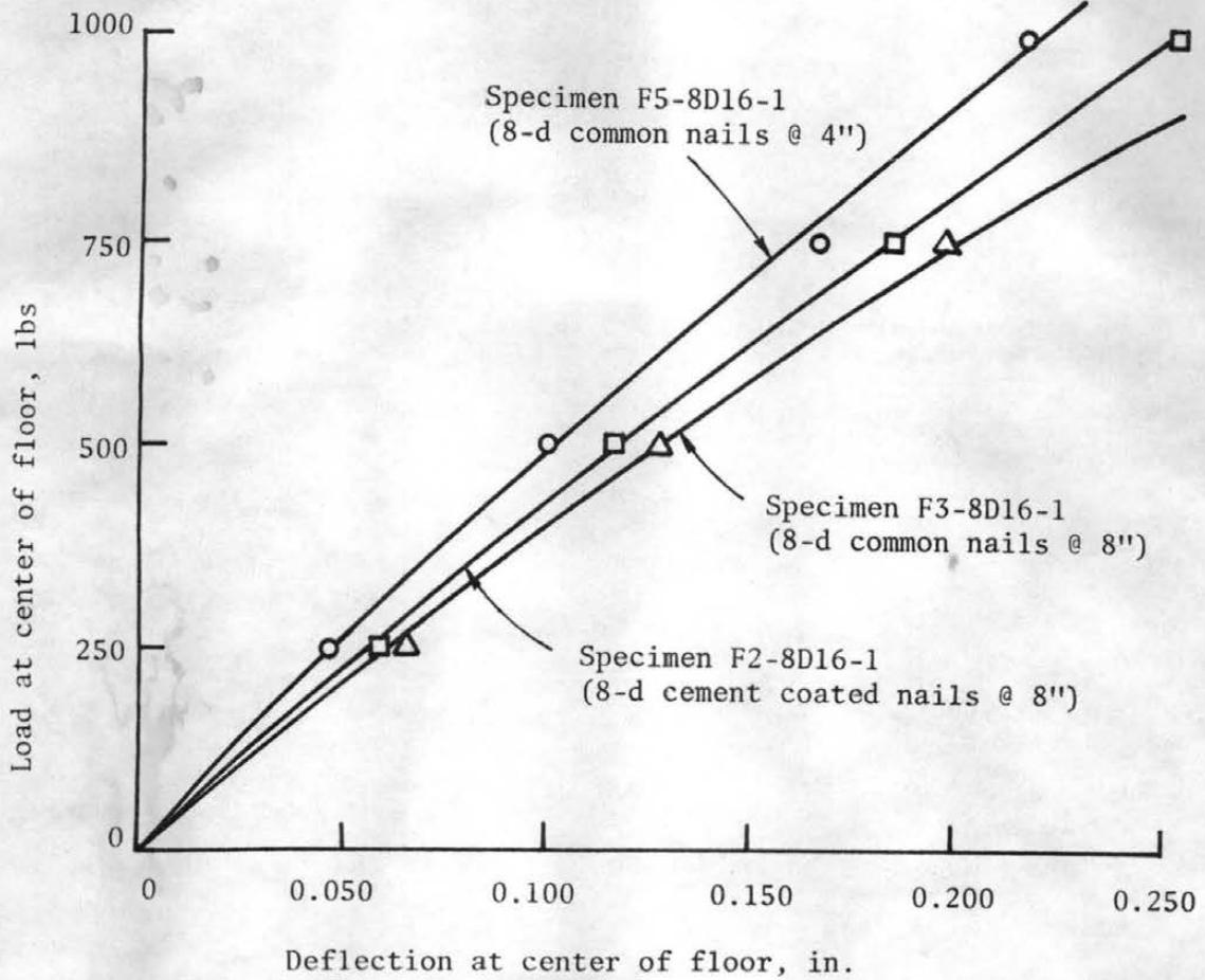
Figure 3.9 Effect of Nail Spacing
