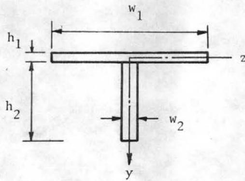
Figure 2.5 Layout and Sign Convention of T-Beam
