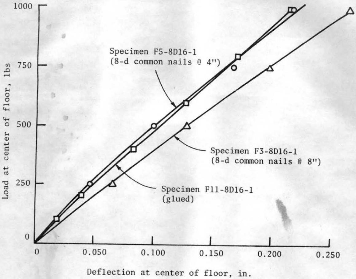
Figure 3.8 Effect of Type of Connector
