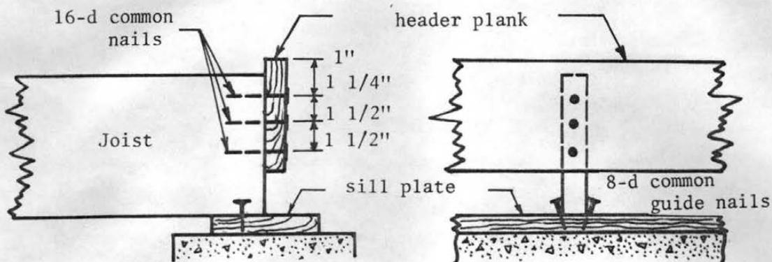
Figure 3.1 Detail of Joist Header Construction
