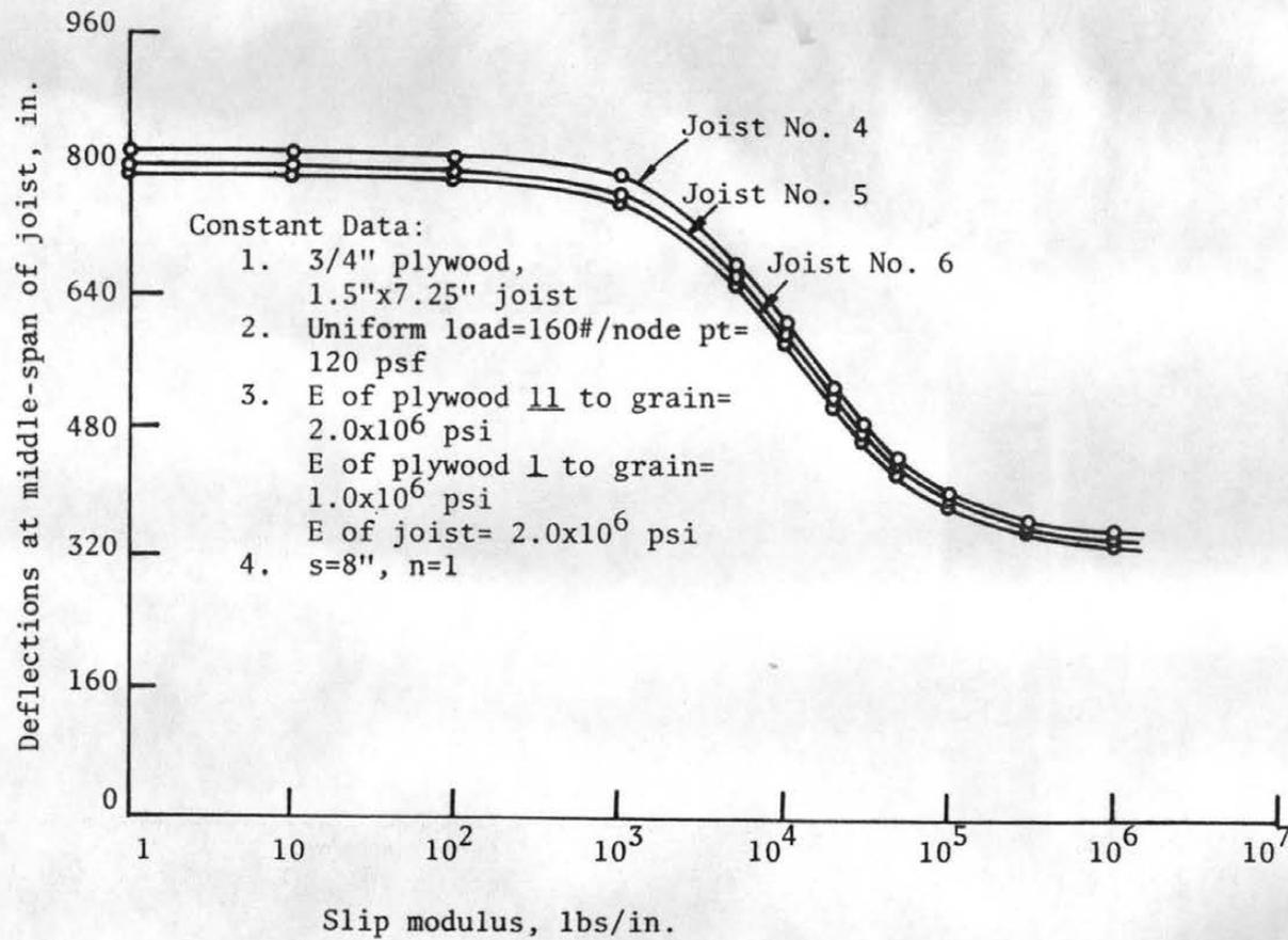
Figure 5.2 Deflections vs Slip Modulus, Uniform Load
