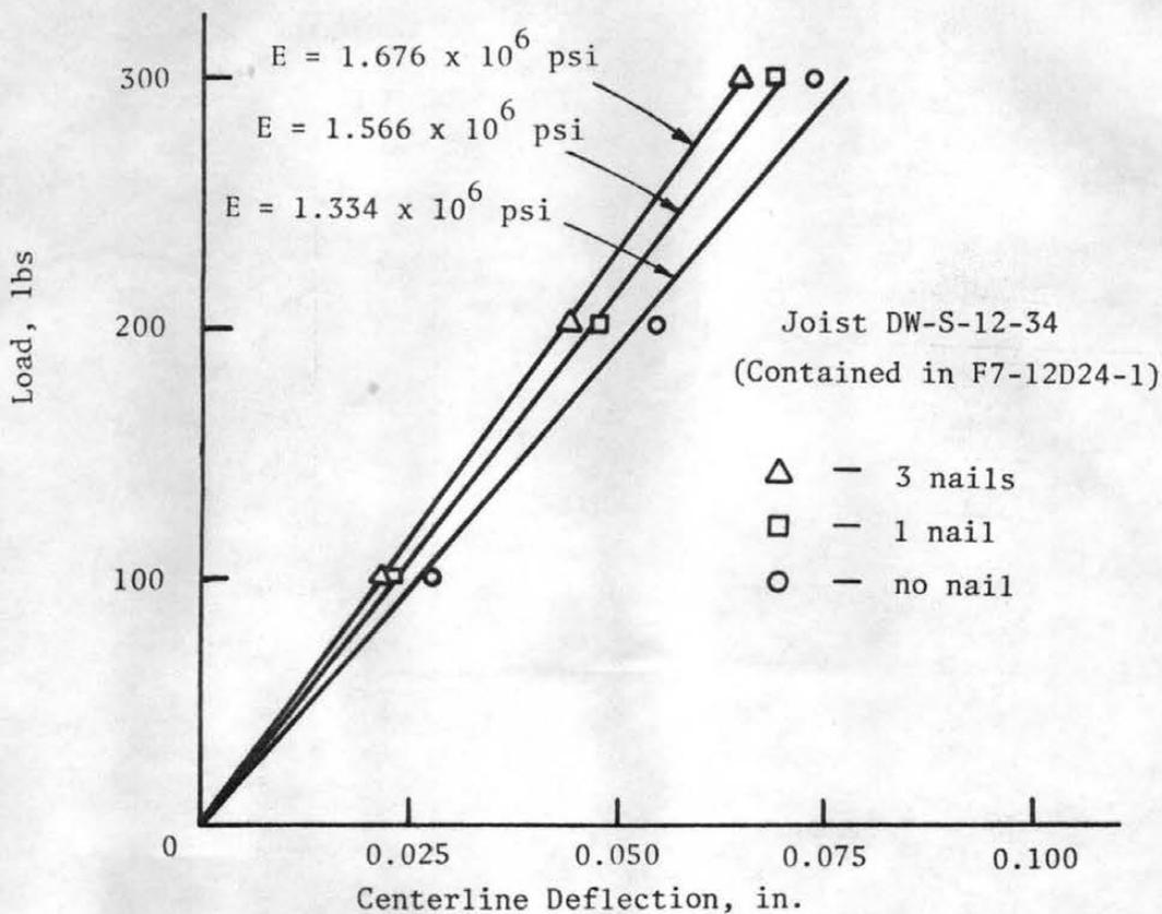
Figure 3.2 Typical Load-Deflection Plot for MOE Test
