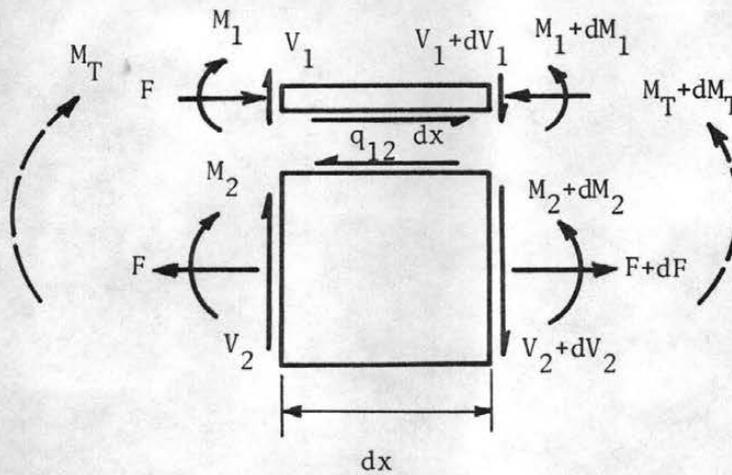
(b) Force components of a beam element
