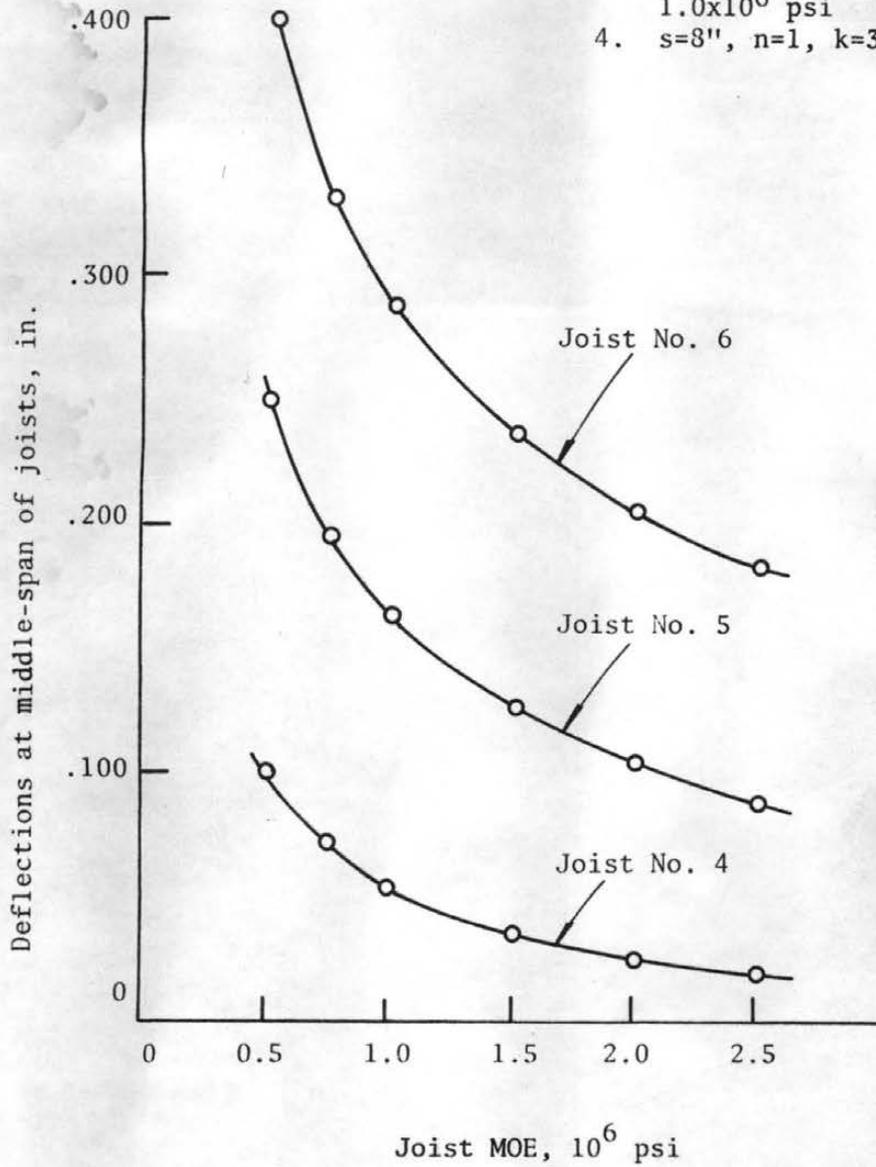
Figure 5.3 Joist MOE vs Deflections
