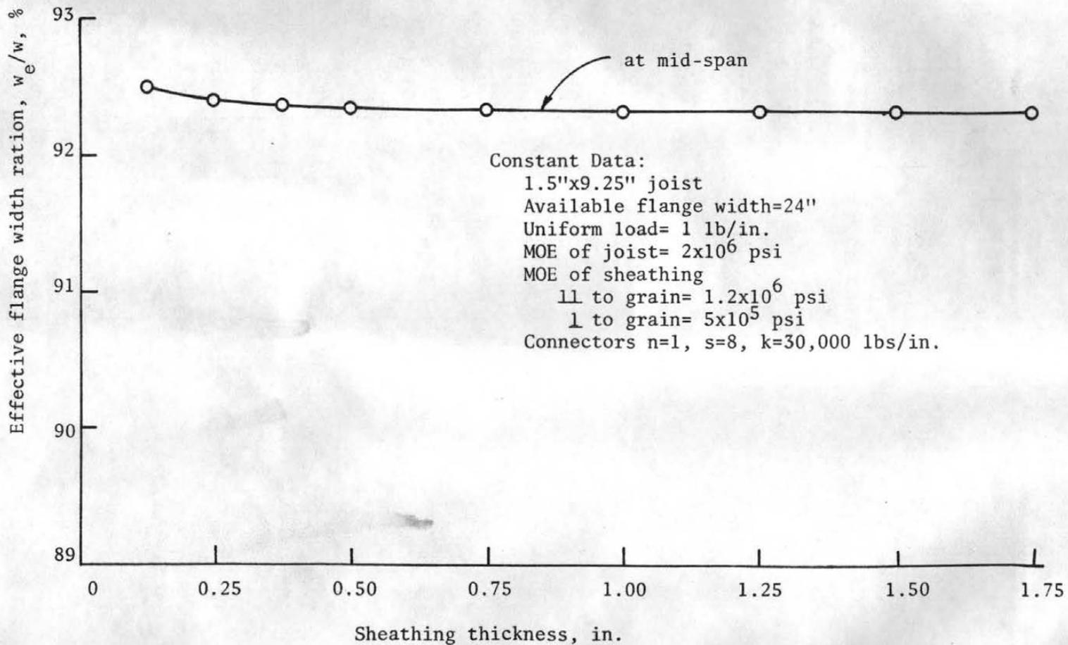
Figure 5.8 Effective Flange Width vs Sheathing Thickness, Uniform Load
