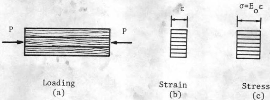
Figure 2.4 Strain and Stress Distributions Over the Transformed Cross Section of Plywood Subjected to Axial Compression
