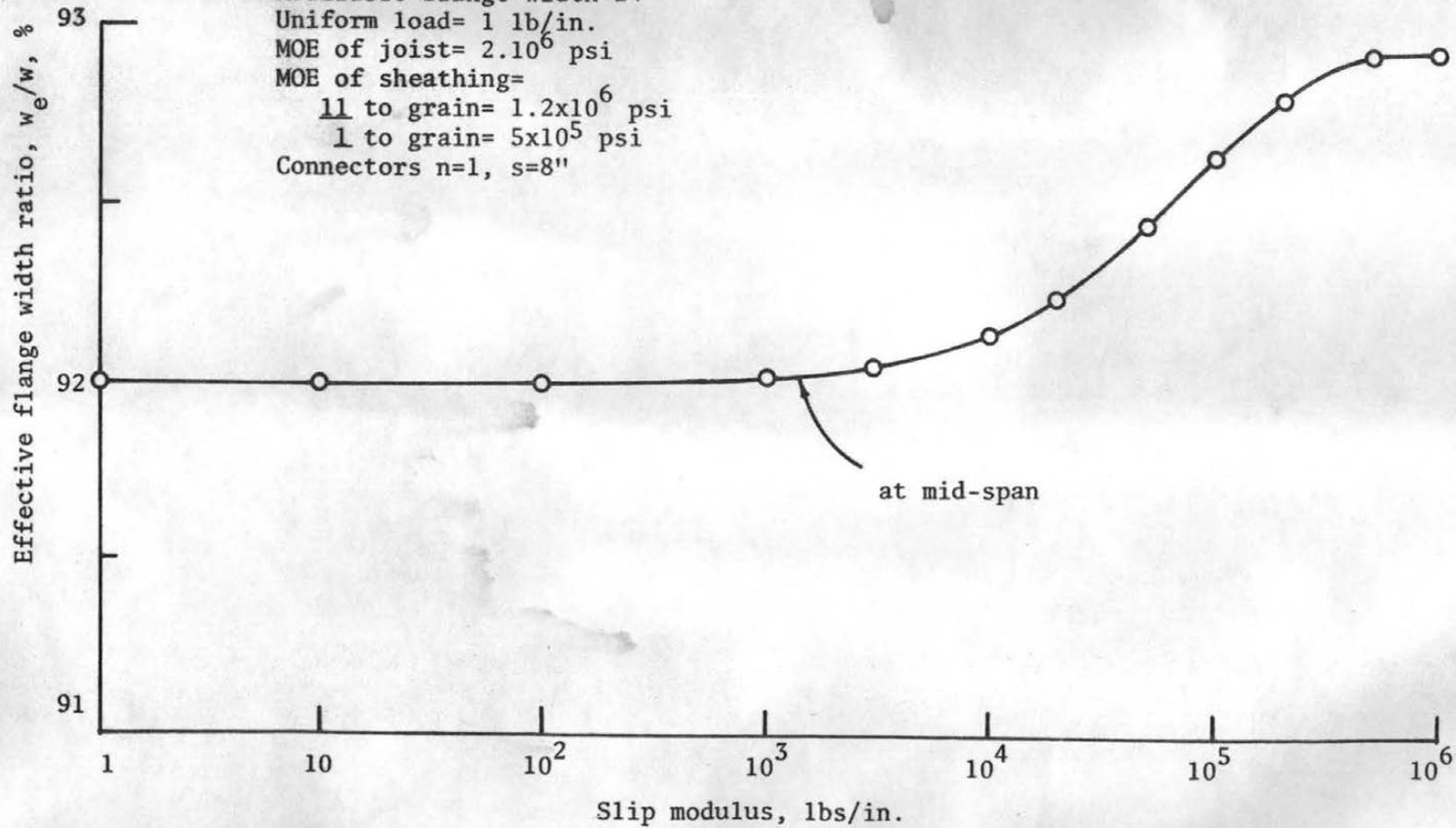
Figure 5.12 Effective Flange Width vs Slip Modulus, Uniform Load
