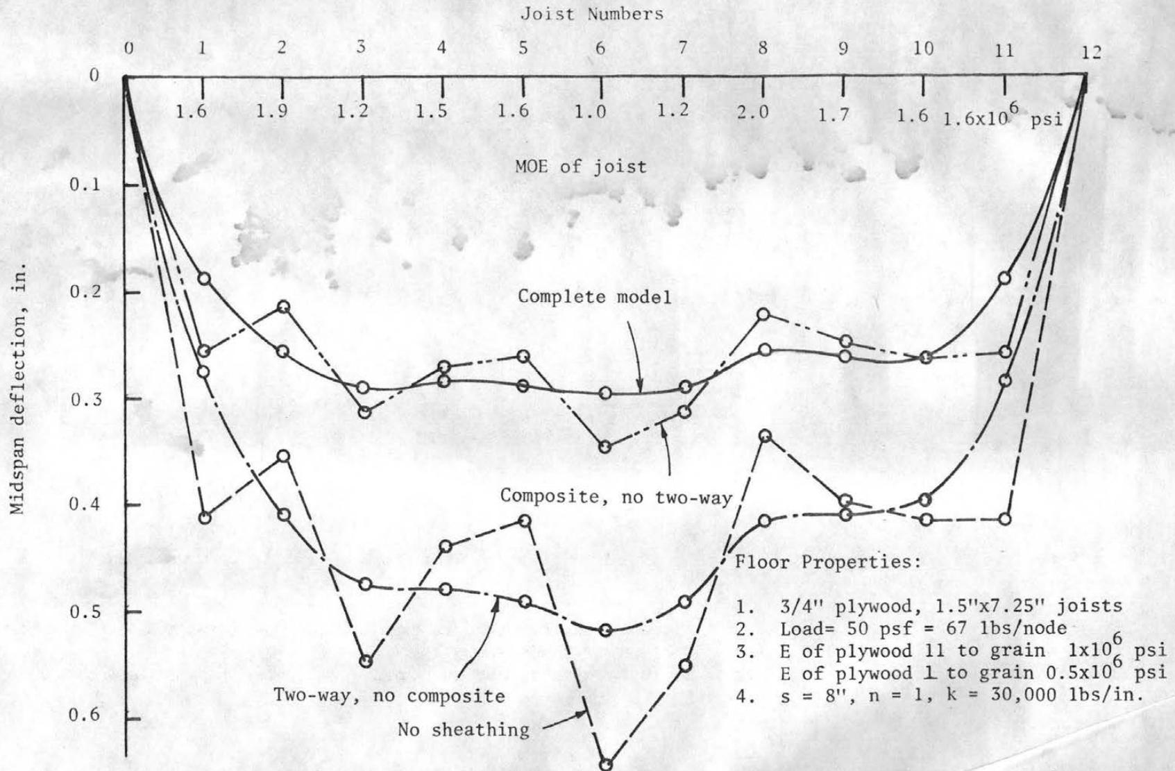
Figure 2.14 Deflection Curves of Limiting Cases for an Example Floor
