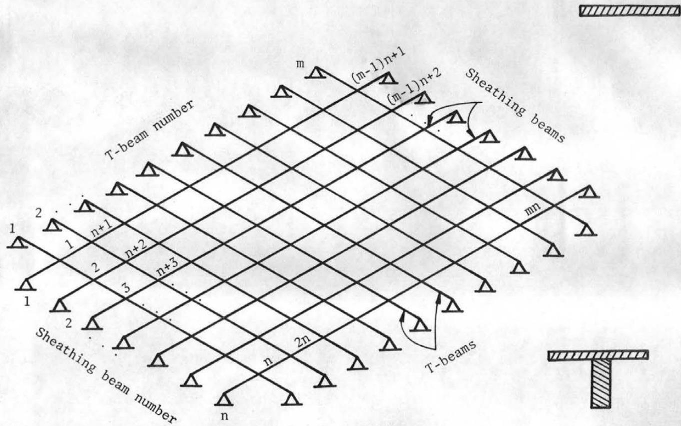
Figure 2.8 Physical Model of a Floor System
