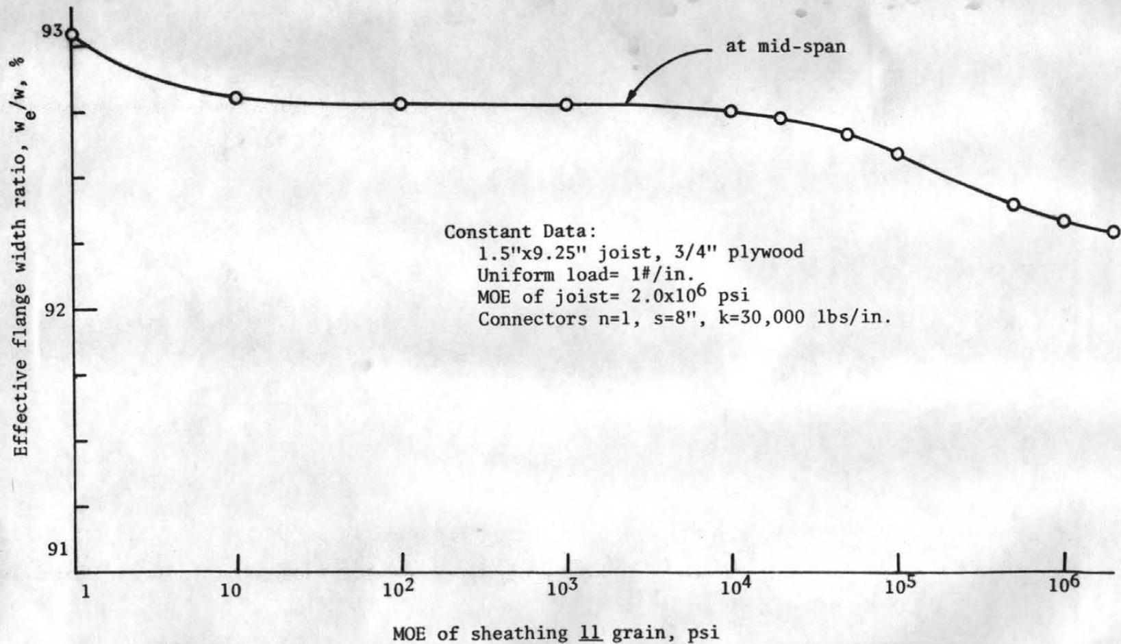
Figure 5.14 Effective Flange Width vs MOE of Sheathing, Uniform Load
