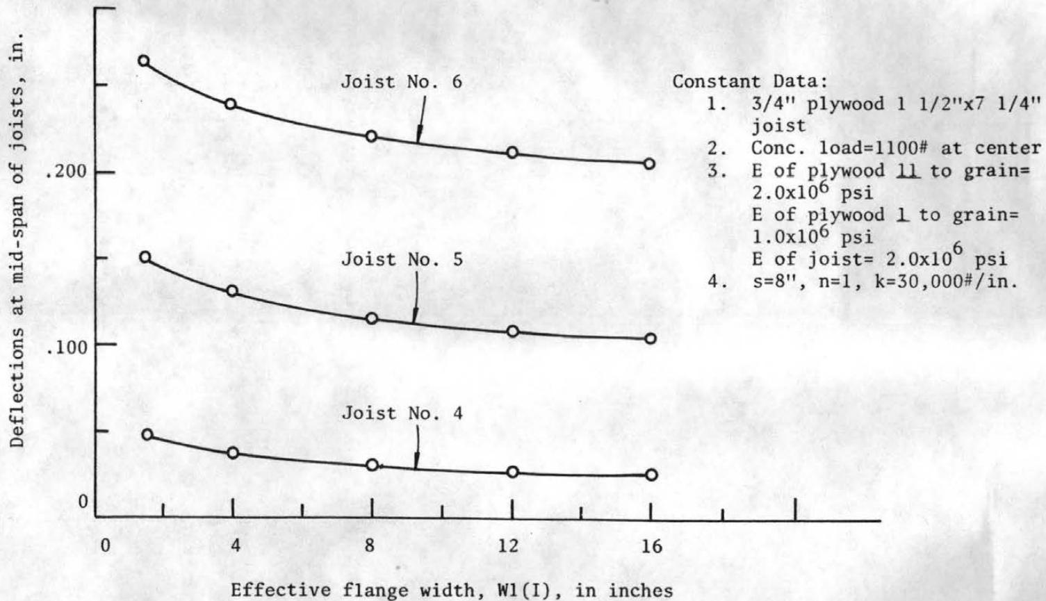
Figure 5.5 Effective Flange Width vs Deflections, Concentrated Load
