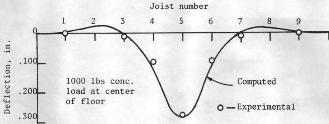
(a) Deflection profile at centerline of joists
