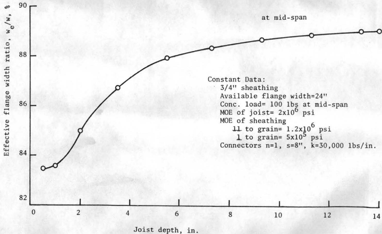
Figure 5.9 Effective Flange Width vs Joist Depth, Concentrated Load
