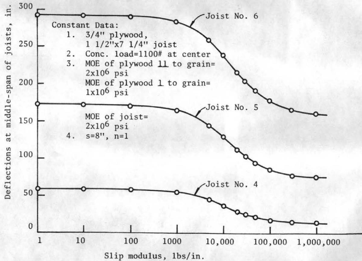
Figure 5.1 Deflections vs Slip Modulus, k, Concentrated Load
