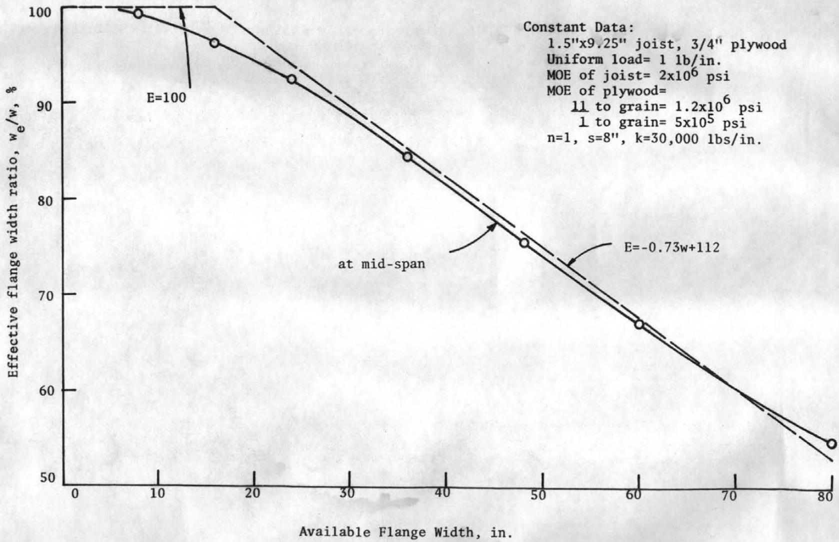
Figure 5.16 Effective Flange Width vs Available Flange Width, Uniform Load
