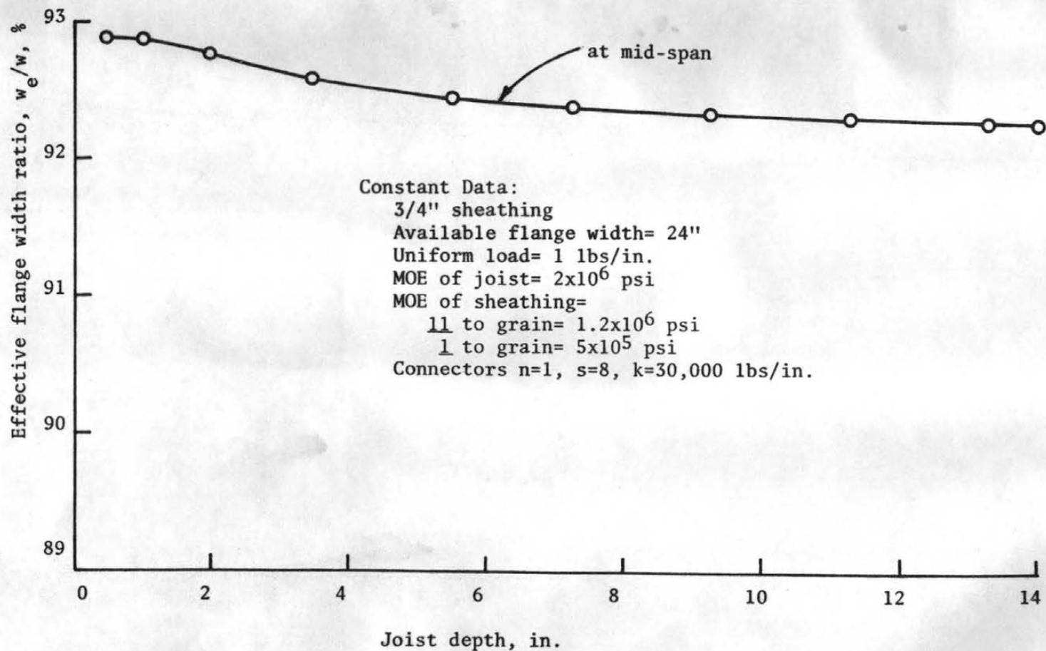
Figure 5.10 Effective Flange Width vs Joist Depth, Uniform Load
