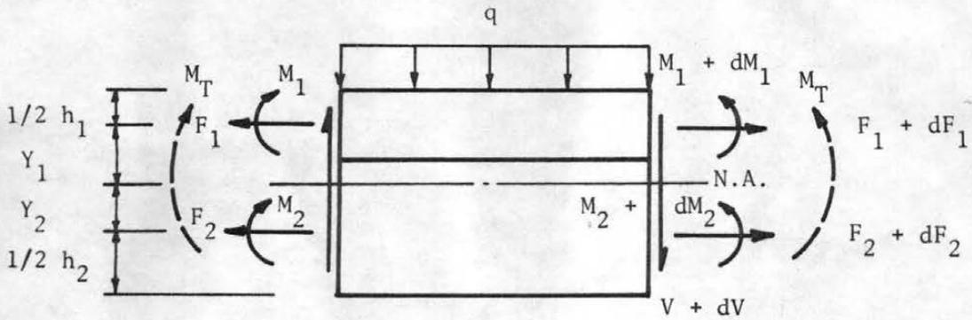
Figure 2.1 Two-Layer Beam System
