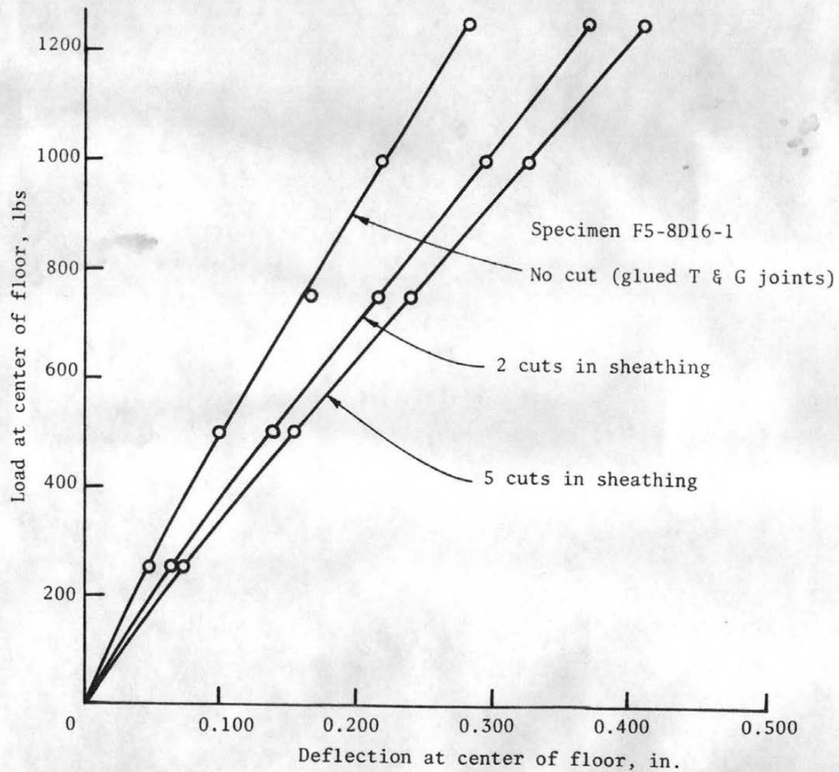
Figure 3.10 Effect of Gaps in the Sheathing
