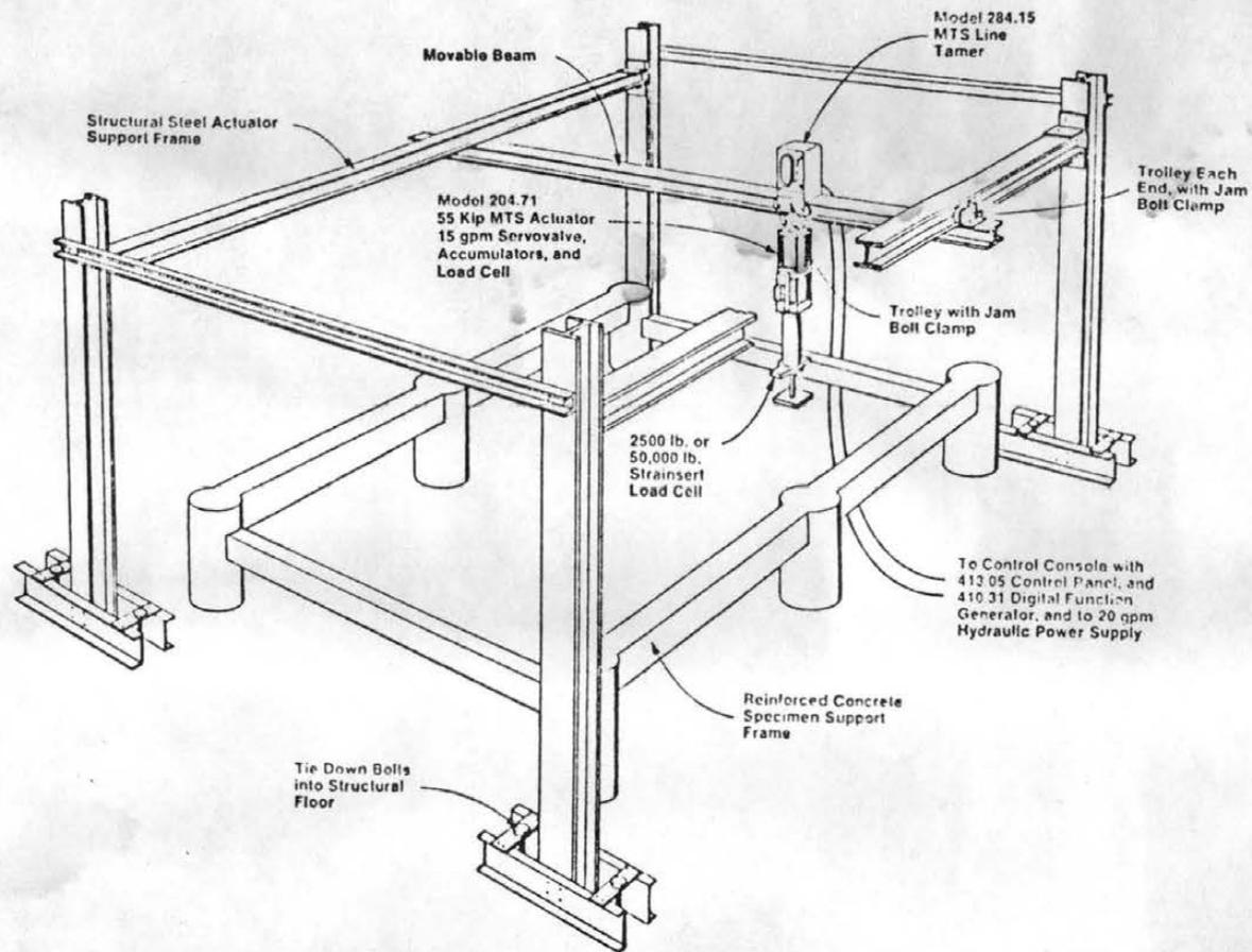
Figure 3.5 55-Kip MTS Loading Actuator and Support Frame
