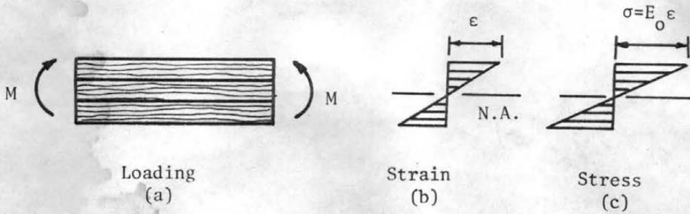
Figure 2.3 Strain and Stress Distributions Over the Transformed Cross Section of Plywood Subjected to Bending
