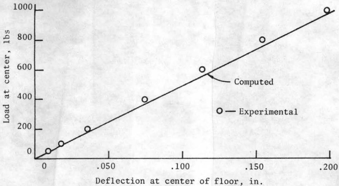
Figure D.17 Computed vs Measured Results of Floor Specimen F11-8D16-2 (Nails of Top Layer Not Driven into Joists)
