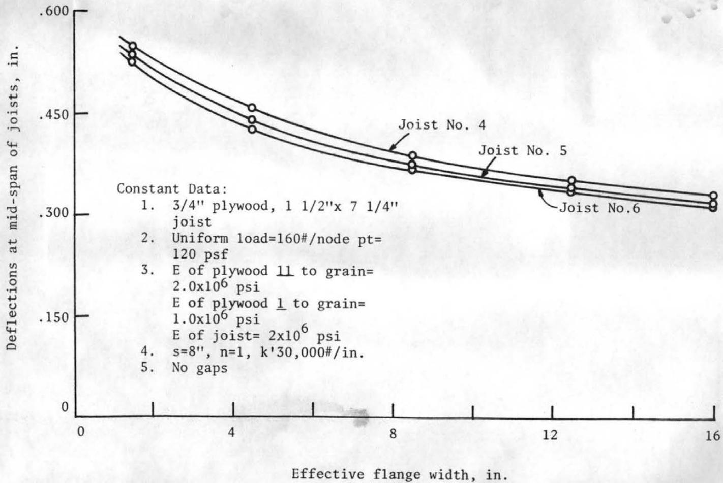
Figure 5.6 Effective Flange Width vs Deflections, Uniform Load
