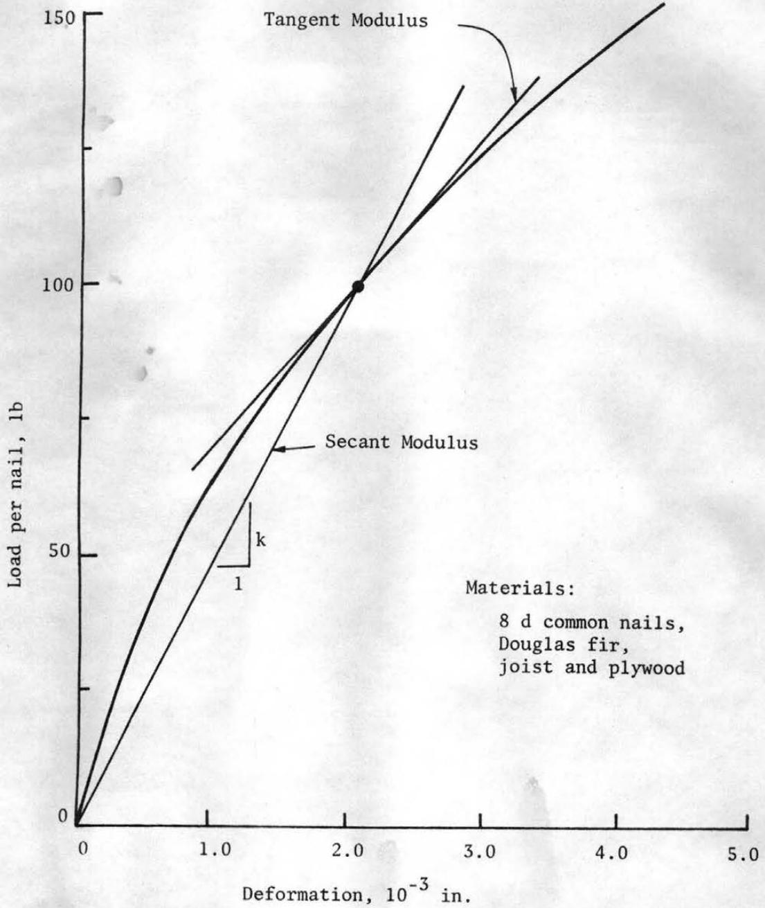
Figure 3.4 Typical Load-Slip Curve
