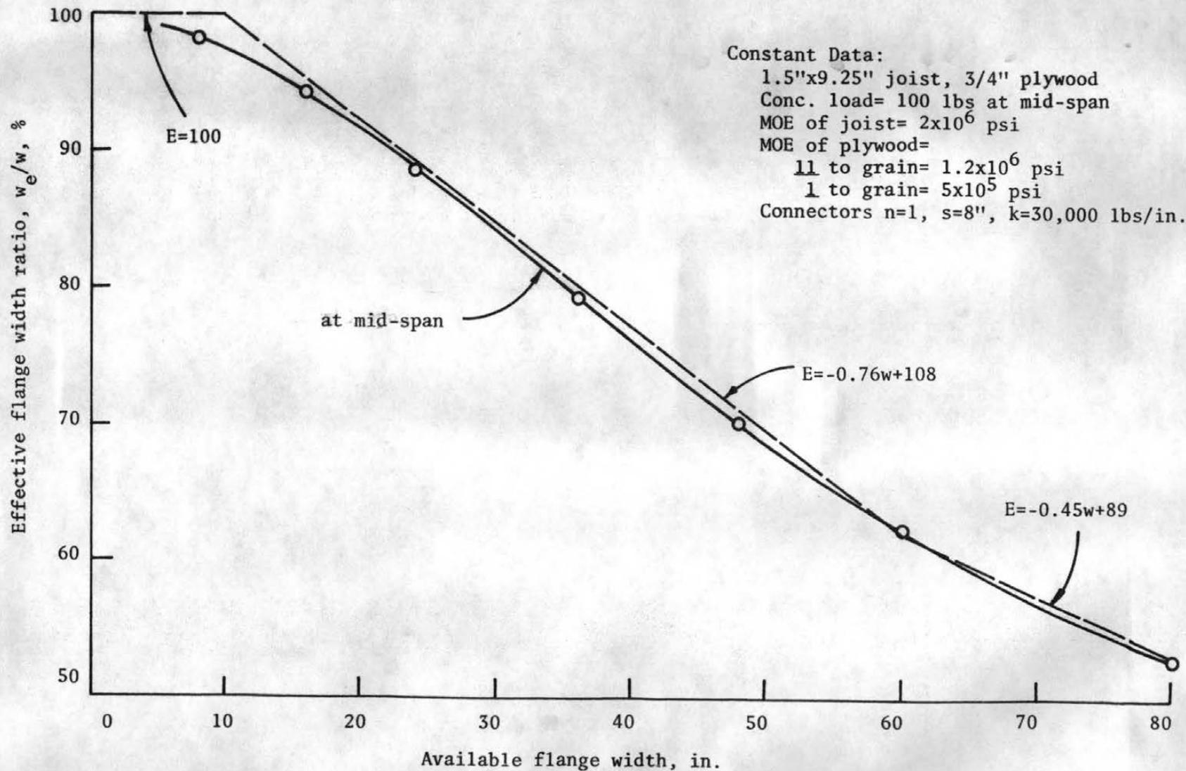
Figure 5.15 Effective Flange Width vs Available Flange Width, Concentrated Load
