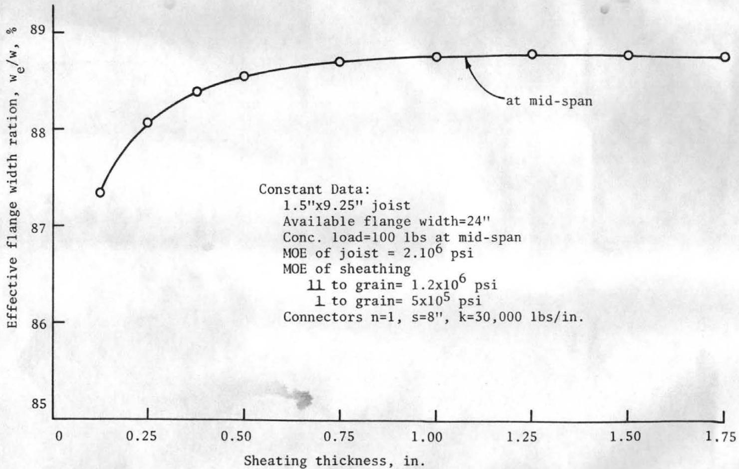
Figure 5.7 Effective Flange Width vs Sheathing Thickness, Concentrated Load
