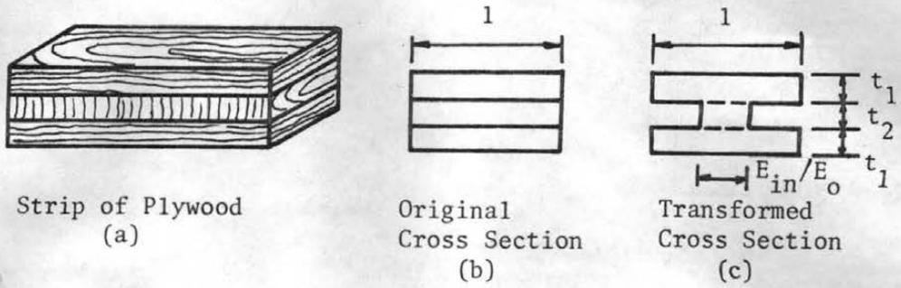
Figure 2.2 Original and Transformed Cross Sections of a Strip of 3-ply Plywood with Unit Width
