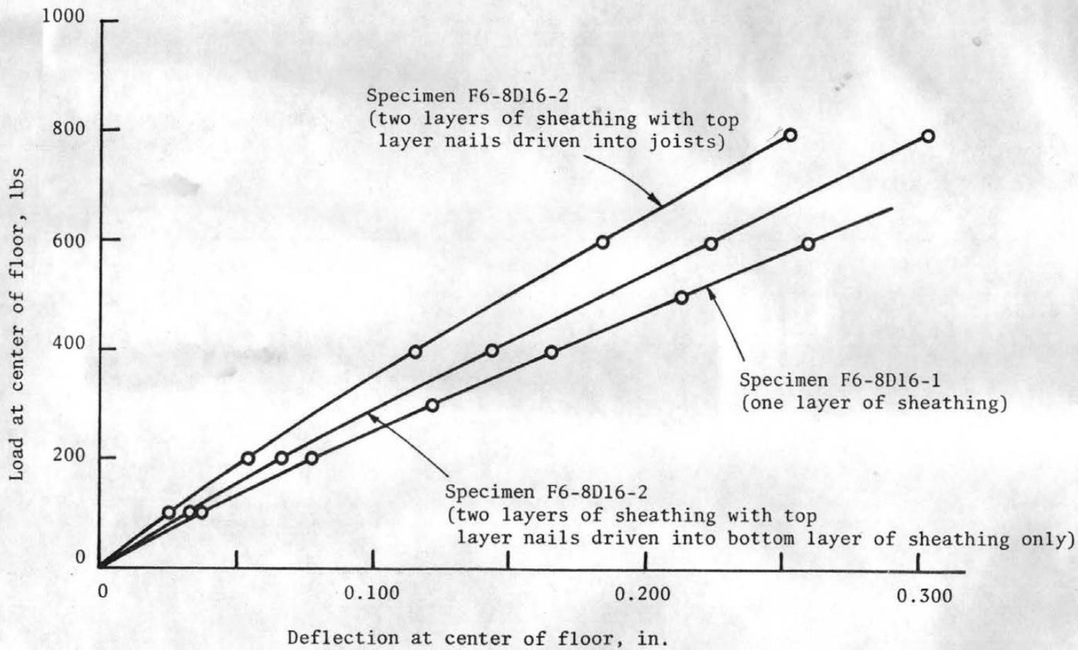
Figure 3.11 Deflection Behavior of a Floor as a Function of Number of Layers
