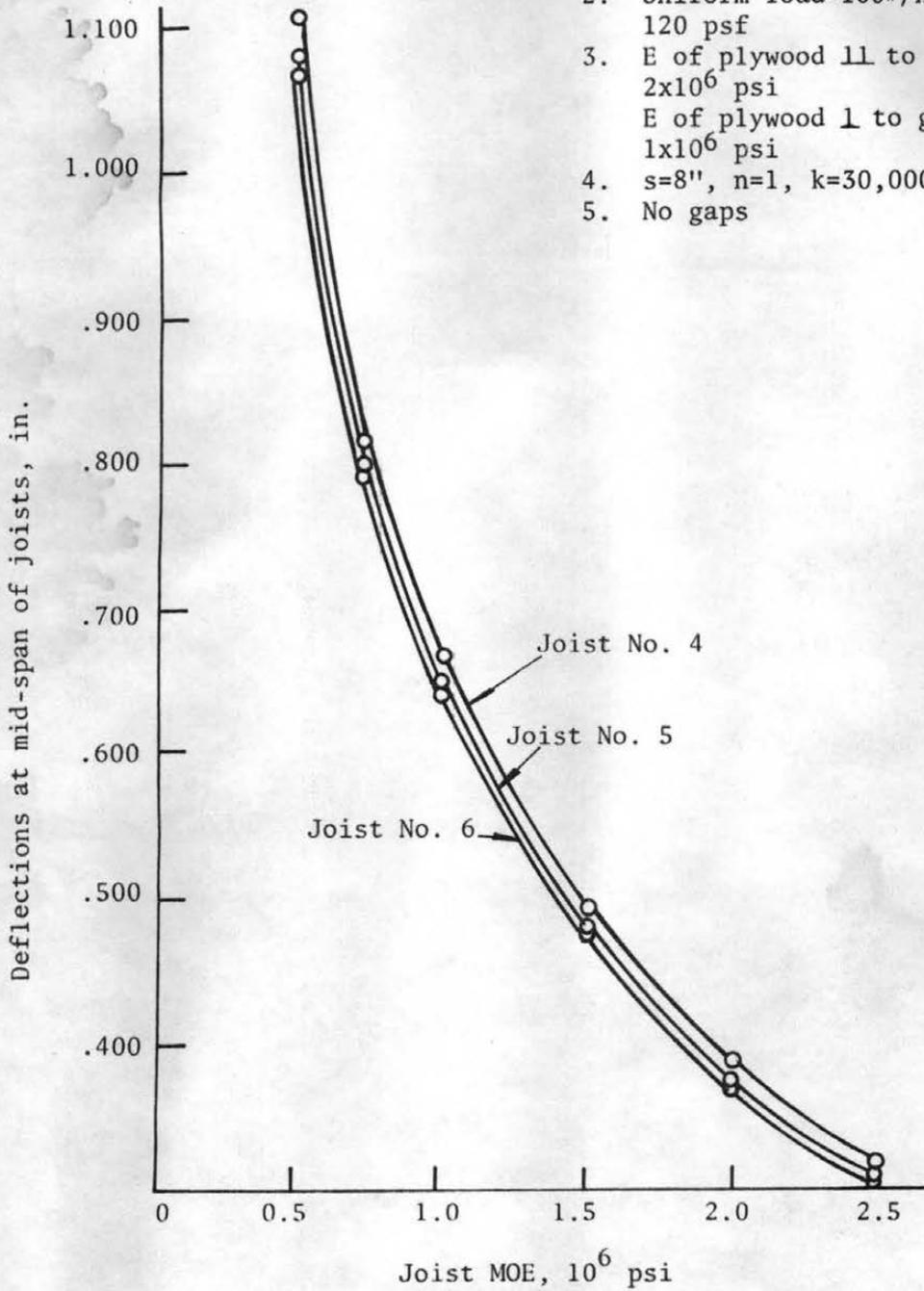
Figure 5.4 Joist MOE vs Deflections, Uniform Load
