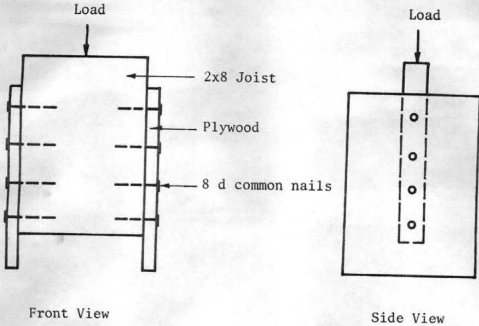
(a) Plywood and joist
