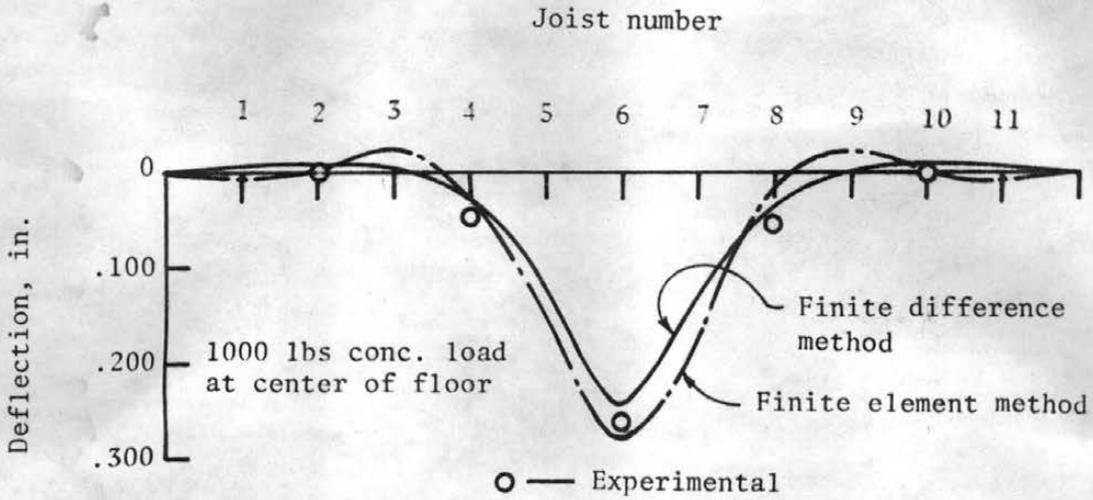
(a) Deflection profile at centerline of joists
