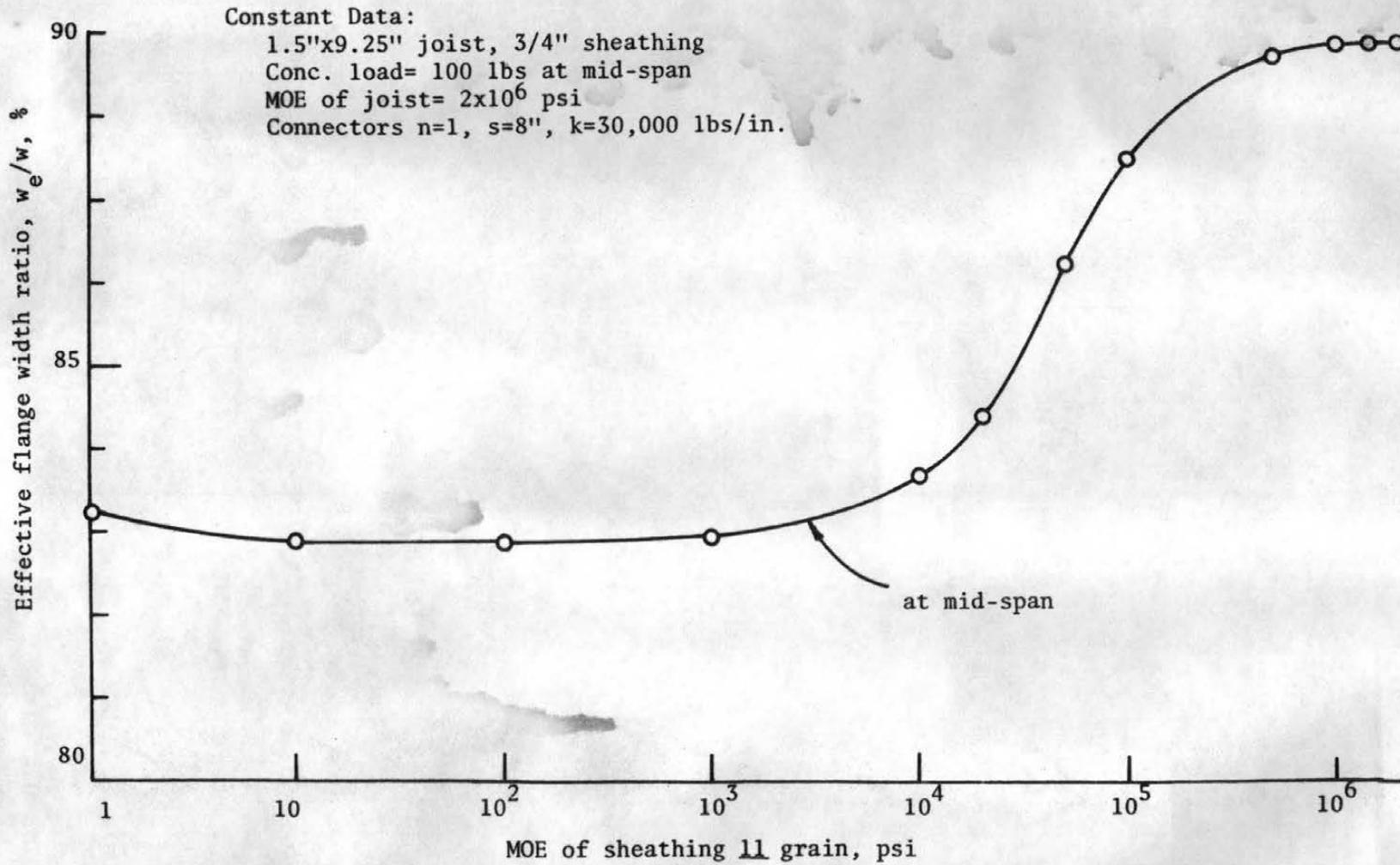
Figure 5.13 Effective Flange Width vs MOE of Sheathing, Concentrated Load
