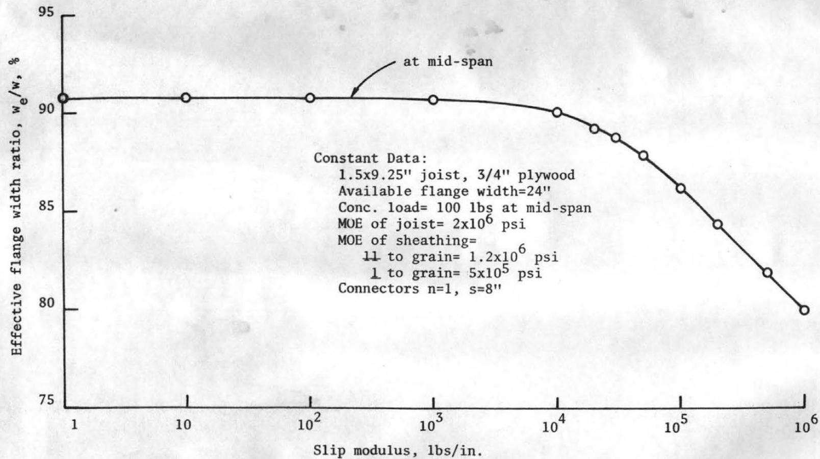
Figure 5.11 Effective Flange Width vs Slip Modulus, Concentrated Load
