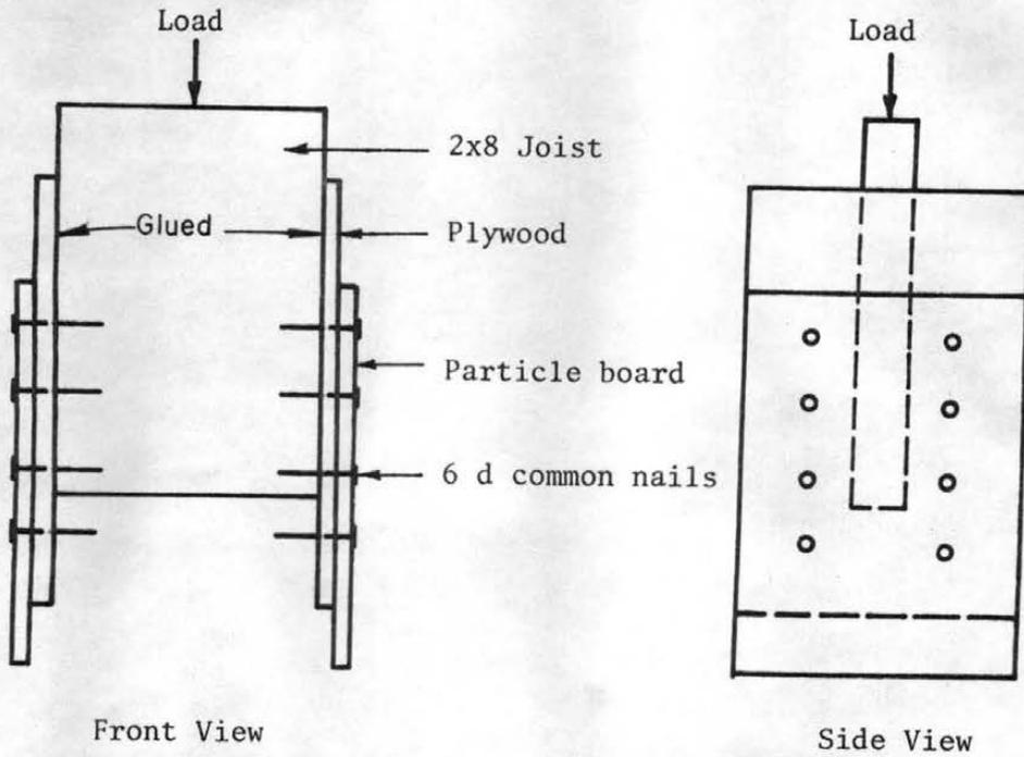
(b) Plywood and particle board
