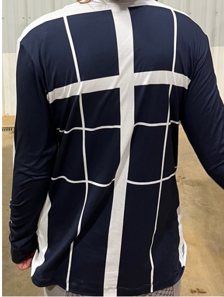
Figure 1. The fitted riding shirt with horizontal and vertical lines (The Equestrian "Straight Rider") from The Refined Rider worn by riders in the study to allow for upper body analysis. 2.6 Video Analysis
