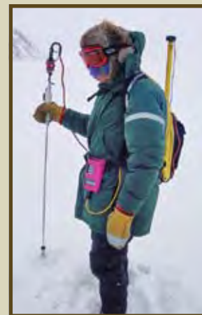
Figure 6. Measuring snow depth and GPS position using automated snow probes.
