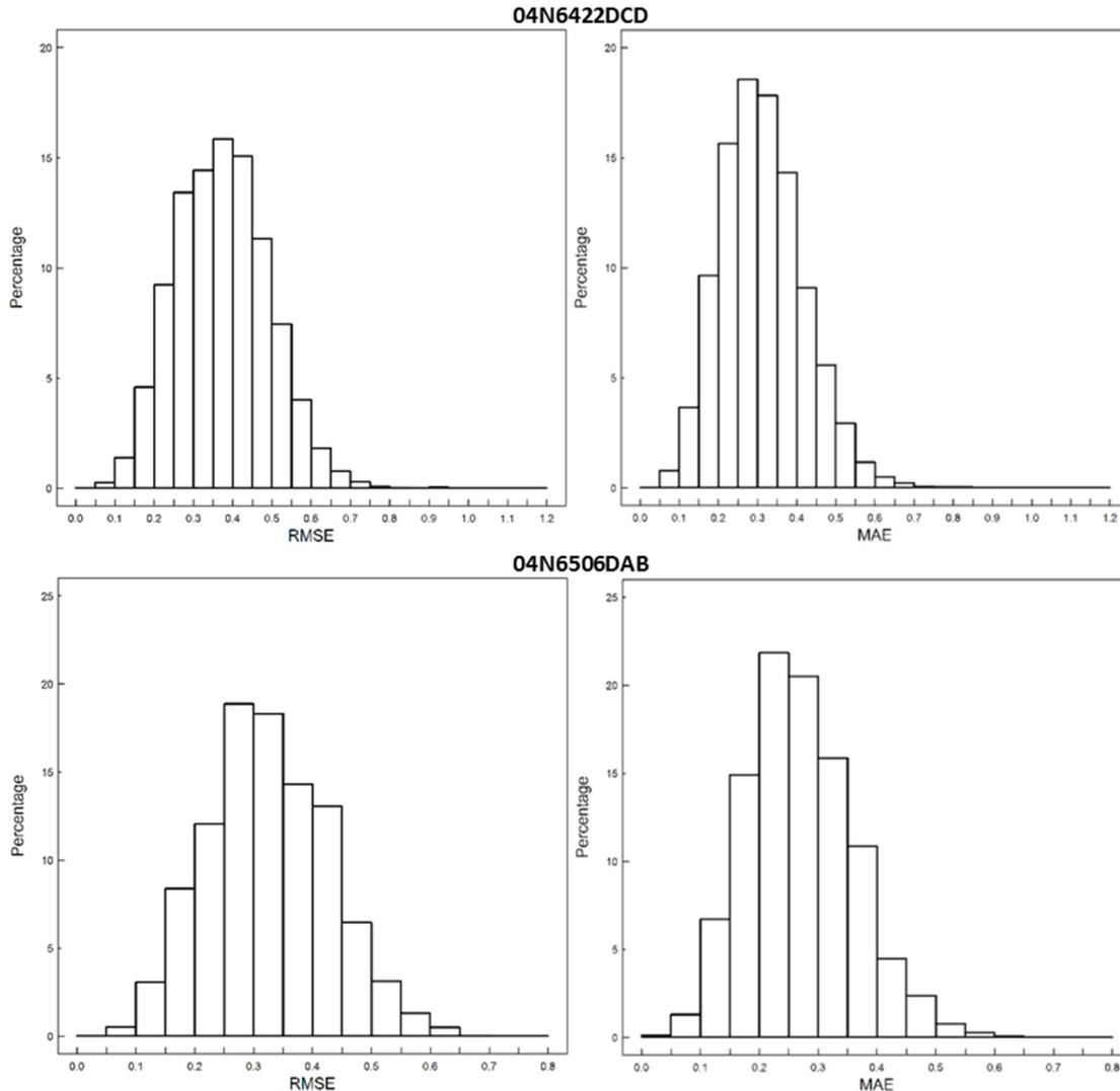
Figure 41: Relative density histograms of RMSE and MAE for wells 04N6422DCD and 04N6506DAB
