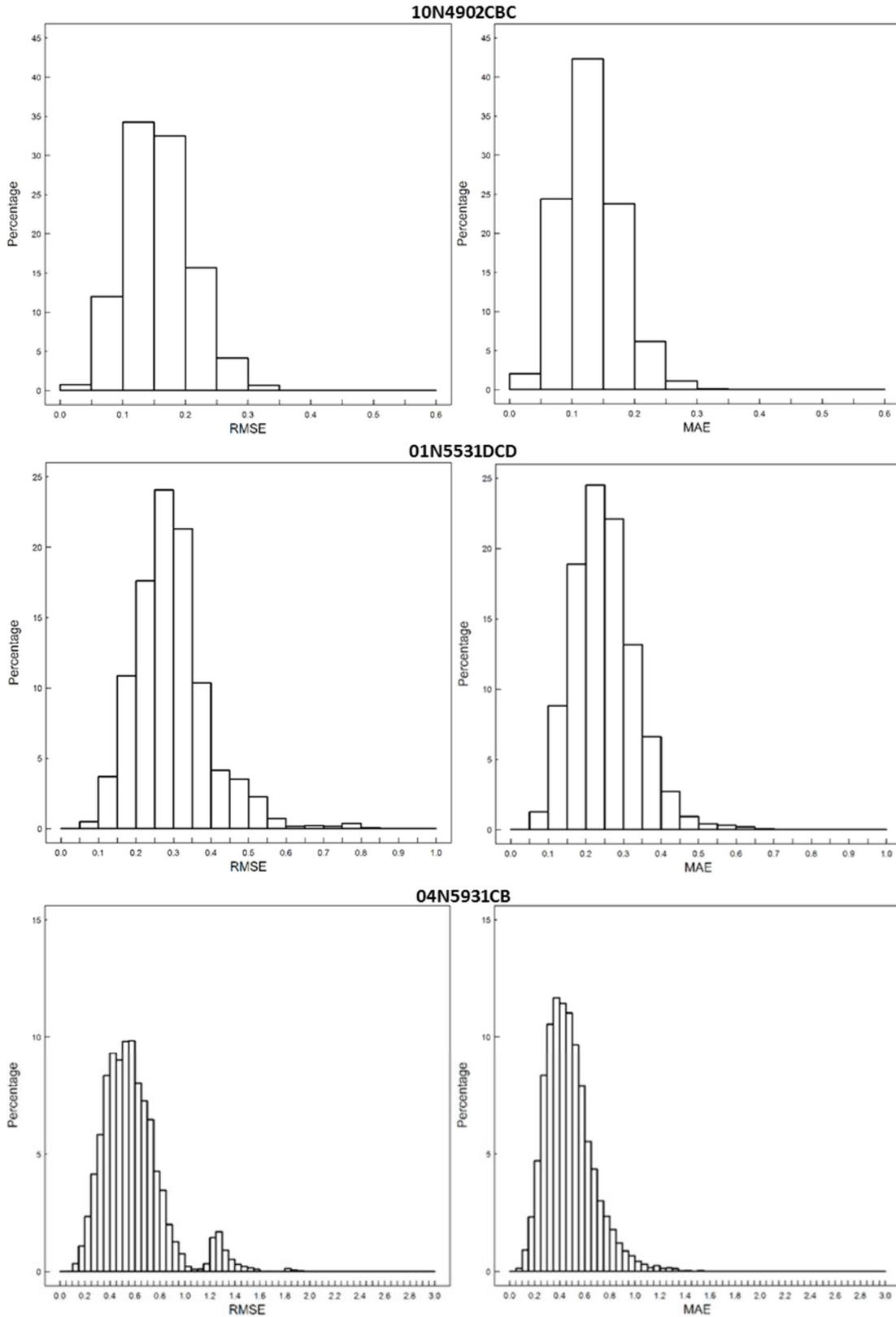
Figure 40: Relative density histograms of RMSE and MAE for wells 10N4902CBC, 01N5531DCD and 04N5931CB
