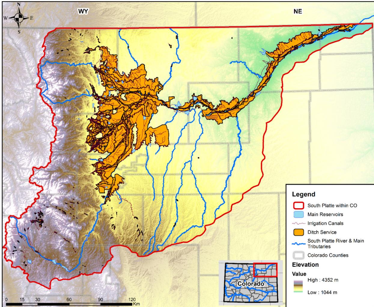
Figure 13: Ditch service areas, irrigation canals and main reservoirs within the South Platte basin
