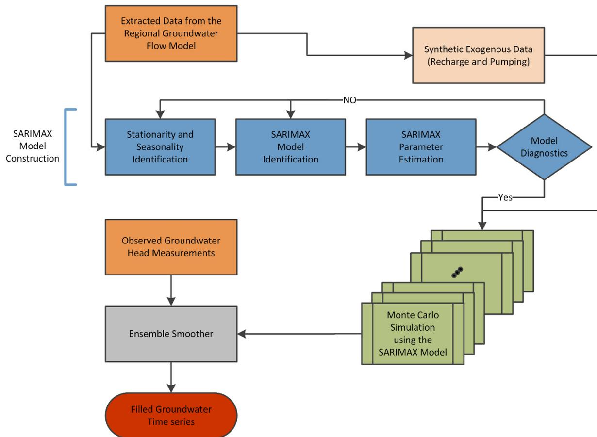
Figure 35: Groundwater Level Measurement Gap-filling Methodology
