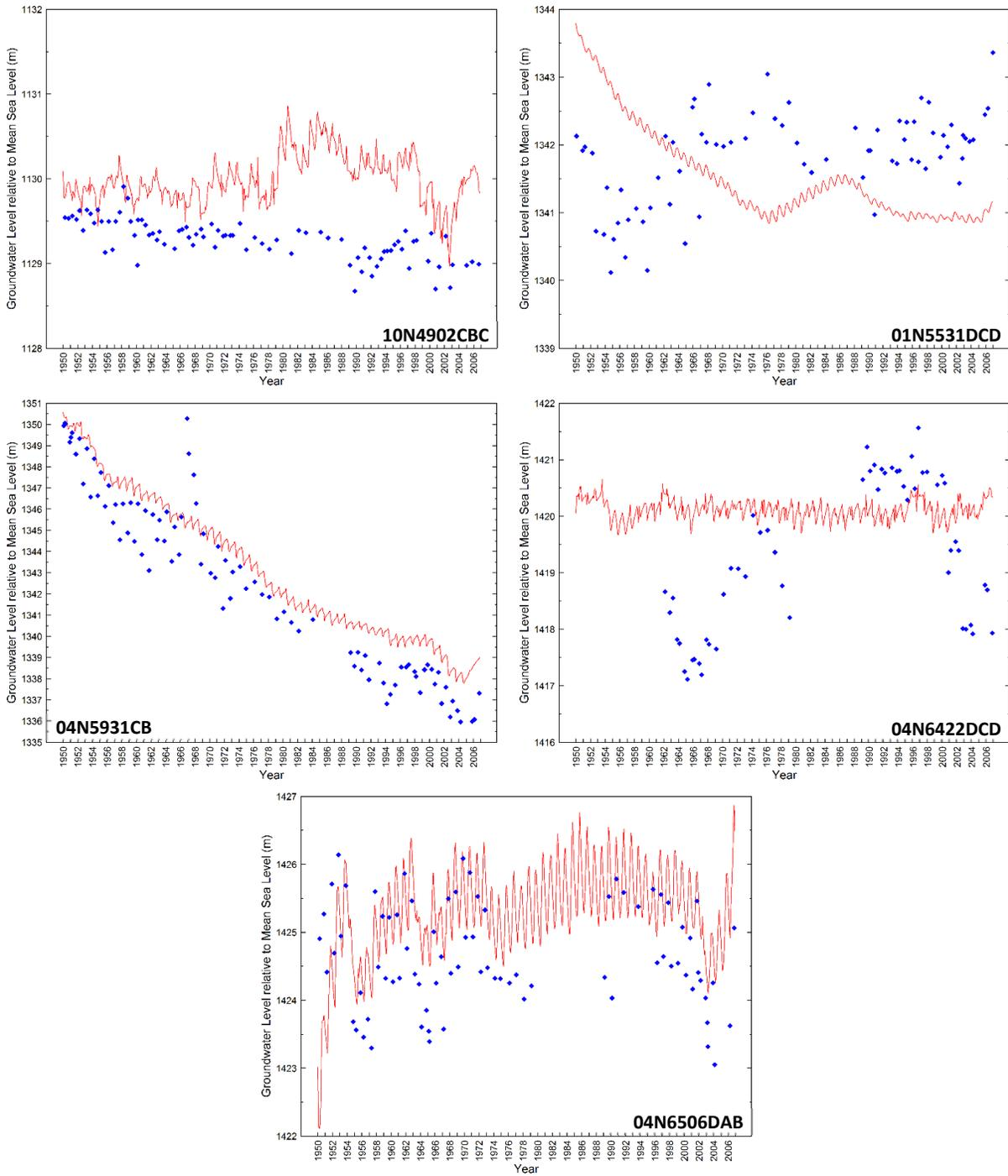
Figure 37: Modeled monthly groundwater level (red line) and biannual observed level (blue dots)
