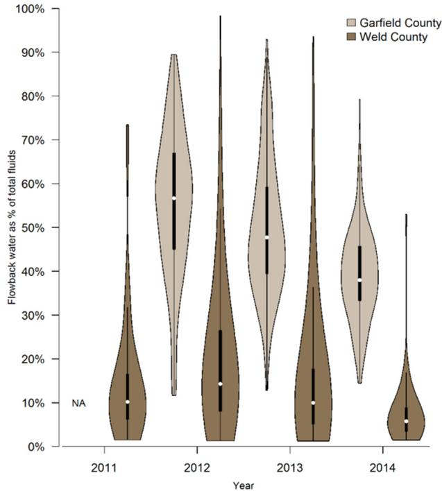
Figure 28: Flowback water as percentage of total fluids used and their rotated kernel densities on each side (NA: not enough data) (COGCC dataset)
