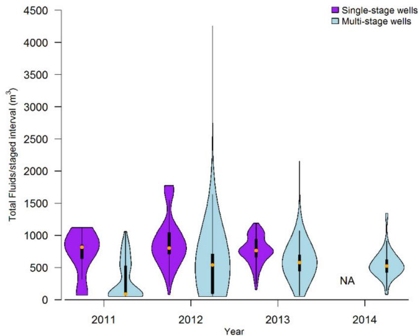
Figure 25: Normalized total volume of fluid used per staged interval in Weld County and their rotated kernel densities on each side (NA: not enough data) (COGCC dataset)
