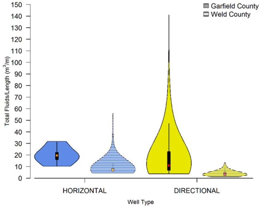
Figure 26: Normalized total volume of fluid used per length of well and their rotated kernel densities on each side (COGCC dataset)
