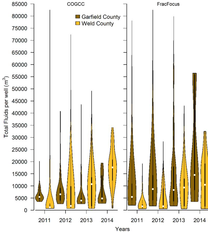
Figure 27: Total volume of fluid consumed for hydraulic fracturing on a per well basis and their rotated kernel densities on each side (COGCC and FracFocus dataset)
