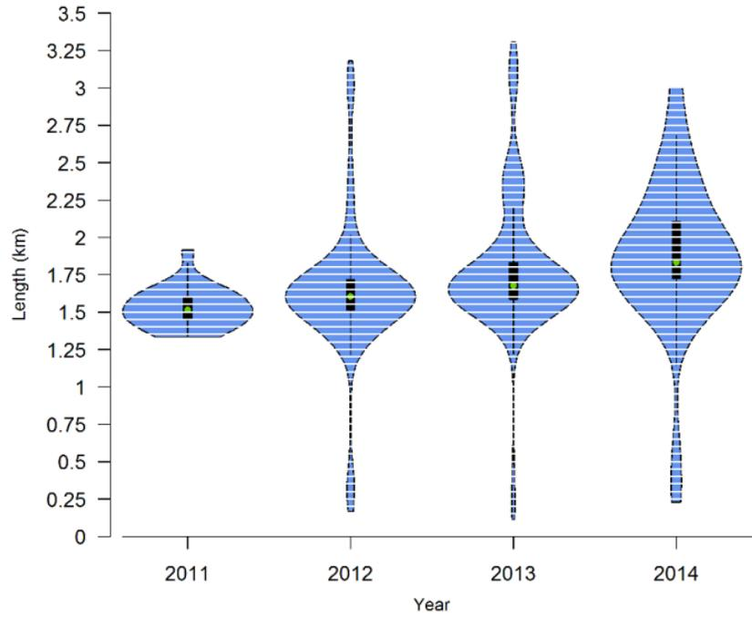
Figure 23: Length of horizontal wells in Weld County and their rotated kernel densities on each side (COGCC dataset)
