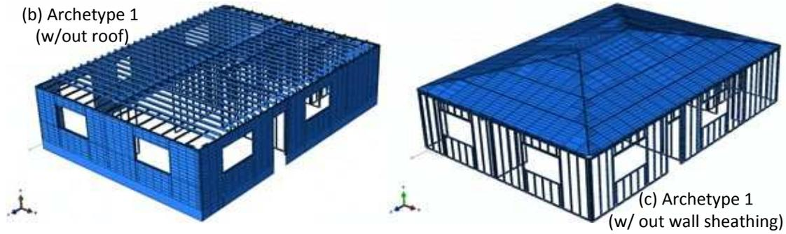
**FIGURE 3. 1 – Archetype 1 layout (a) complete, (b) w/out roof, (c) w/out wall sheathing**
