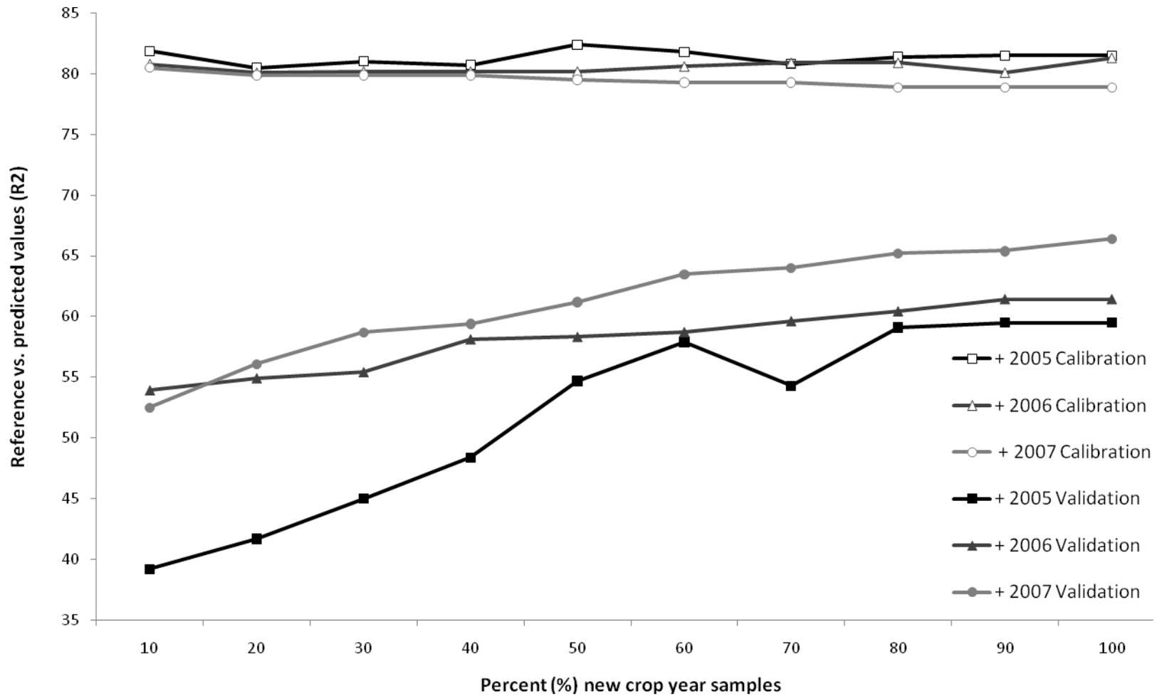
Figure 1.7. Effect of adding percentages (%) of new crop year samples on prediction of kernel hardness index. Validation was done on remaining samples of the new crop year.
