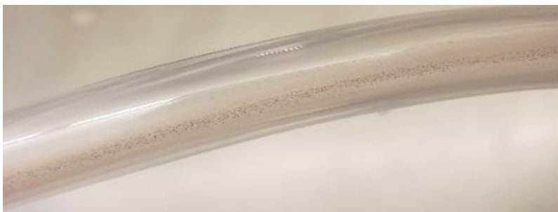
Figure 2.5. Image of settled CuBTri on the tubing that was coated with the initial coating procedure using 0.1% w/v CuBTri.
