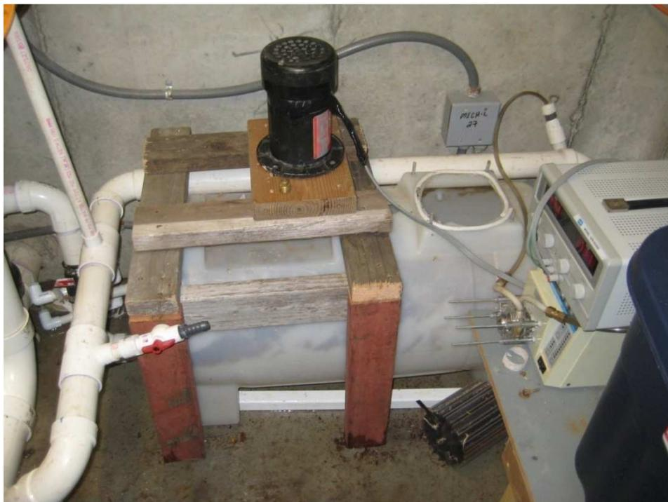
**Figure 9.9: Perforated PVC housing around compositing tank influent draw tubing**
