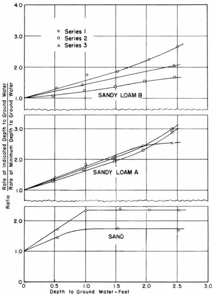
FIGURE 38.—Effect of depth to ground water on seepage rate in sand, sandy loam A, and sandy loam B.
