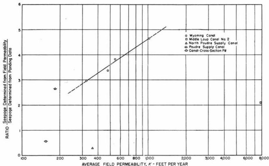
FIGURE 23.—Relationship of seepage rates derived from field permeameter data and those derived from ponding data by use of the equation  $R=3.3 \log_{10} K-5.3$ , for three series of tests made in the present study and two made by the Bureau of Reclamation.
