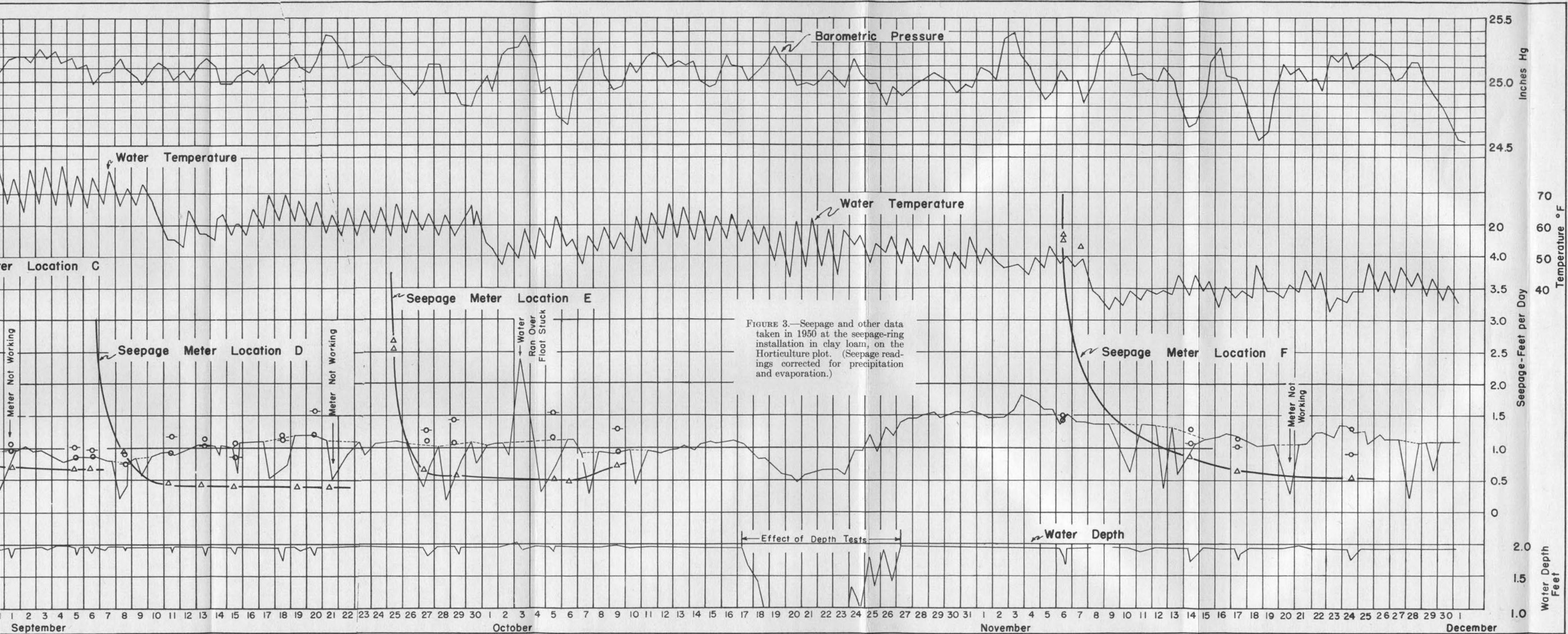
FIGURE 3.—Seepage and other data taken in 1950 at the seepage-ring installation in clay loam, on the Horticulture plot. (Seepage readings corrected for precipitation and evaporation.)
