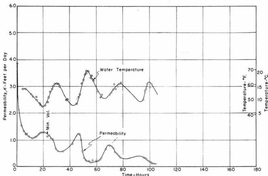
FIGURE 31.—Effect of temperature on soil permeability in well-permeameter tests, proposed North Poudre Supply Canal. (Permeability corrected for viscosity to 60° F.)
