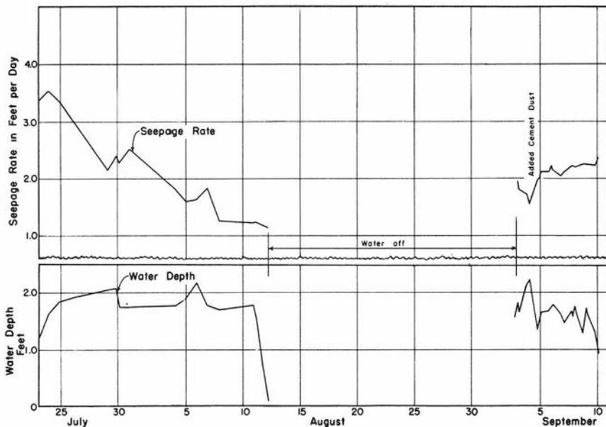
FIGURE 20.—Results of ponding tests in canal-cross-section pit, 1952.
