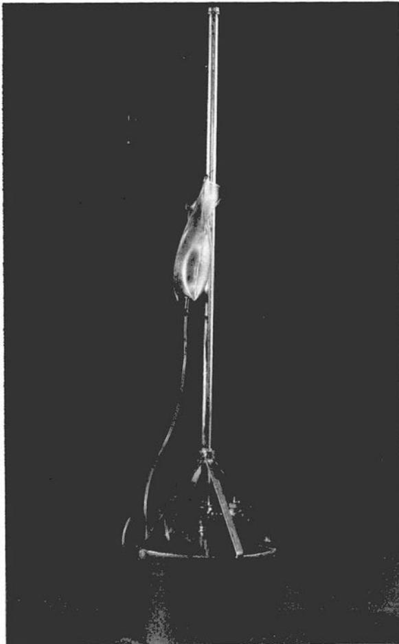
FIGURE 11.—Bureau of Reclamation seepage meter, with metal bell and plastic bag.
