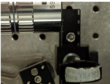
Figure C10: Picture showing the location of the silicon lens after the sample in the collinear geometry.
