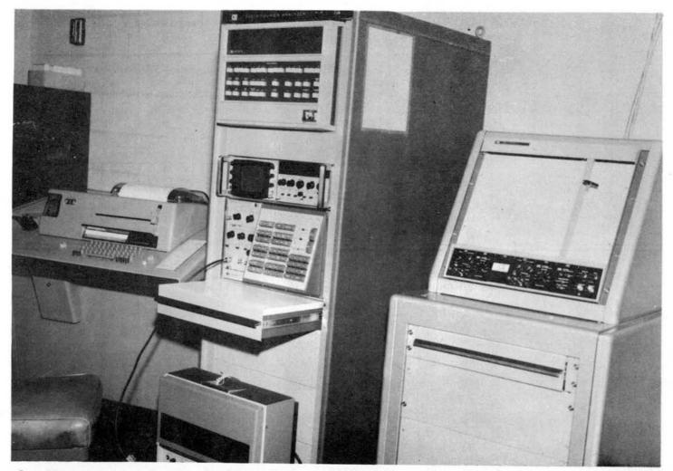
Figure 4. Photograph of Fourier Analyzer System utilized to analyze data. (US Army photograph)
