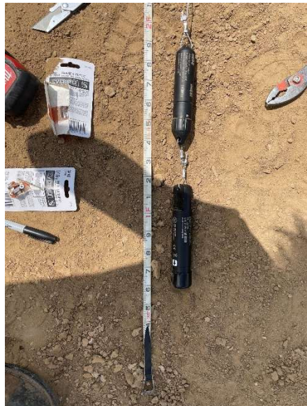
Figure A.3 Example of EC and 30' WL sensor chained together.
