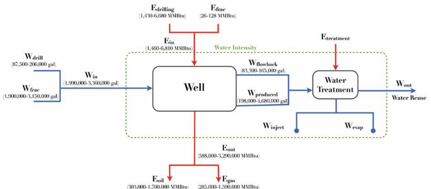
Figure 1. Material balance used to define the water intensity assessment of Noble Energy oil and gas wells in the Wattenberg field
