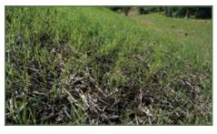
WoodStraw<sup>®</sup> is an erosion-control material made up of interlocking wood strands. Photo: Trent Jones
