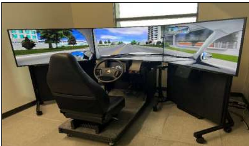
Figure 5. NADS miniSim driving simulator located in CSU Human Systems Lab
