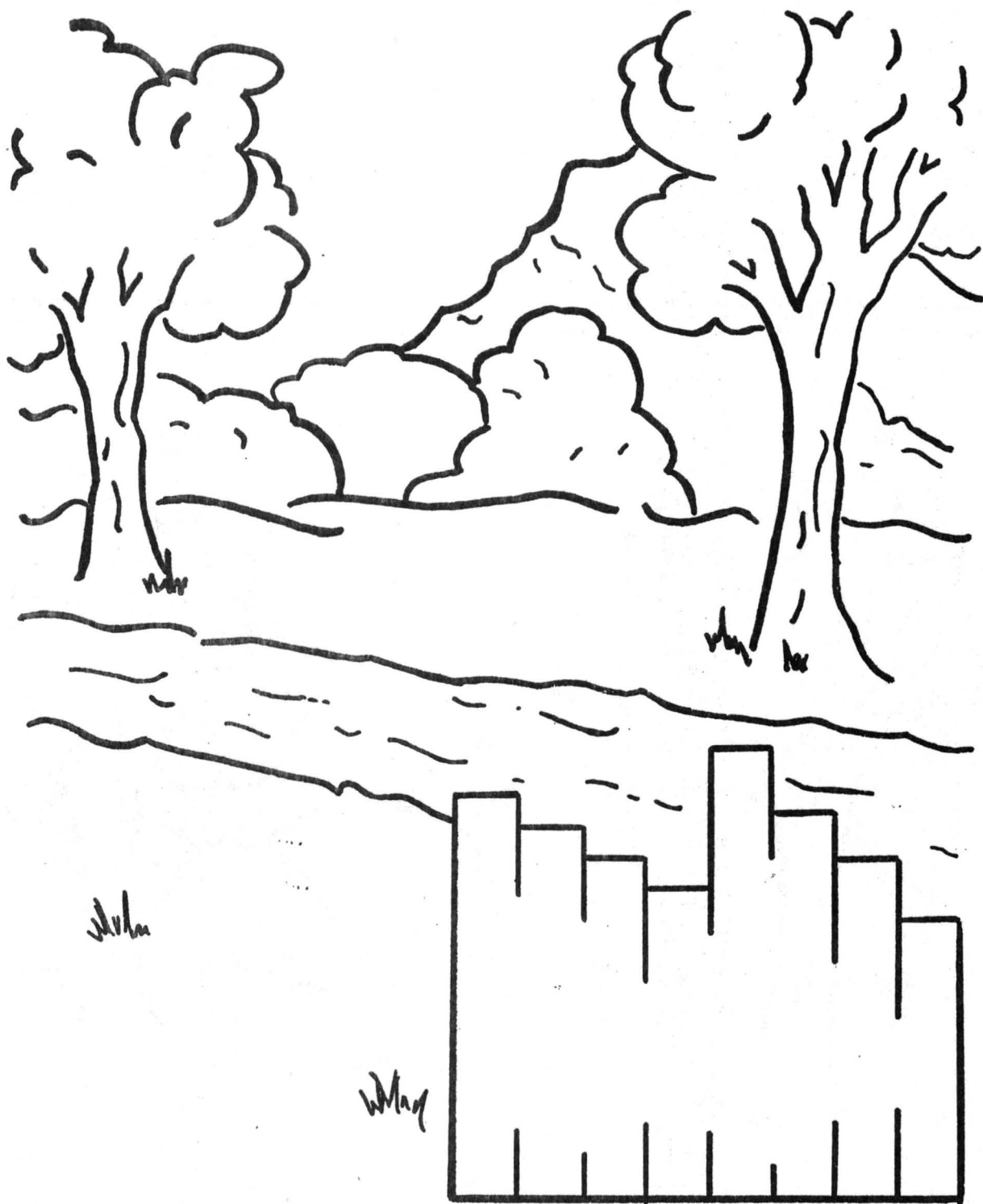
Figure 8. A sturdy entrance sign could be made of logs bolted together and sunk in the ground. Lettering could be painted or plastic or metal letters nailed on the sign.
