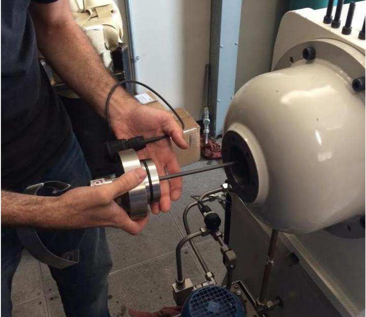
**Figure 8.8 Removing RCM Linear Transducer.**
