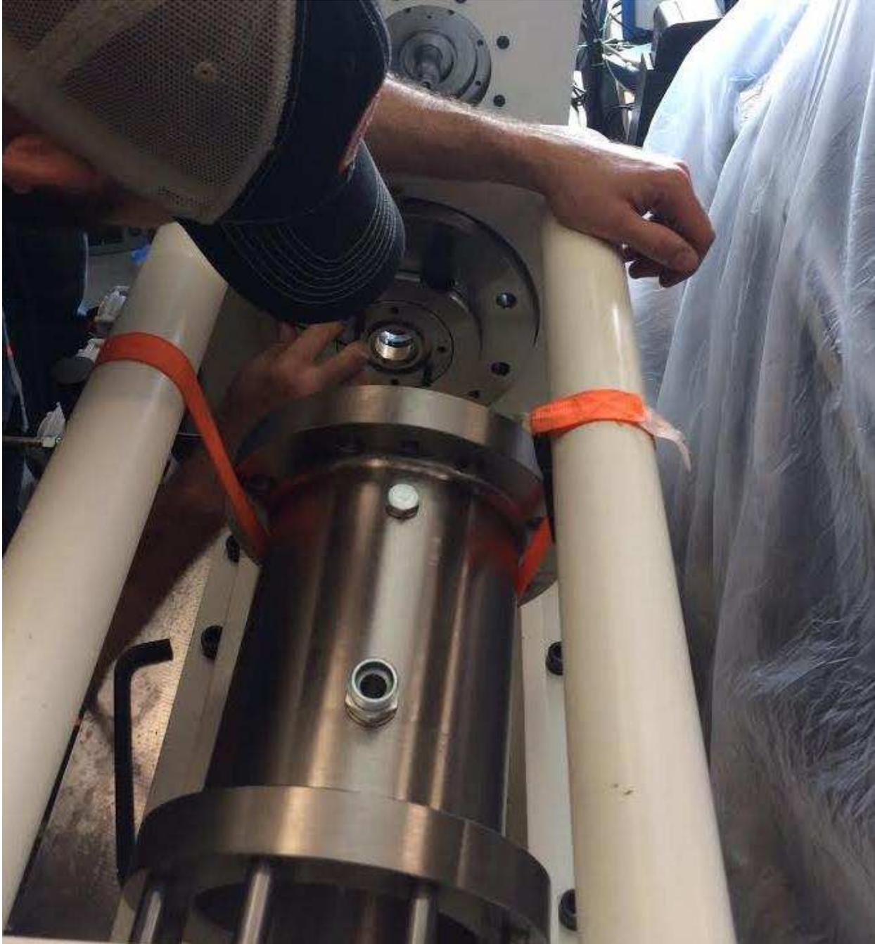
**Figure 8.14 External Oil Chamber supported by Ratchet Strap.**
