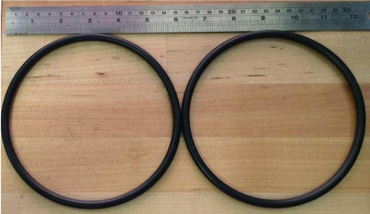
**Figure 9.10 Rear Hydraulic Oil Chamber Seals.**
