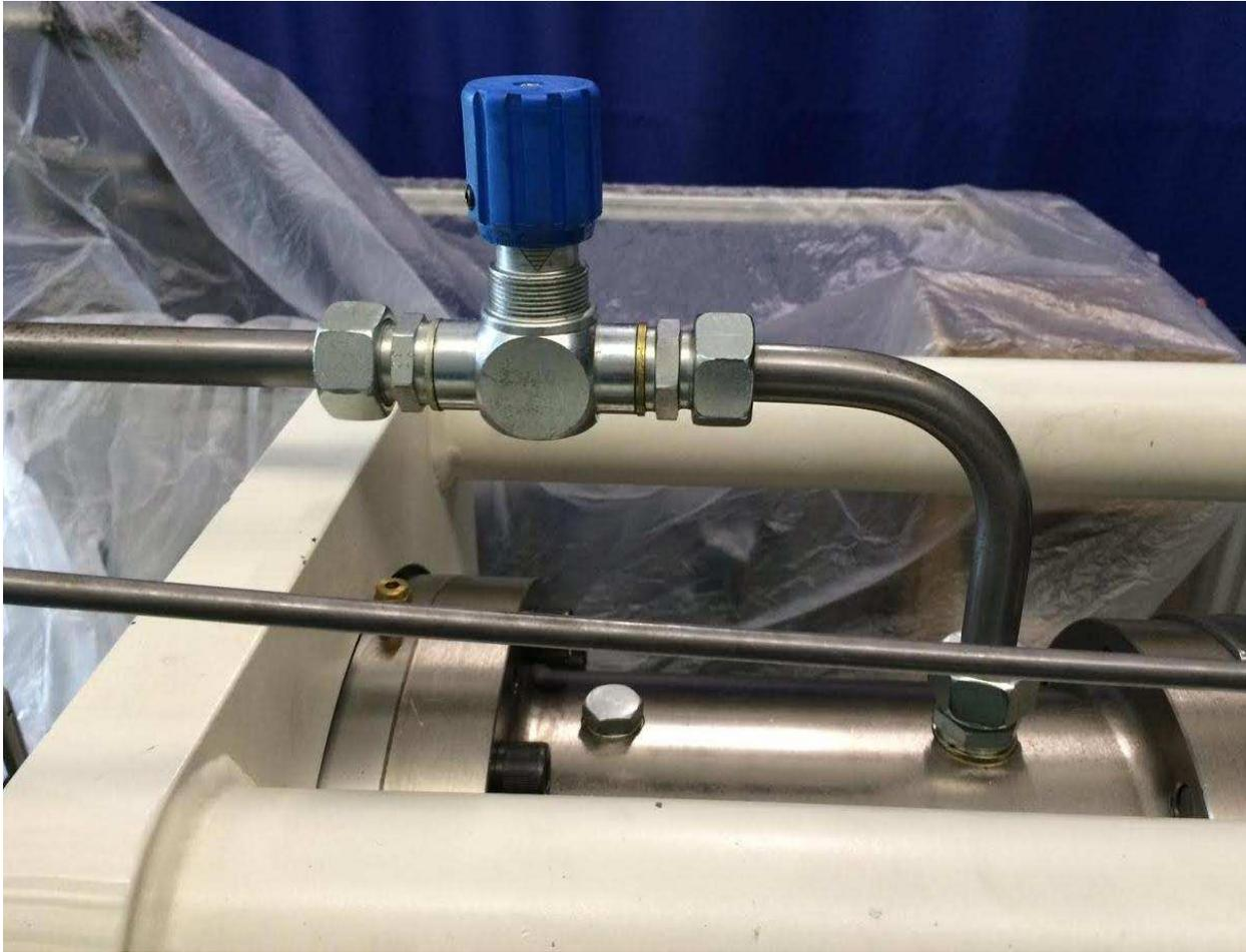
**Figure 8.13 Rapid Compression Machine Main Hydraulic Line.**
