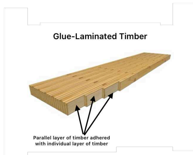
Figure 16: Glue Laminated Timber Manufacturing Detail
