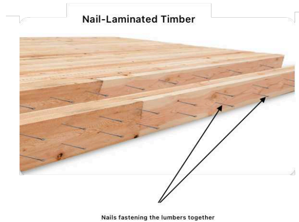
Figure 17: Nail Laminated Timber Manufacturing Detail.
