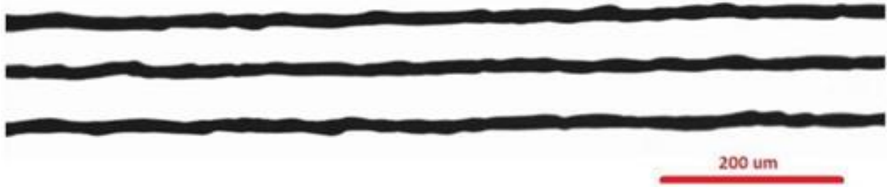
Figure 4.7. Batch of fibers with jogged morphology. Mean Batch Diameter: 13.52 \pm 0.95 \mu\text{m}
