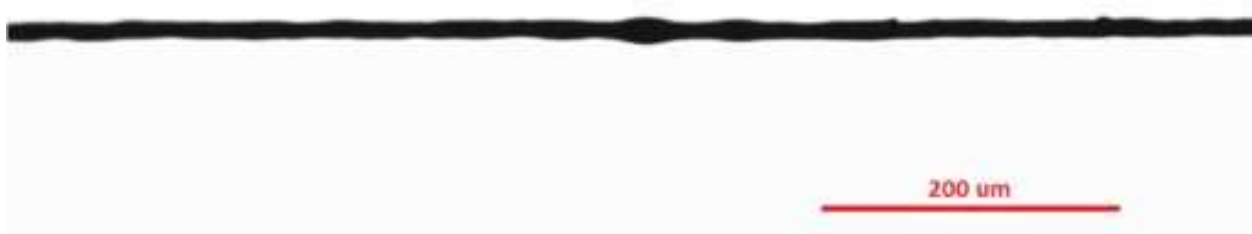
Figure 4.2. Non-uniform morphology. Diameter: 12.93 \pm 0.76 \mu\text{m} UTS: 1.57 GPa
