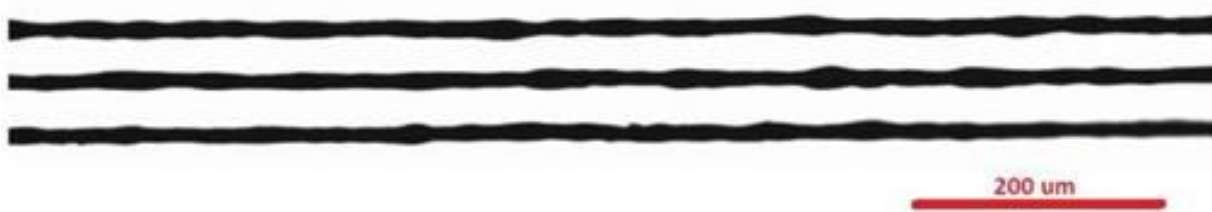
Figure 4.9. Batch of fibers with fluctuating morphology. Mean Batch Diameter: 11.93 \pm 0.58 \mu\text{m} Mean Batch UTS: 0.64 \pm 0.44 GPa
