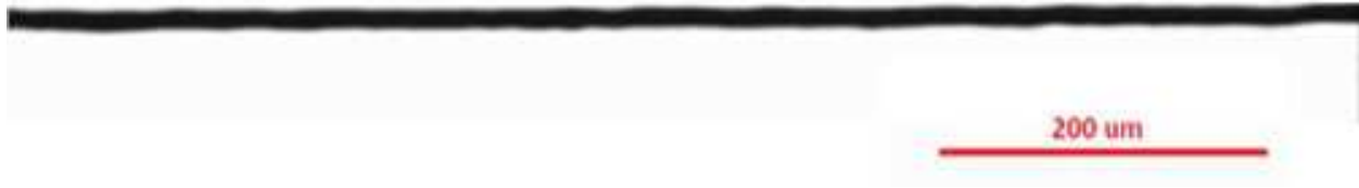
Figure 4.1. Straight morphology. Diameter: 12.37 \pm 0.51 \mu\text{m} UTS: 3.36 Gpa
