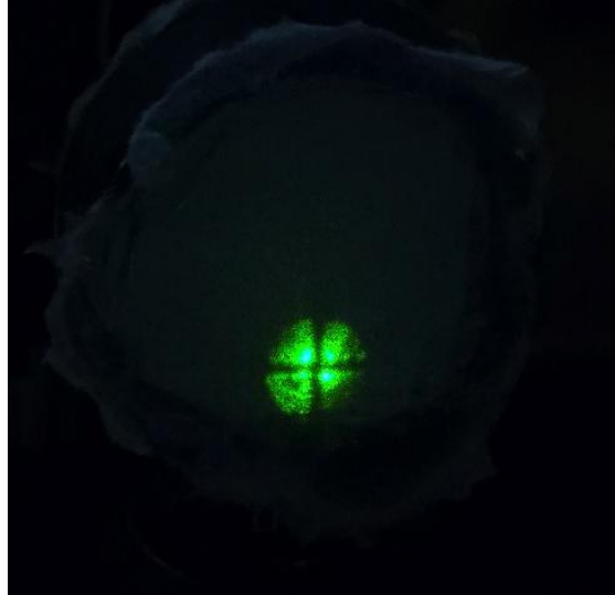
Figure 7: A well aligned cavity using proprietary targets
