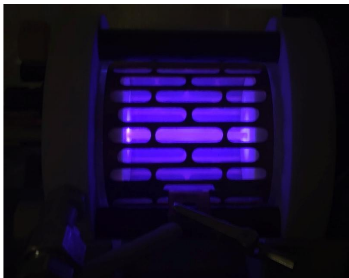
Figure 12: DBD regime at 22% NH 3 /78% N 2 45.1 SLPM 100 kHz, 100 pulses 900 VDC, 0.49 SEI
