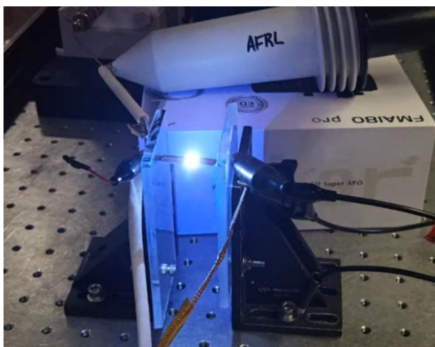
Figure 8: Plasma discharge at atmospheric conditions to validate function of HV pulser system This initial test validated that the pulser system had arrived in functioning condition from
