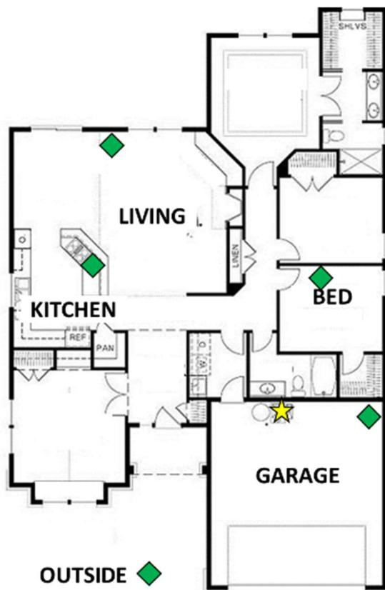
Figure 1: Example layout of home locations of commercial-grade indoor air quality sensors (green diamonds) and energy monitor (yellow star) indicated.
