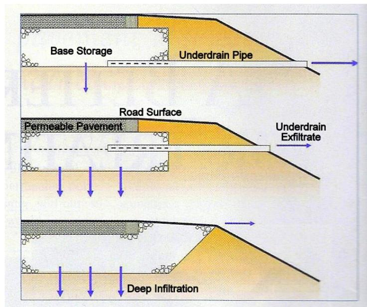
**Figure 2.5-4 Permeable Pavement Underdrain Configurations**
