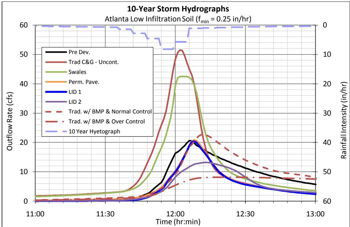
Figure 13.2-3 10-Year Storm Hydrographs – Atlanta Low Infiltration Soil
