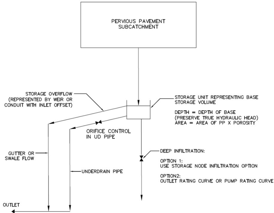
**Figure 4.3-1 SWMM Representation of Permeable Pavement with Underdrain**
