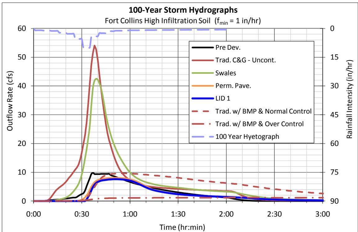
Figure 12.1-4 100-Year Storm Hydrographs – Fort Collins High Infiltration Soil
