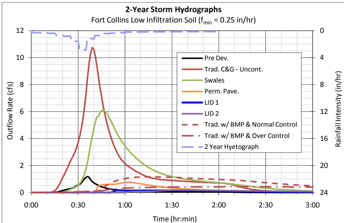
Figure 12.2-2 2-Year Storm Hydrographs – Fort Collins Low Infiltration Soil
