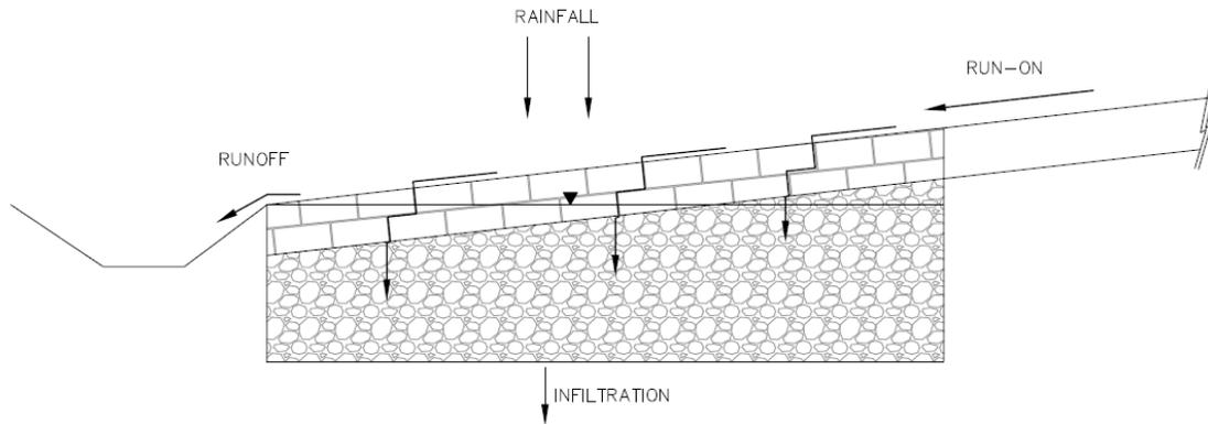
**Figure 4.2-3 Permeable Pavement - Runoff Condition**
