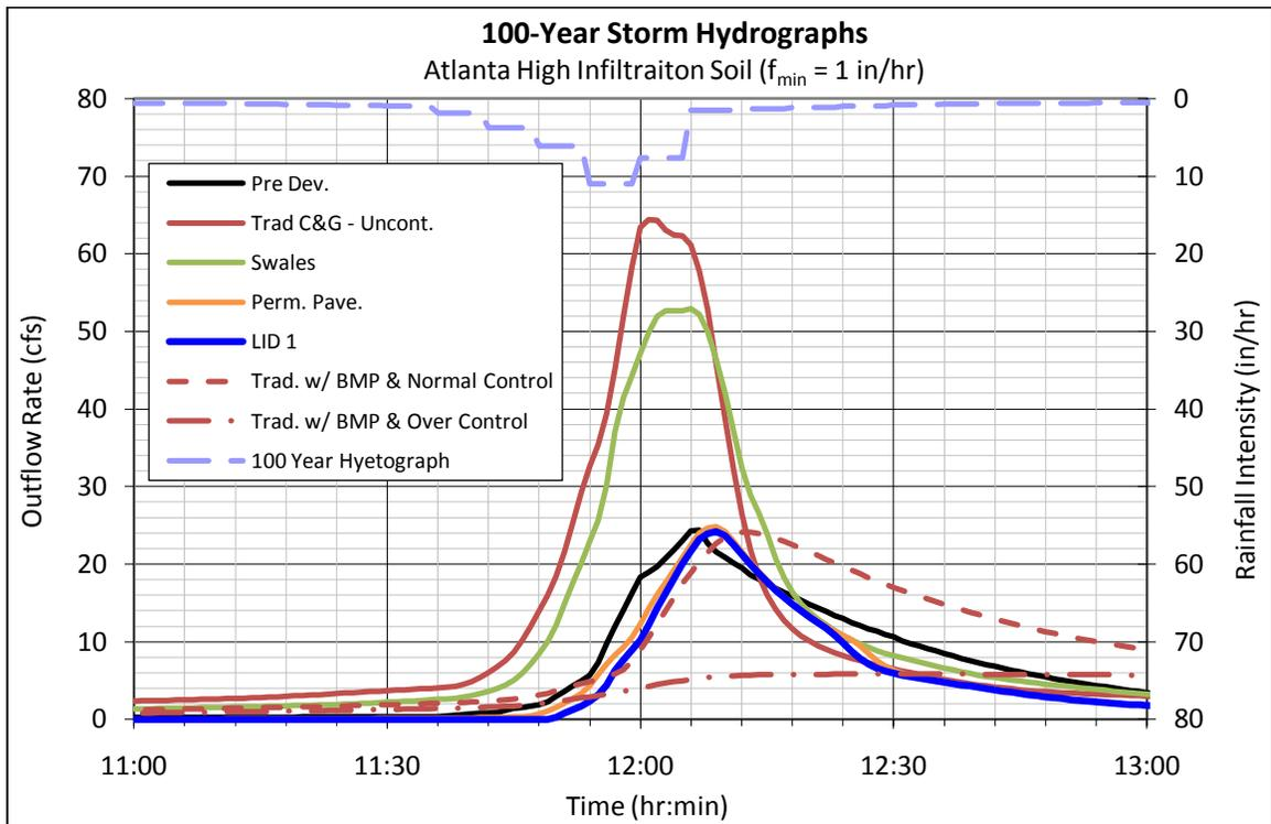
Figure 13.1-4 100-Year Storm Hydrographs – Atlanta High Infiltration Soil
