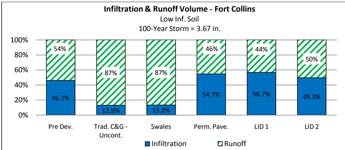
**Figure 12.3-2 Water Balance Graphs – Fort Collins Low Infiltration Soil**
