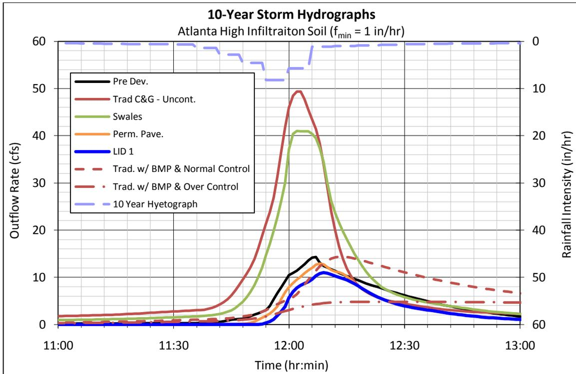
Figure 13.1-3 10-Year Storm Hydrographs – Atlanta High Infiltration Soil
