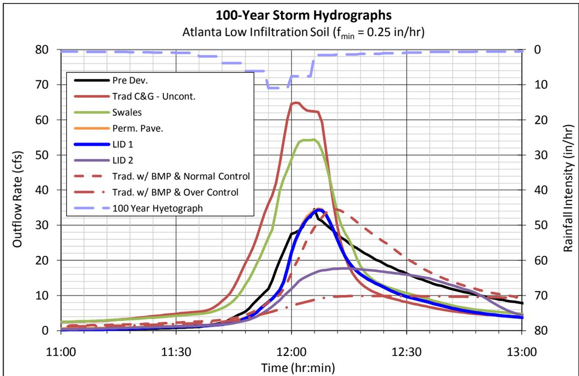
Figure 13.2-4 100-Year Storm Hydrographs – Atlanta Low Infiltration Soil
