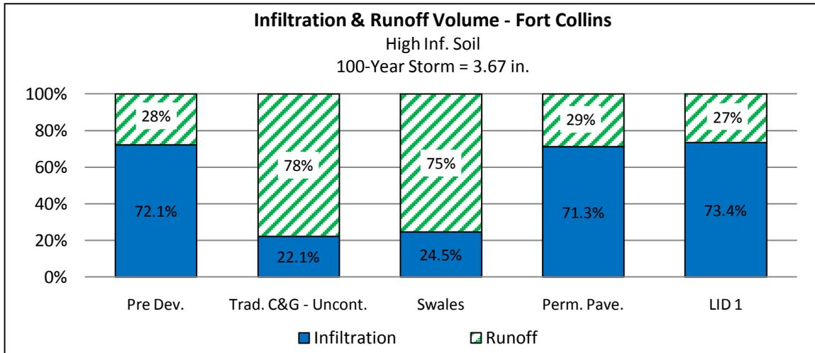
**Figure 12.3-1 Water Balance Graphs – Fort Collins High Infiltration Soil**
