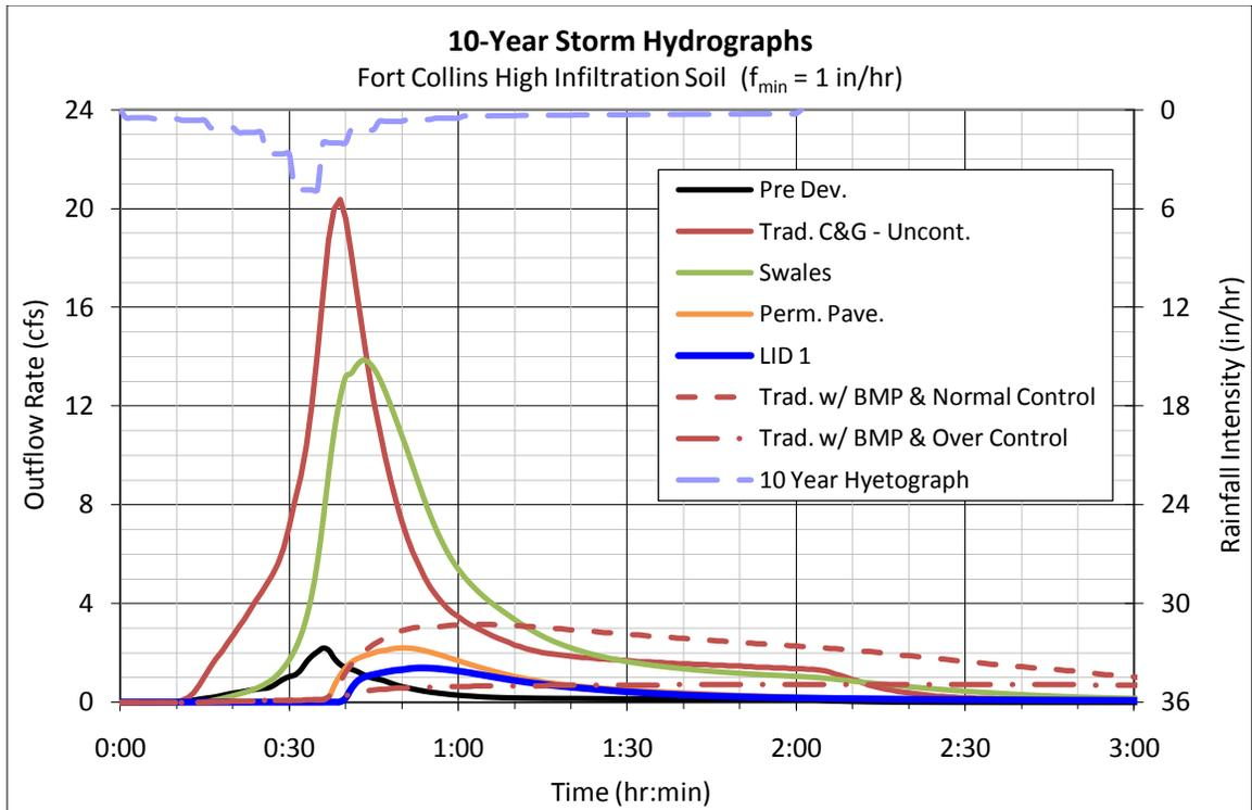
Figure 12.1-3 10-Year Storm Hydrographs – Fort Collins High Infiltration Soil
