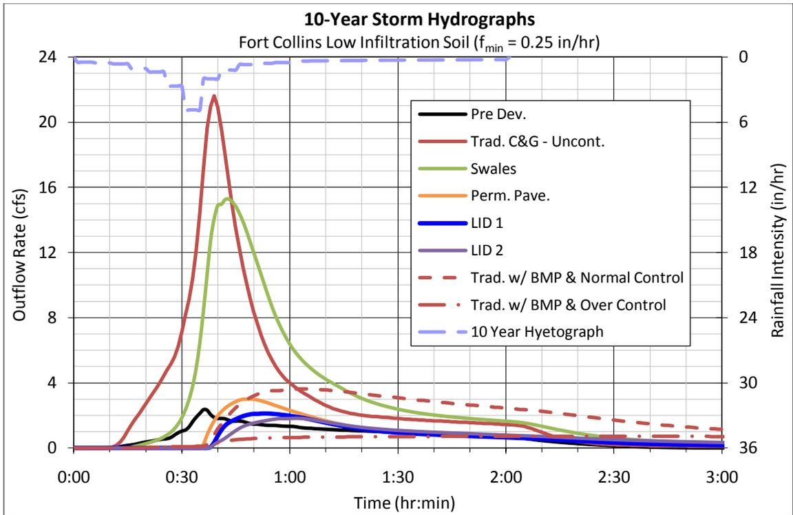
Figure 12.2-3 10-Year Storm Hydrographs – Fort Collins Low Infiltration Soil
