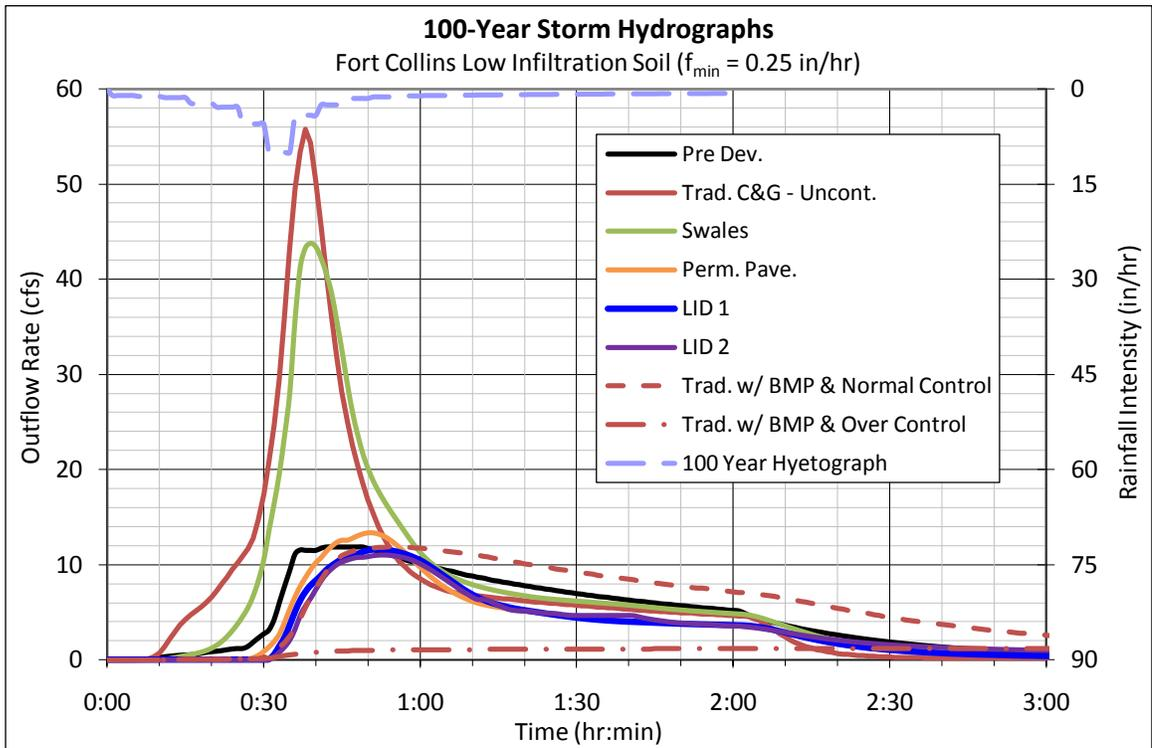
Figure 12.2-4 100-Year Storm Hydrographs – Fort Collins Low Infiltration Soil
