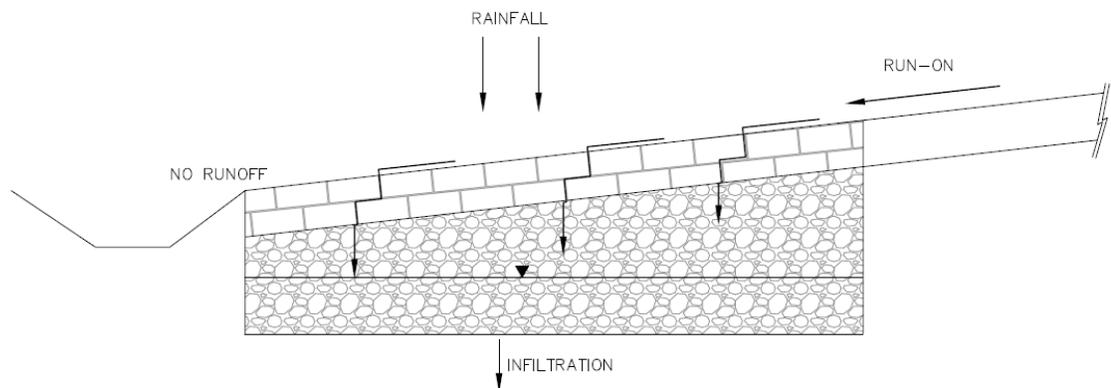
**Figure 4.2-2 Permeable Pavement - No Runoff Condition**
