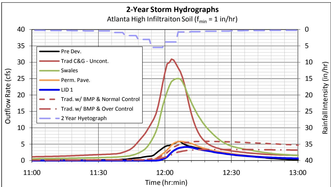
**Figure 13.1-2 2-Year Storm Hydrographs – Atlanta High Infiltration Soil**
