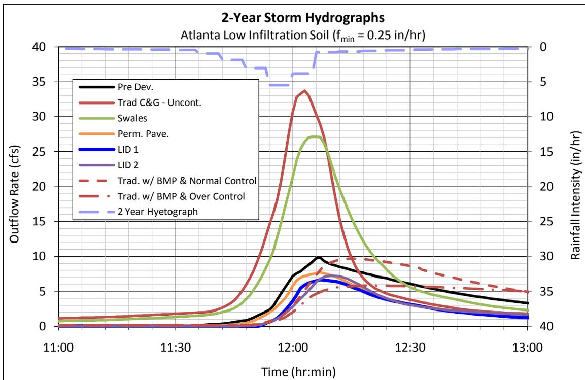
Figure 13.2-2 2-Year Storm Hydrographs – Atlanta Low Infiltration Soil
