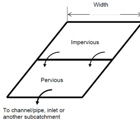
**Figure 4.2-1 Pervious Subcatchment Routing**
