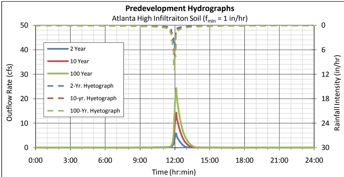
**Figure 13.1-1 Predevelopment Hydrographs – Atlanta High Infiltration Soil**
