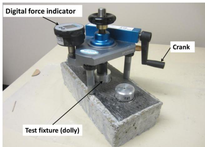
Figure 3.8. Pull-off testing setup
