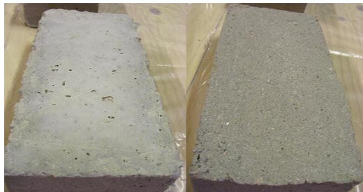
Figure 3.4. Concrete surface before (left) and after (right) sandblasting
