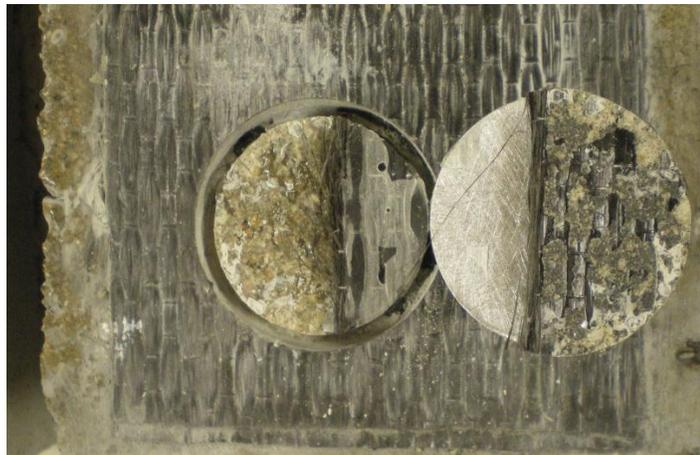
Figure 3.22. Combined Mode A and Mode F failure
