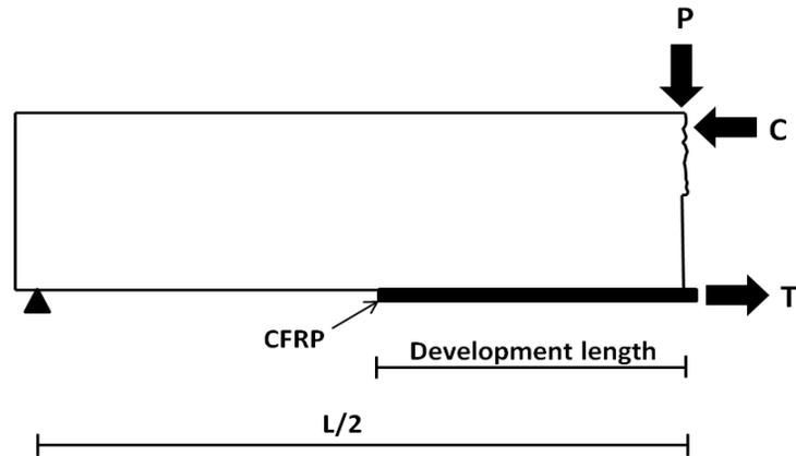
Figure 2.6. Development length and forces under three-point bending. This figure shows half of the beam.  $P$  is the load applied at mid-span,  $T$  is the tension force generated at the bottom of the beam, and  $C$  is the compression force at the top of the beam
