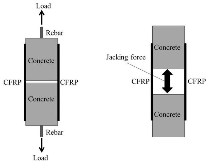
Figure 2.2. Types of Double-Face Shear Tests
