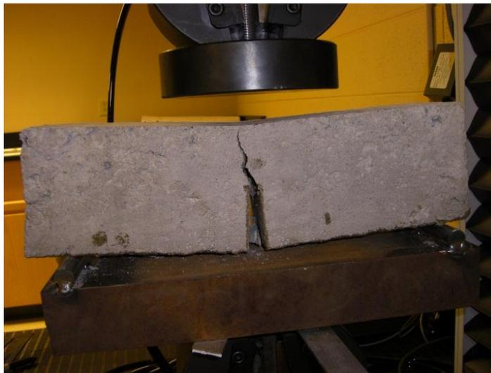
Figure 3.16. Beam following crack failure
