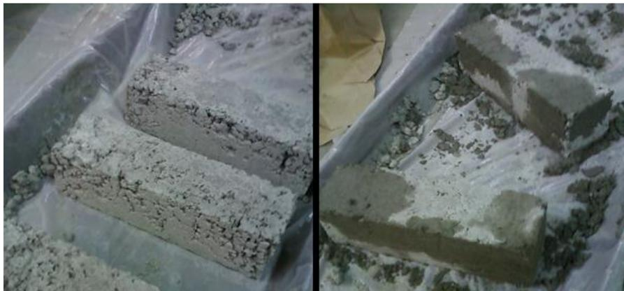
Figure 3.3. Concrete beams before (left) and shortly after (right) patching
