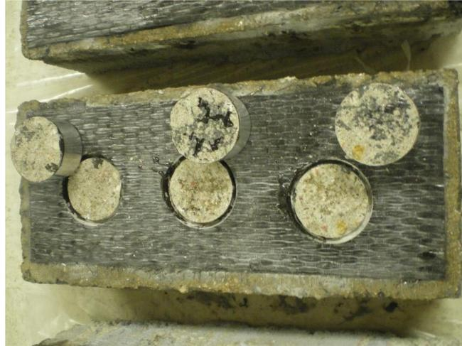
Figure 3.19. Mode F failures (ASTM D7522) during Stage 1 testing
