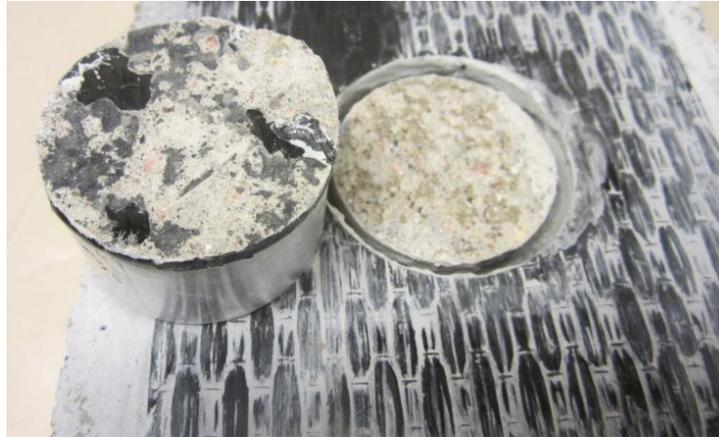
Figure 3.24. Representative Mode F failure for Stage 2
