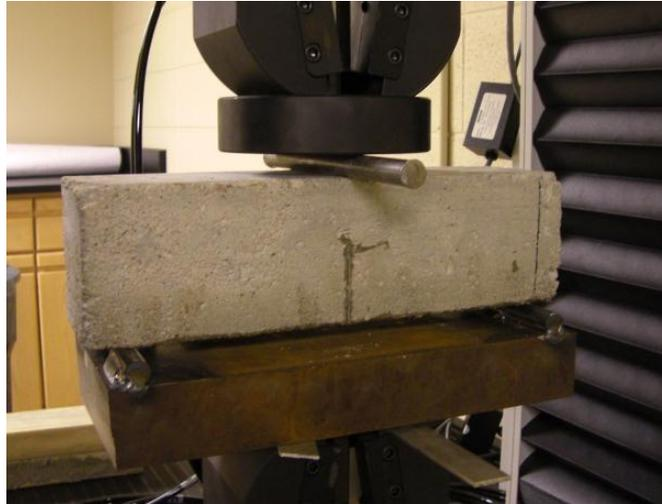
Figure 3.10. Beam fixture and specimen
