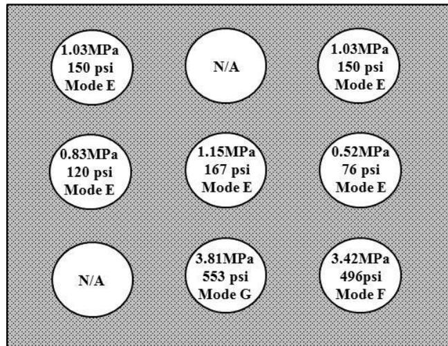
Figure 4.5. Pull-off test results, including strengths and failure modes for north end of west arch, labeled as 1NW. Dollies spaced approximately 6 in (15 cm) center-to-center from each other.
