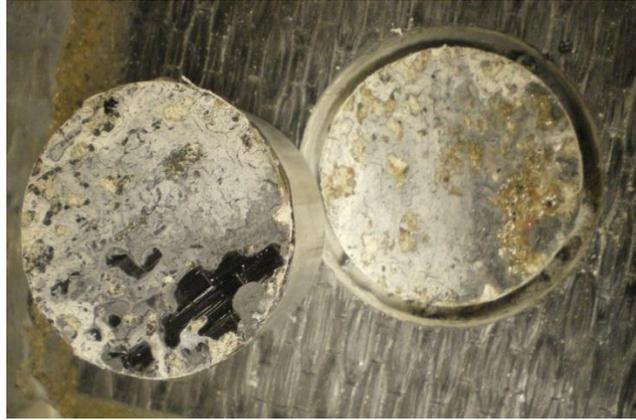
Figure 3.21. Presence of moisture at CFRP-concrete interface
