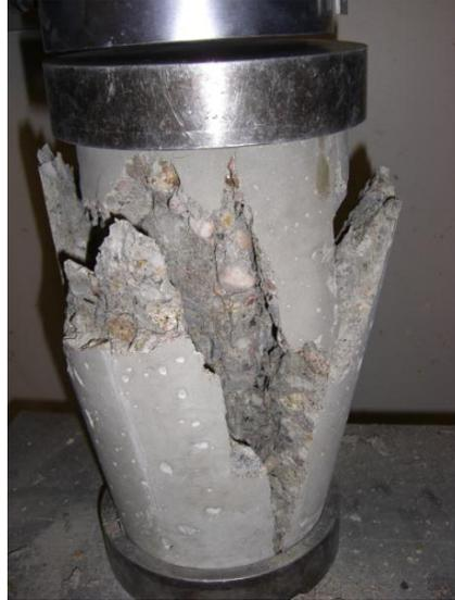
Figure 3.11. Characteristic failure for compression tests
