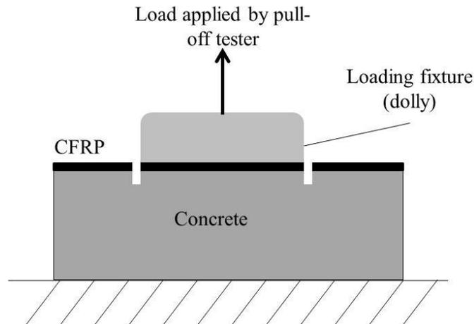
Figure 2.3. Pull-off test representation
