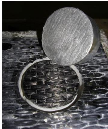
Figure 3.12. Pull-off Mode A failure
