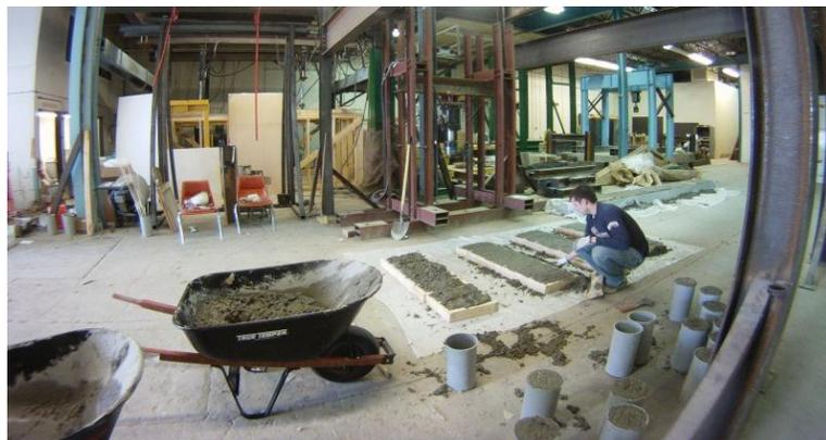
Figure 3.2. Casting of concrete specimens
