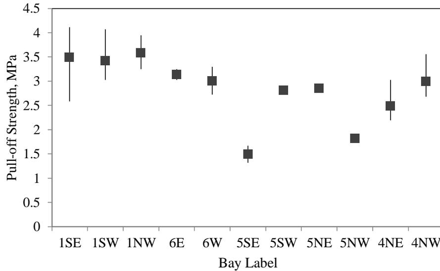
Figure 4.3. Castlewood Canyon Bridge pull-off strength results (CTC-Geotek, 2003)
