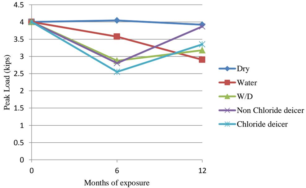
Figure 3.30. Average beam results for the 6-month and 12-month exposure
