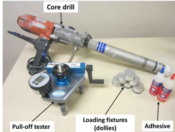
Figure 2.4. Instruments needed to conduct pull-off tests
