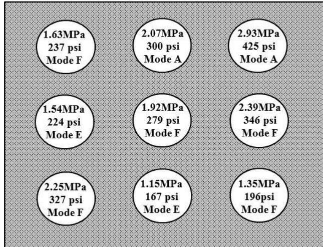
Figure 4.4. Pull-off test results, including strengths and failure modes for north end of east arch, labeled as 1NE. Dollies spaced approximately 6 in (15 cm) center-to-center from each other.
