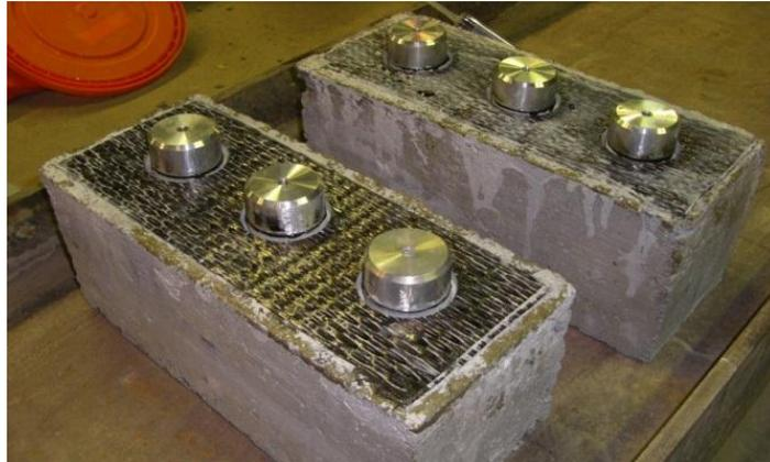
Figure 3.7. Concrete specimens following adhesion of dollies
