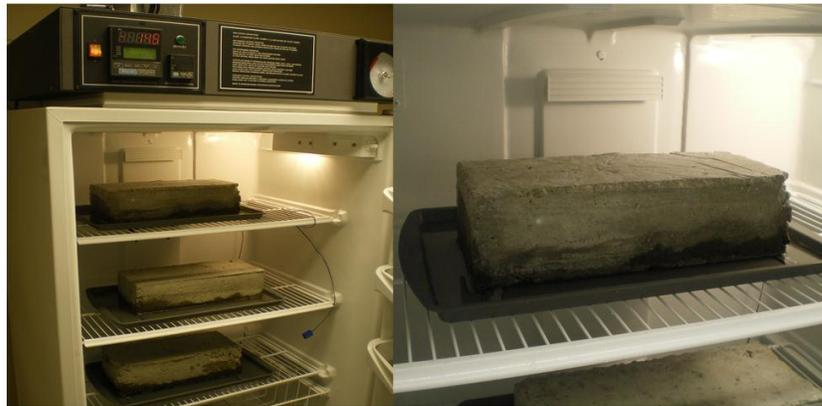
Figure 3.1. FRP Reinforced Concrete specimens undergoing free-thaw exposure
