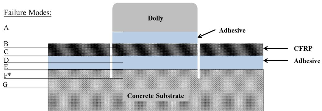
Figure 2.5. Pull-off test failure modes. Mode F failure represents a combination of Mode E and Mode G failures
