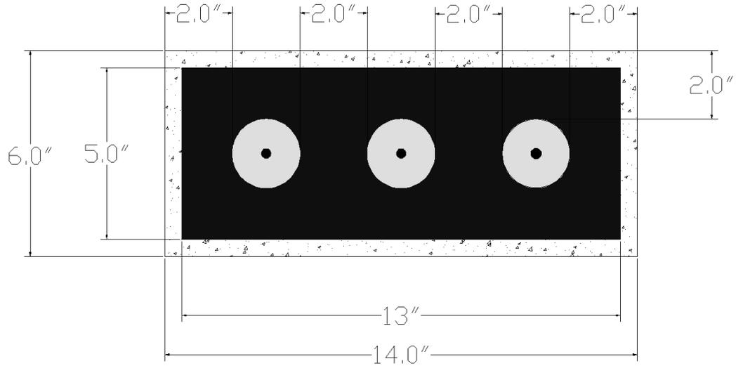
Figure 3.6. Specimen dimensions and dolly spacing
