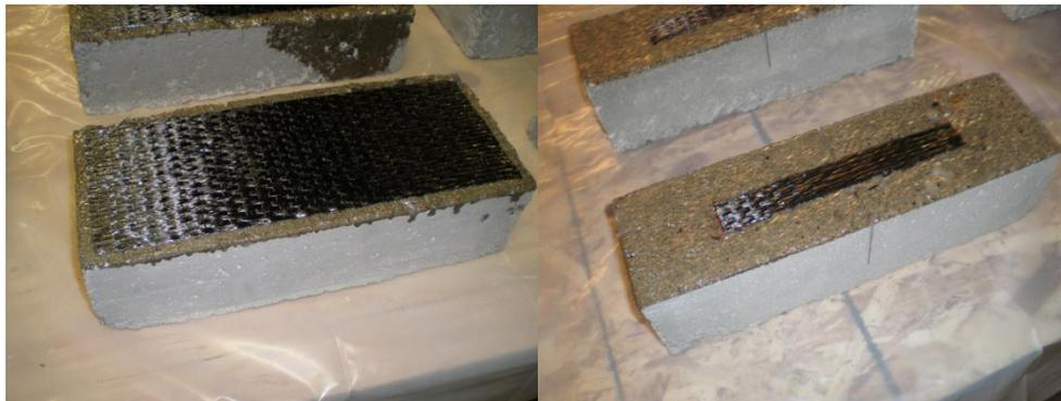
Figure 3.5. Concrete specimens reinforced with CFRP for pull-off (left) and flexural (right) tests
