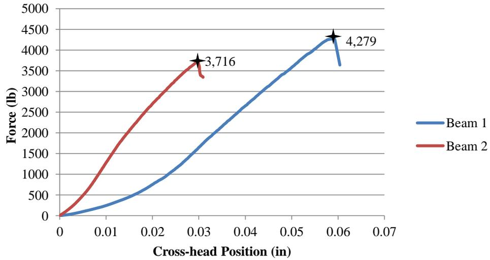
Figure 3. 18. Force vs. Displacement Graphs for Stage 0 Beams
