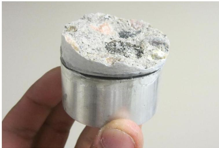
Figure 3.25. Mode G Failure in Dolly #20
