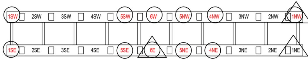
Figure 4.2. Pull-off test locations from 2003 study (circles) and 2011 study (triangles) (Allen, 2011)
