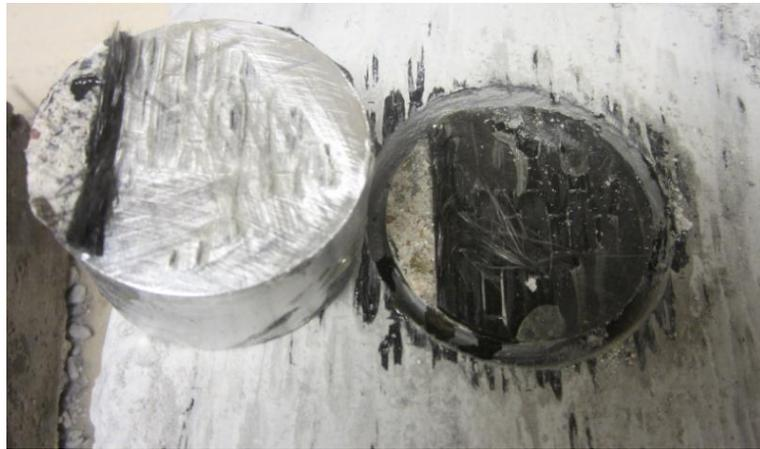
Figure 3.27. Combined Mode A and Mode F failure in Dolly #42
