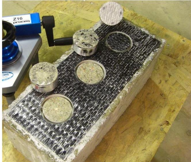
Figure 3.13. Pull-off Tests 1, 2, and 3 failure modes
