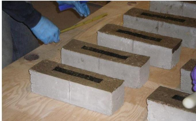
Figure 3.9. Concrete beams reinforced with CFRP
