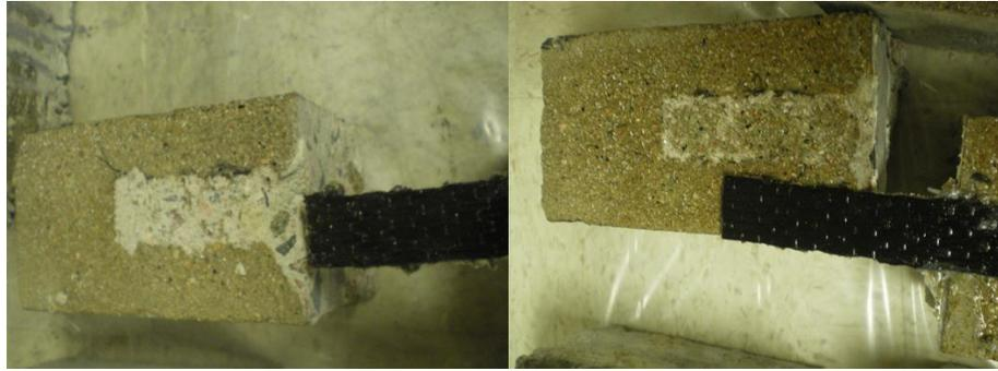
Figure 3.23. Beam #1 (left) vs. Beam #8 (right) failure
