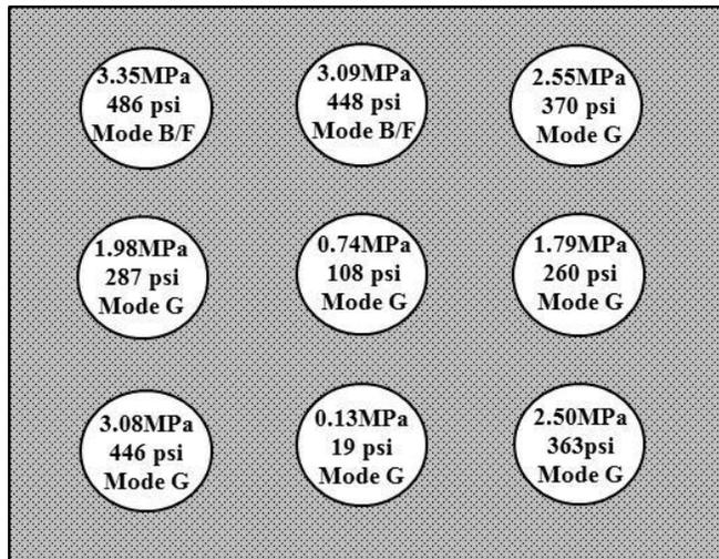
Figure 4.6. Pull-off test results, including strengths and failure modes for center of east arch, labeled as 6E. Dollies spaced approximately 10 in (25 cm) center-to-center from each other (Allen, 2011)
