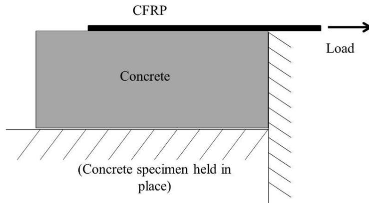
Figure 2.1 Direct Shear Test Representation.
