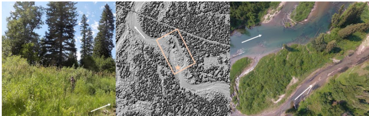
Figure 3.5. Accretion along the mainstem Swan River, downstream of Goat Creek confluence (Figure 3 for location within the catchment). This feature may be transitional between an island, as described for the tributaries, and an avulsion on the Swan River. The ground view is on the left, first-return hillshade from lidar is at the center, and the drone photograph is on the right. The pink box denotes the location of
