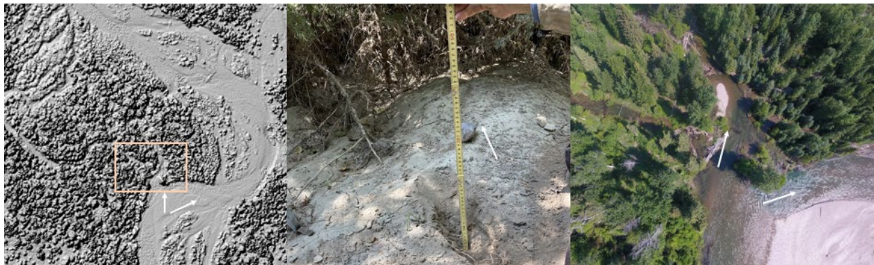
Figure 3.6. An avulsion on the Swan River downstream of Goat Creek (Figure 3 for location within catchment). The first return hillshade from lidar is on the left, ground view of floodplain vertical accretion during 2022 peak flows is at the center, and the
