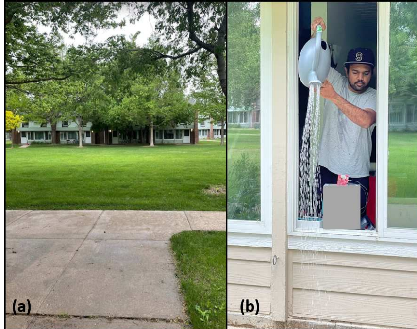
FIGURE 3.18. (a) scene of observation and (b) Snapshot of water being poured in front of the automobile radar evaluation board.
