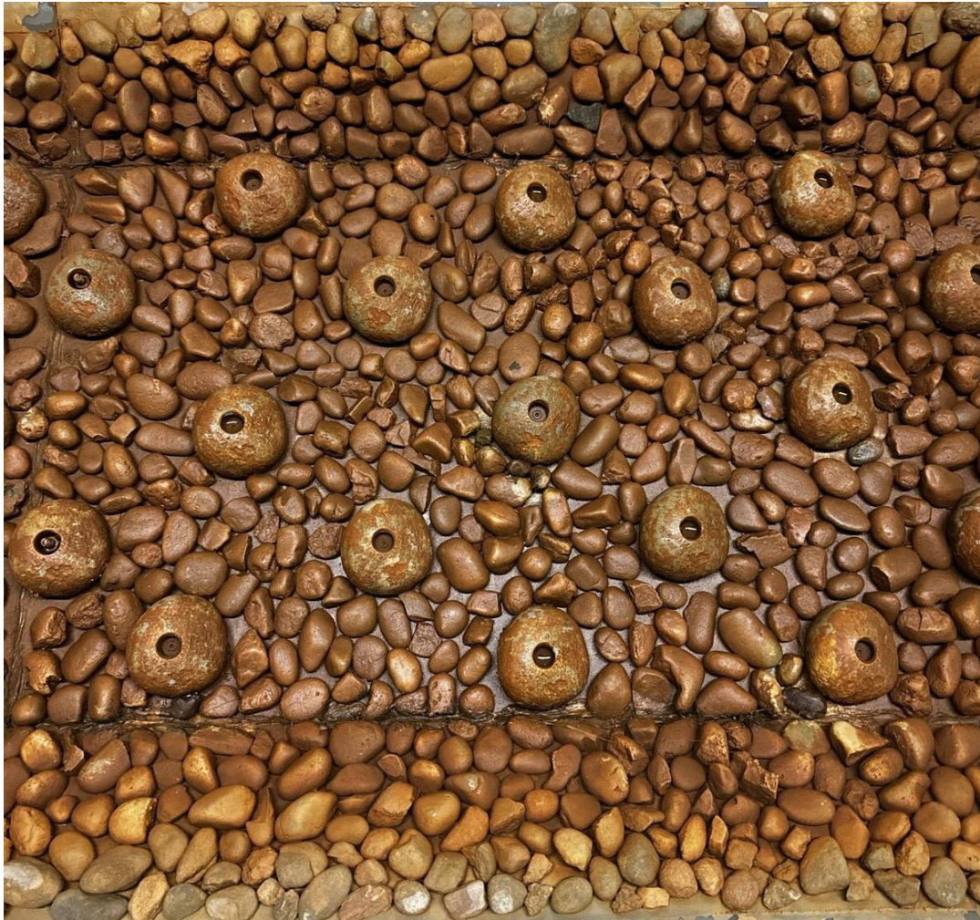
Figure 1. The 95-mm roughness elements were spaced approximately one diameter apart in a chevron pattern, with small cobble substrate adhered to the surface between the roughness elements and on the angled margins.
