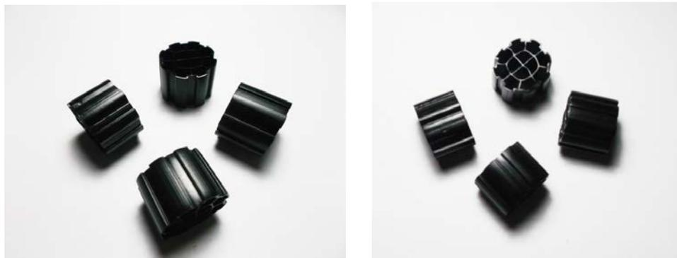
**Figure 5.2 Plastic media used in the fixed-film and hybrid reactors**
