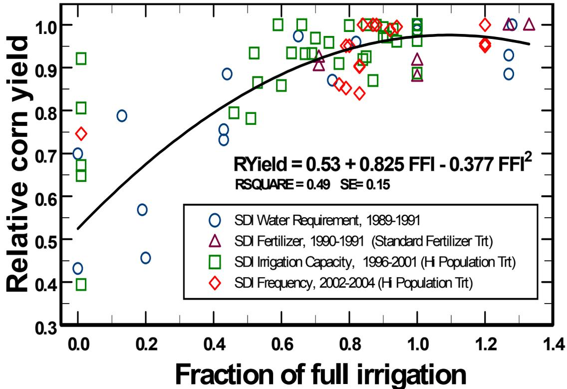
Figure 4. Relative corn grain yield for a given SDI research study and year as related to the fraction of full irrigation, Colby, Kansas.
