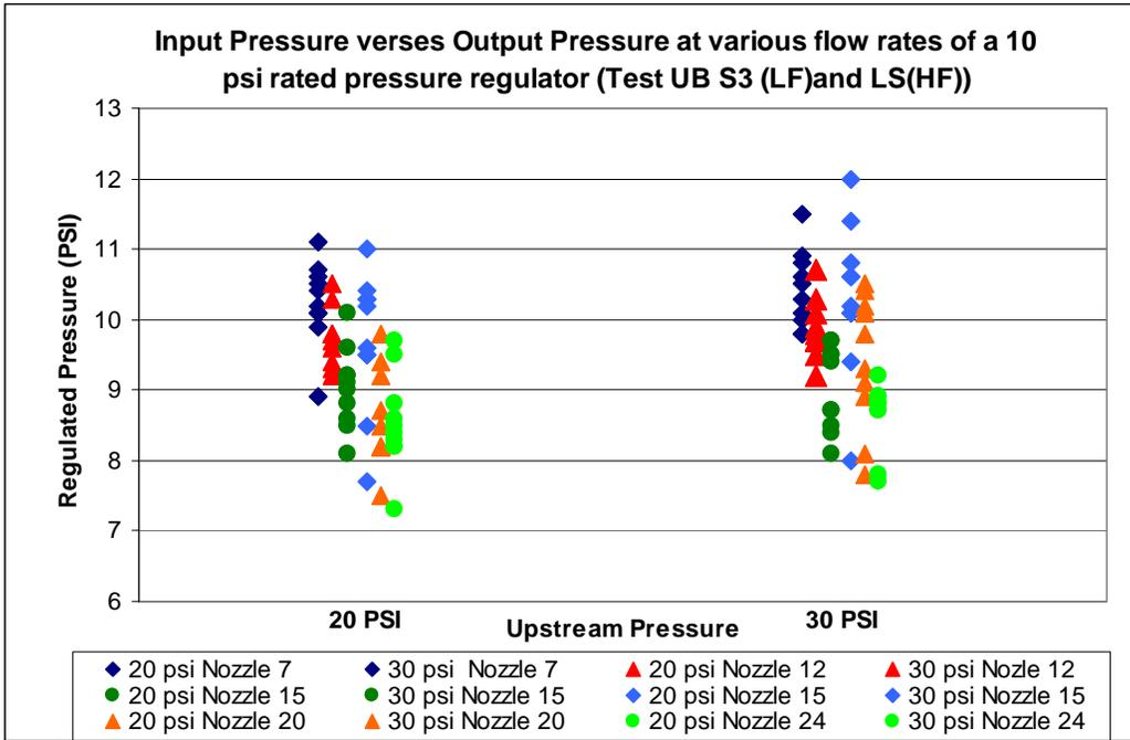
Figure 5. Input pressure verses output pressure at various flow rates for 10 psi pressure regulators for Tests UB S3 and LS.
