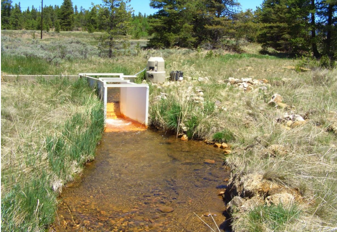
Figure C-33: View of CG-5 flume outlet and data recording equipment.
