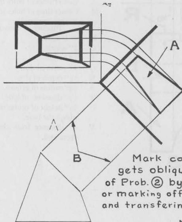
Mark correct if student gets oblique view from (B) of Prob. ② by using dividers or marking off on piece of paper and transferring to Prob. ③.
