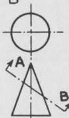
⑬ Cross out lines not drawn correctly in this projection the top view of which is correct
