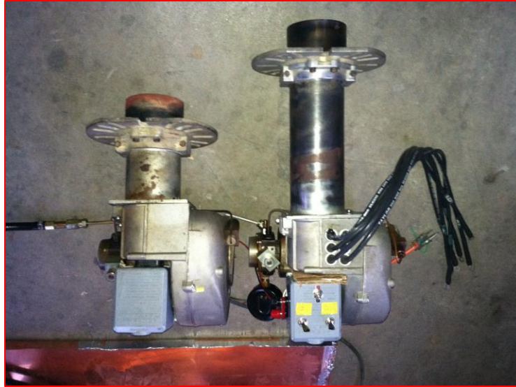
Figure 4-3: Stock burner (left) and modified burner (right).
