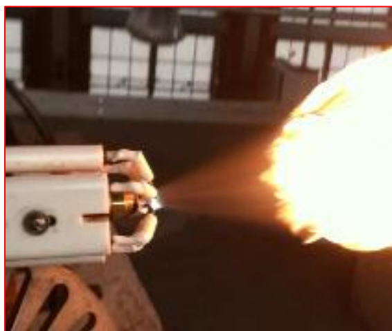
Figure 4-9: Combustion of fuel without the use of the turbulator or burner tube in the modified burner.
