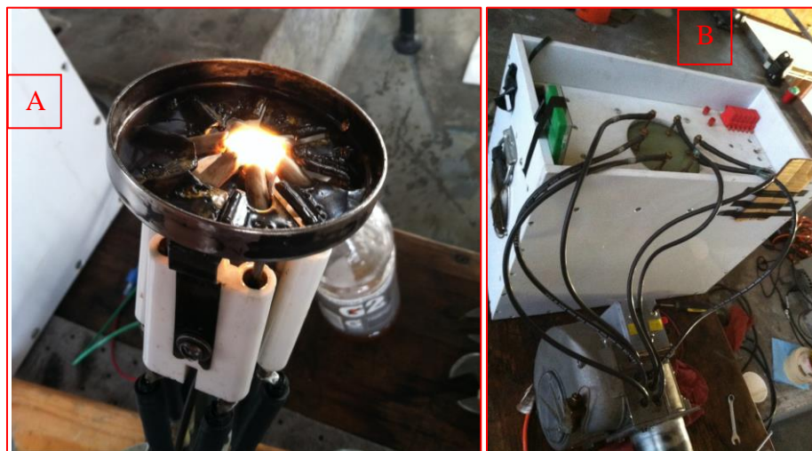
Figure 4-8: Modified burner - A) Electrodes and turbulator, B) Connection to plasma generator.
