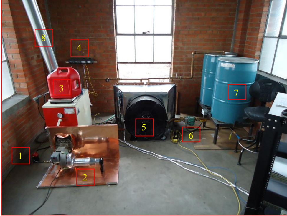
Figure 4-5: Burner Testing System: 1) Fuel Filter, 2) Air Sleeve and Anemometer, 3) Fuel Tank, 4) NI FieldPoint System, 5) Heat Exchanger/Fan, 6) Water Pump, 7) Water Tanks, 8) Exhaust Duct.
