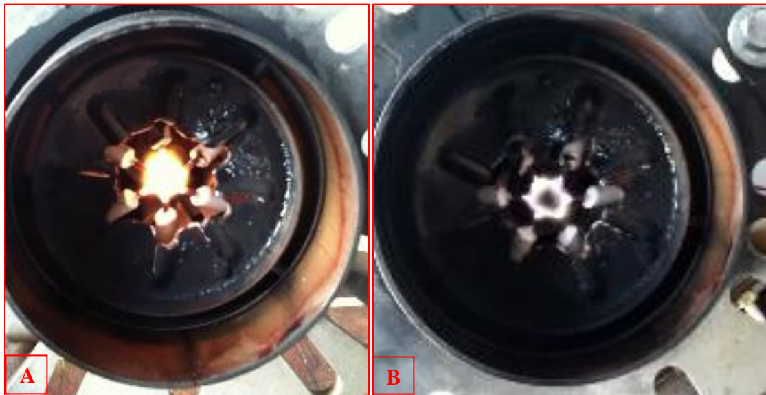
Figure 4-11: A) Plasma formation with no air flow, B) Plasma formation with air flow.
