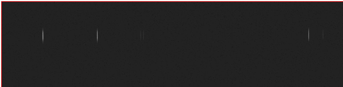
Figure 3-1: Spectrum collected with 150 g/mm grating, 10 micron slit width, and 5 ms exposure time.
