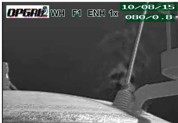
**Figure 3.8:** Still image taken from optical gas imaging (OGI) camera footage. In this case the emission rate exceeded the measurable leak rate, and was not capturing the entire emission plume.
