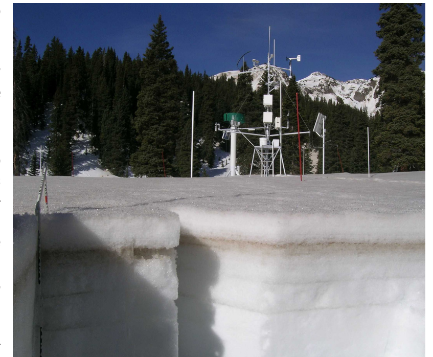
An excavated snow pit near a weather station features individual dust events layered throughout; April 30, 2013 at Swamp Angel in the Senator Beck Basin.
