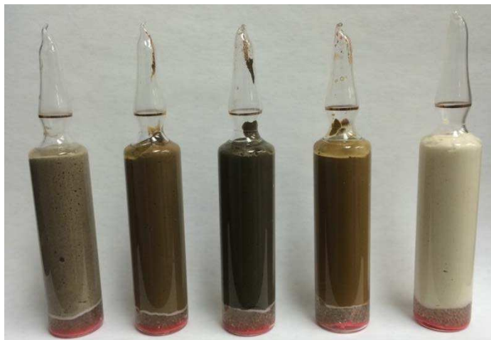
Figure 21. Ampule vial setup with field soils and lab grade soil.
