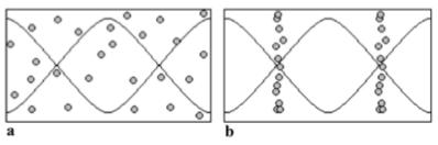
Figure A.1: Acoustophoresis principle diagram.
