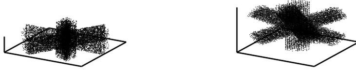
Figure 4.4: Aggregate particle shapes. On the left is a 6-arm particle with arms in a single plane, and on the right is an 8-arm particle with arms oriented spatially.
