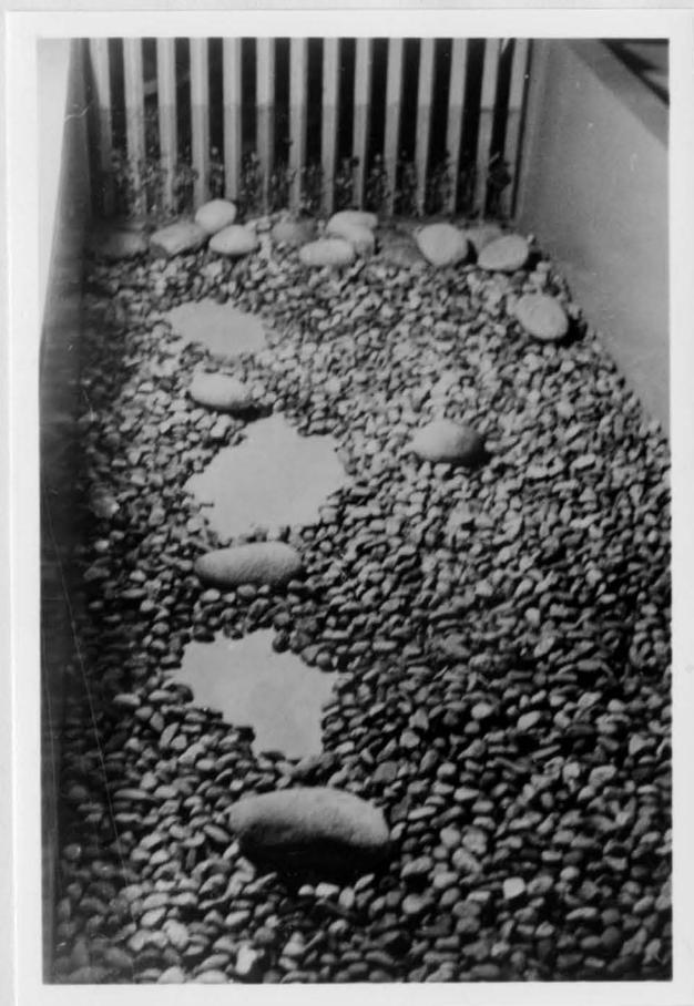
Fig. 15 Movement of bed near entrance of flume which occurred at a slope of  $2\frac{1}{2}\%$
