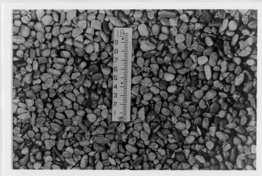
Fig. 14 1-in. gravel after completion of tests
