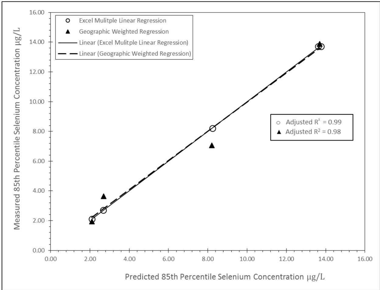
Figure 20 - Measured versus predicted 85th selenium concentration values (µg/L) for Excel multiple linear regression and Geographic Weighted Regression models.
