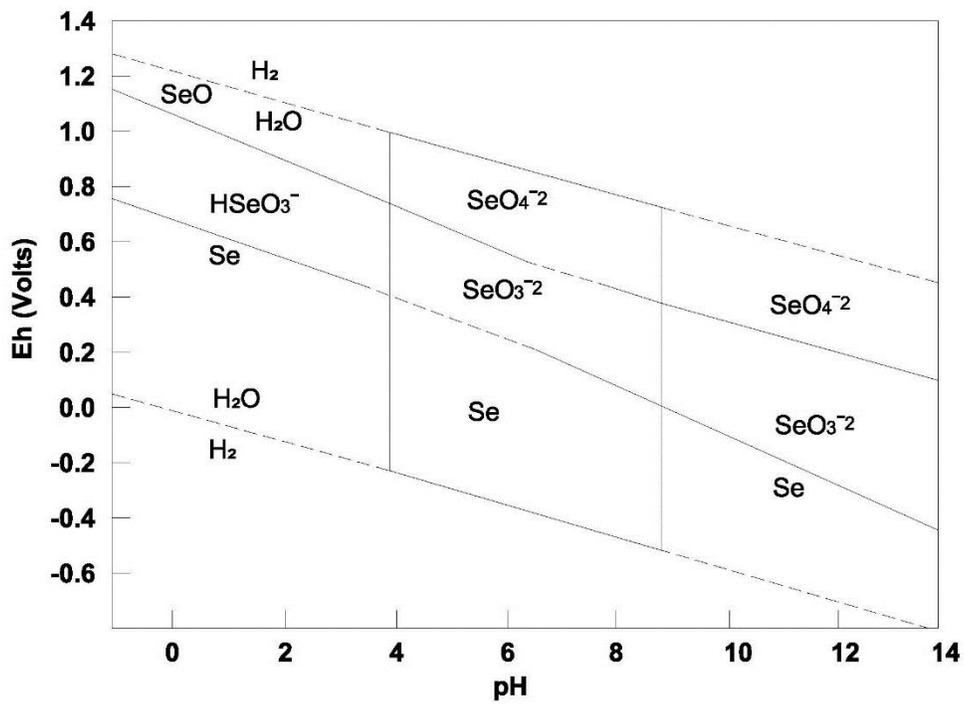
Figure 1 – Eh-pH diagram of Se in soils (from Dissanayake and Chandrajith, 1999)
