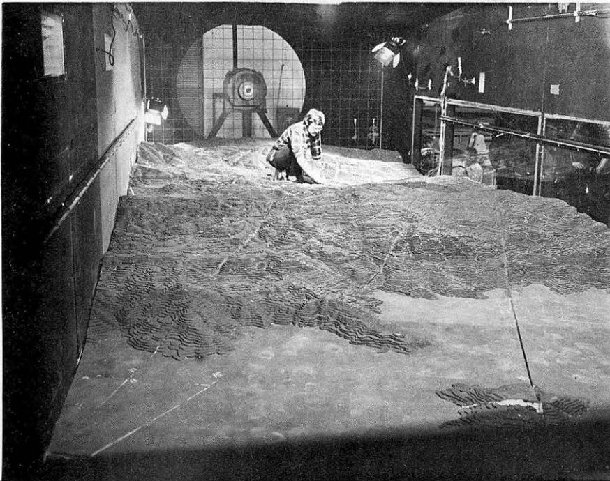
Figure 3.1-2. Photograph of terrain model in the Environmental Wind Tunnel.
