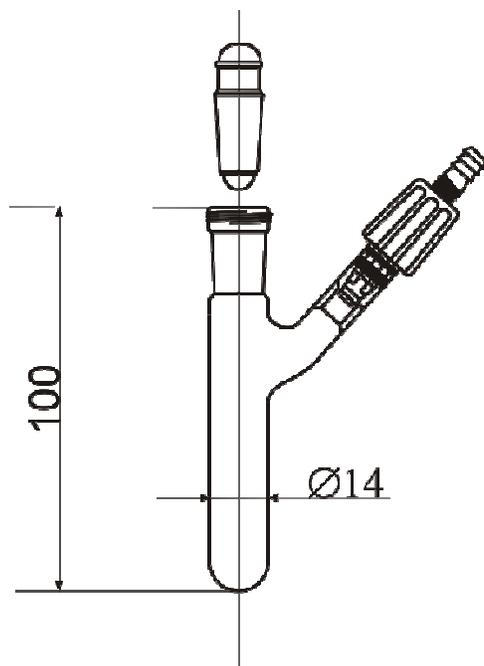
**Figure II.31.** Small-scale greaseless air-free reactor.
