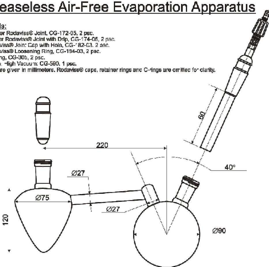
**Figure II.19.** Small-scale greaseless evaporation apparatus.
