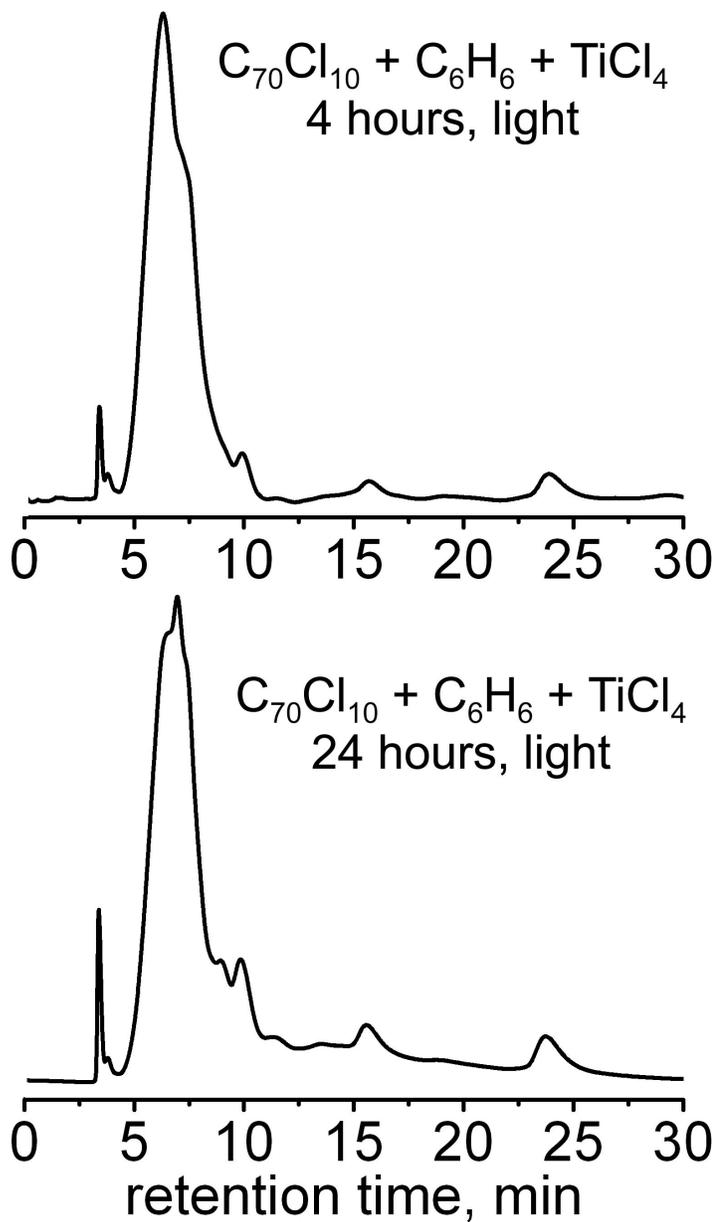
**Figure V.8.** The HPLC analysis of the products of  $C_{70}Cl_{10}$  phenylation in the presence of  $TiCl_4$  catalyst. The traces were acquired using 50/50 v/v toluene/heptane eluent with 5 mL/min flow rate.
