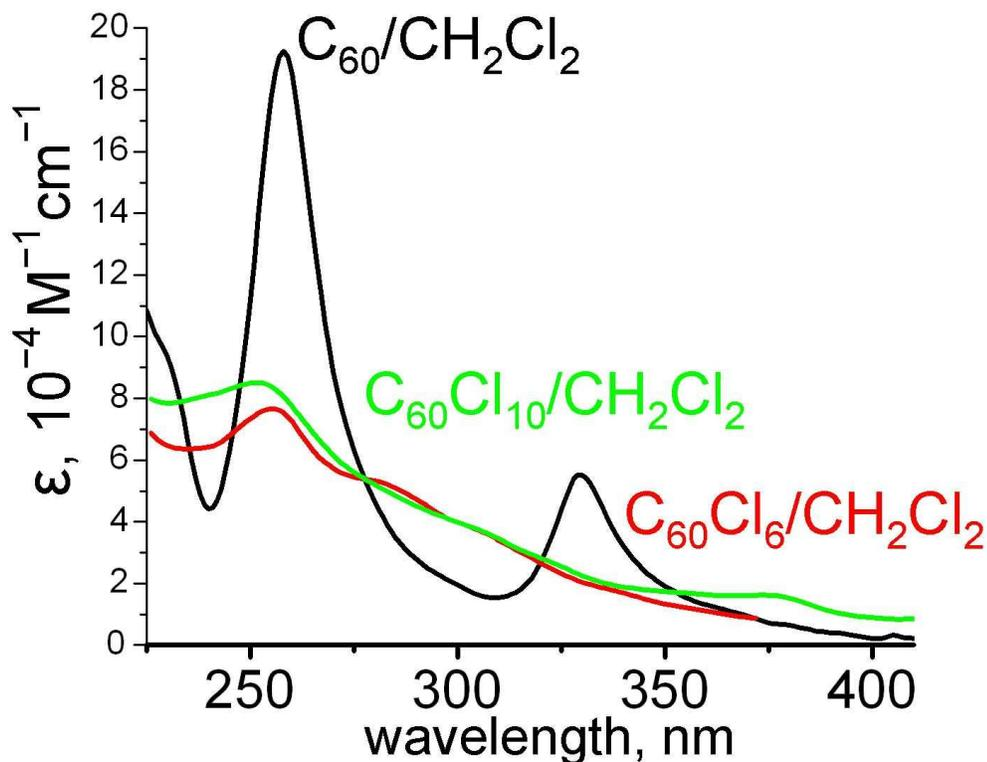
**Figure A.3.** Plots of  $\epsilon(\text{C}_{60})$ ,  $\epsilon(\text{C}_{60}\text{Cl}_6)$ , and  $\epsilon(\text{C}_{60}\text{Cl}_{10})$  vs.  $\lambda$  measured in  $\text{CH}_2\text{Cl}_2$ .
