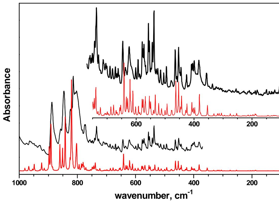
Figure A.10. Expansions of experimental (black) and simulated (red) IR spectra of  $C_{60}Cl_{10}$ .
