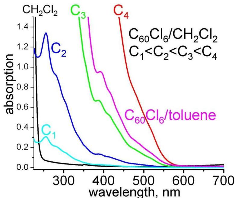
**Figure A.1.** UV-vis spectra of 95%  $C_{60}Cl_6$  in  $CH_2Cl_2$  and toluene solution ( $C_1 < C_2 < C_3 < C_4$  are concentrations of  $C_{60}Cl_6$  in  $CH_2Cl_2$ ). See Table A-1-1 for numerical data.
