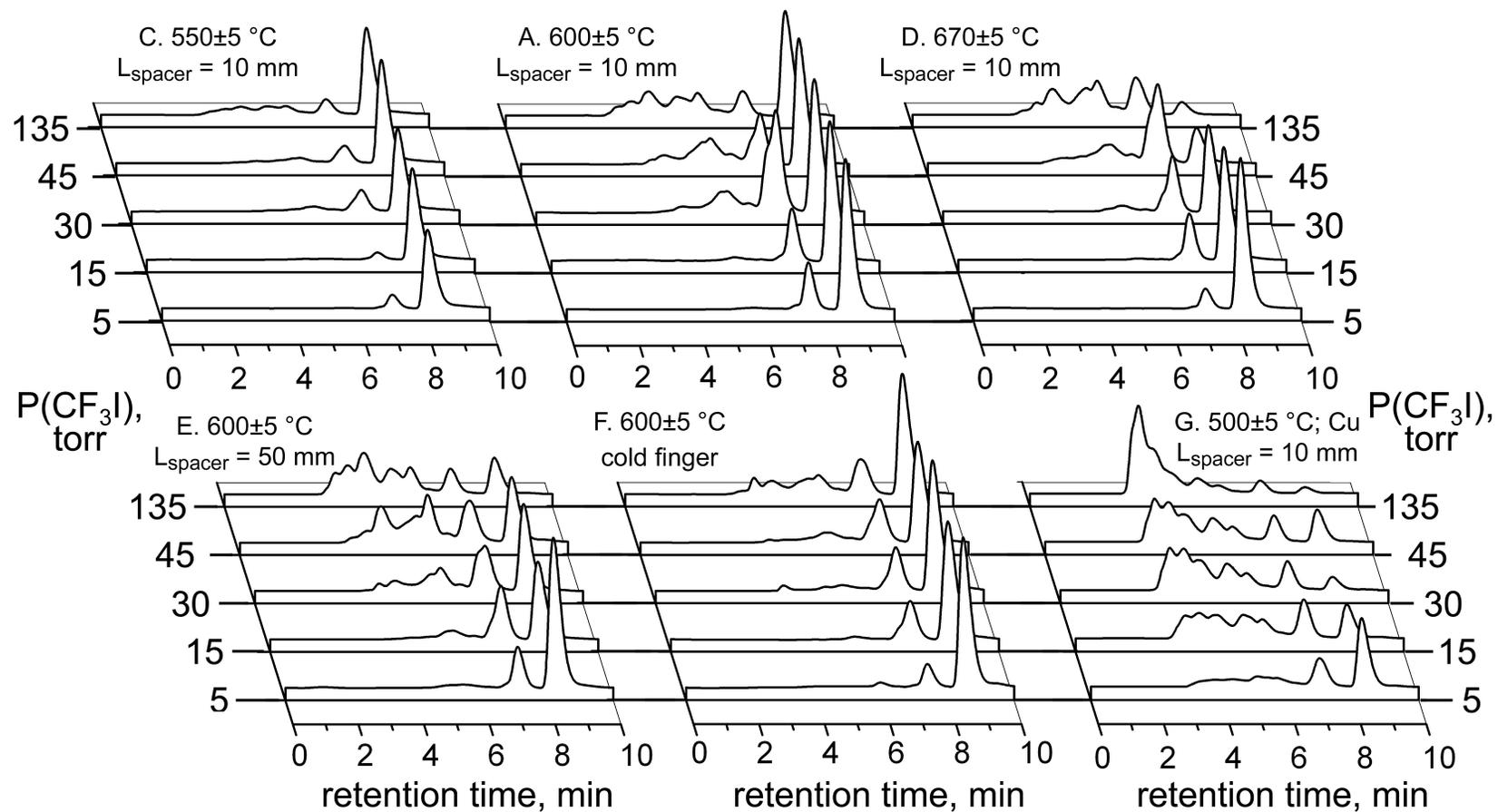
**Figure VII.4.** 3D waterfall plots of the normalized HPLC traces of the products of  $C_{60}$  trifluoromethylation in hot-plate reactor under different conditions (see Table VII.1).
