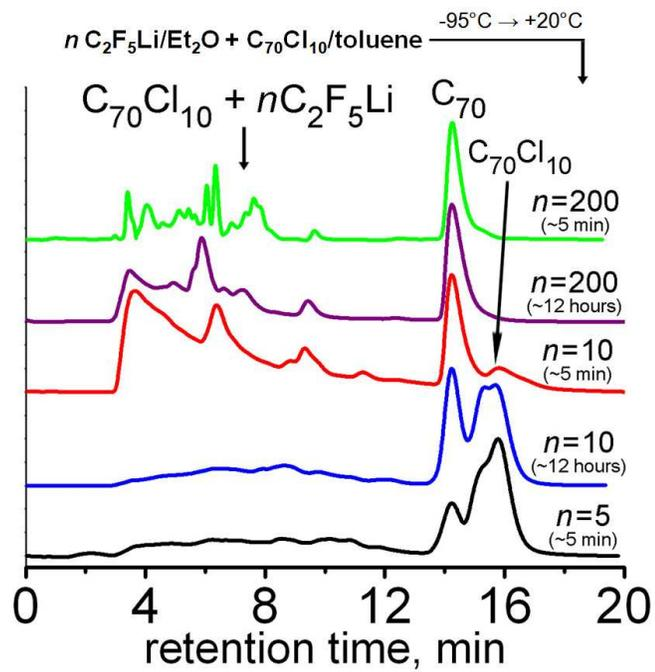
**Figure VI.3.** HPLC analysis of the products of  $\text{C}_{70}\text{Cl}_{10}$  reaction with various amounts of  $\text{C}_2\text{F}_5\text{Li}$  reagent.
