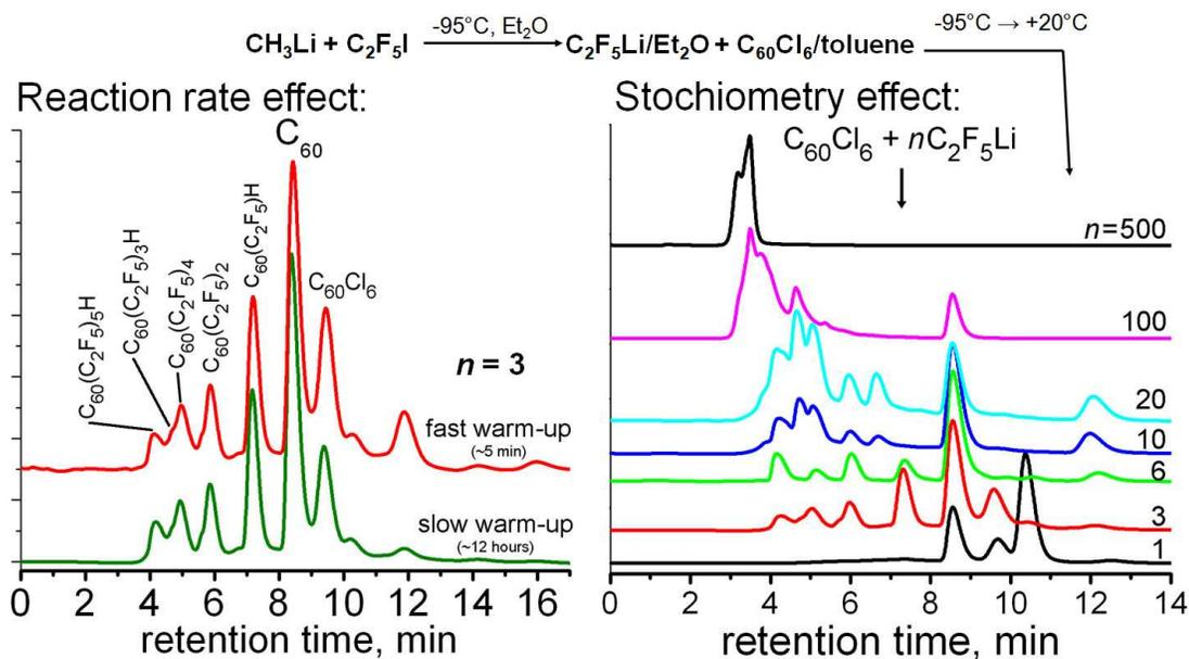
**Figure VI.1.** Effects of reaction rate and stoichiometry on the product distribution of C<sub>60</sub>Cl<sub>6</sub> reaction with C<sub>2</sub>F<sub>5</sub>Li (the HPLC traces of various crude products are shown).
