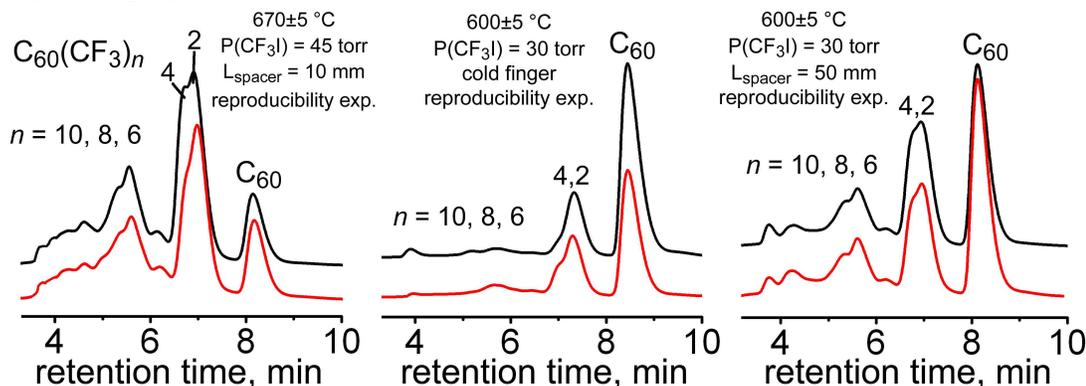
**Figure VII.2.** Experiments on the reproducibility of trifluoromethylation in hot-plate reactor (all experiments were performed for 30 minutes). The red and black lines are the HPLC traces corresponding to different repetitions.
