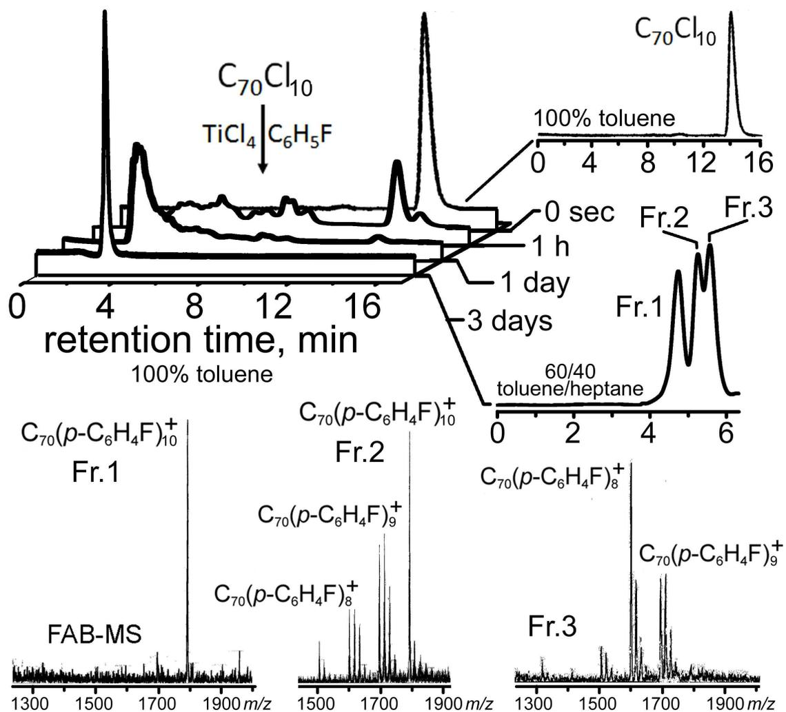
**Figure V.9.** Dynamic HPLC plot of  $C_{70}Cl_{10}$  fluorophenylation. The HPLC trace of the starting  $C_{70}Cl_{10}$  is shown in the top right corner of the figure. The crude reaction mixture after 3 days of the reaction was separated by HPLC and analyzed by FAB-MS, which are shown in the bottom part of the figure.
