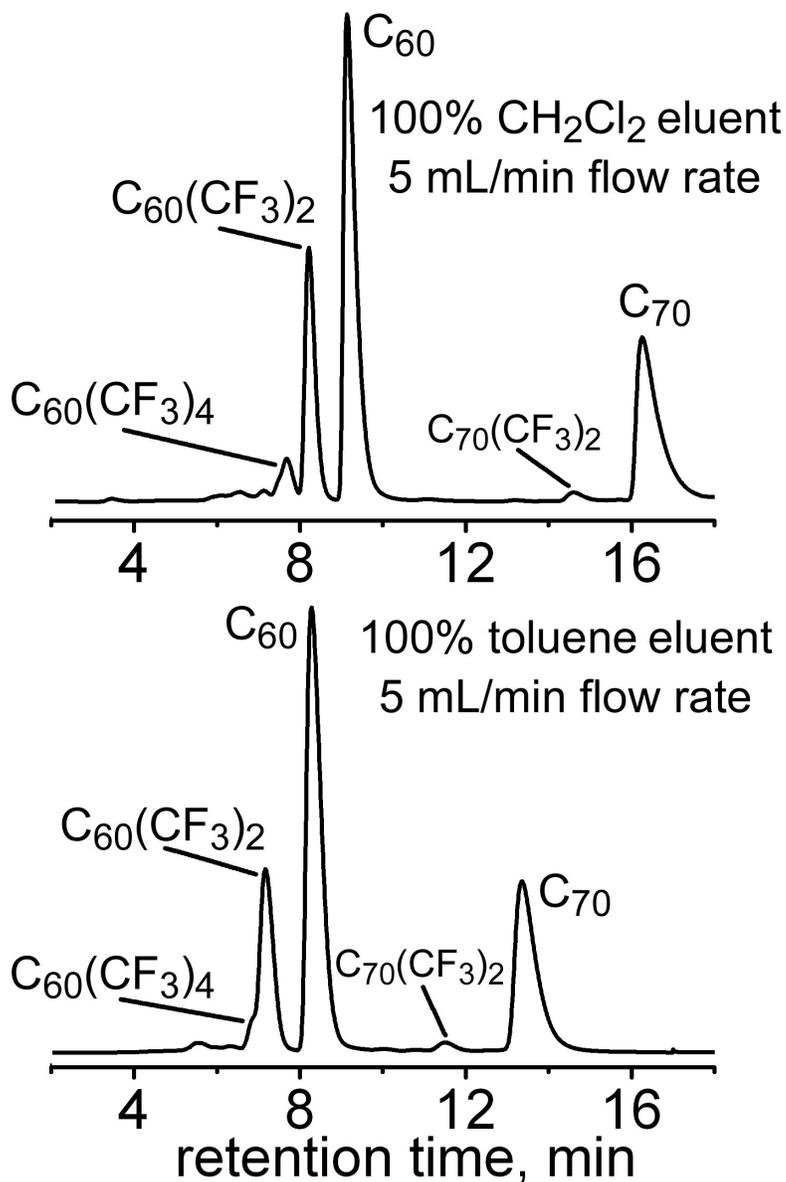
**Figure VII.8.** Large-scale selective synthesis of  $\text{C}_{60}(\text{CF}_3)_2$  from fullerene extract. Top figure shows the HPLC trace acquired using dichloromethane eluent; bottom figure shows the HPLC trace acquired using toluene eluent (same crude product is analyzed in both cases).
