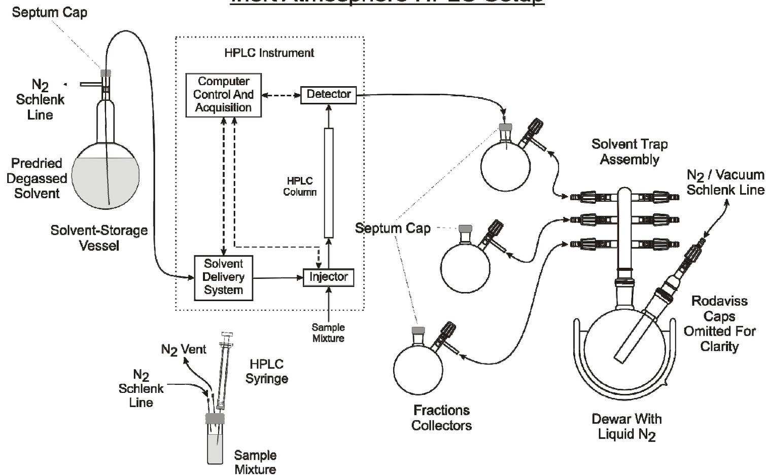
**Figure V.11.** The schematic representation of the inert-atmosphere HPLC setup (see also Figure IV-12). Through the use of protective atmosphere of dry nitrogen, the air-sensitive compounds can be manipulated outside of the glove-box in a convenient benchtop system.
