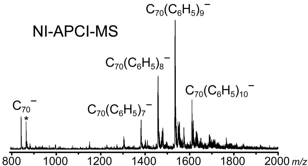
**Figure V.2.** NI-APCI-MS of the sample a (see Figure IV-1). The peak designated with an asterisk is due to a non-fullerene impurity.
