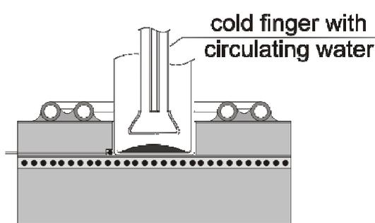
II. Reactor equipped with a cold finger
