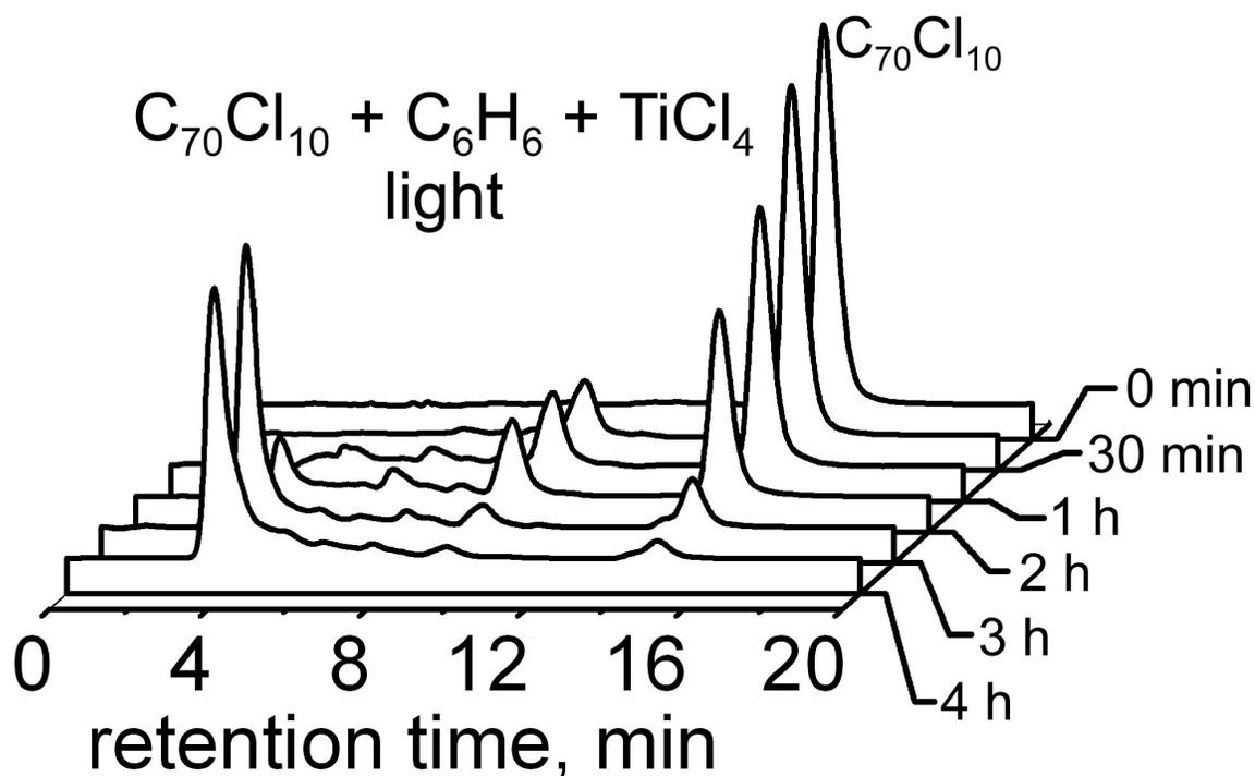
**Figure V.7.** Dynamic HPLC monitoring of  $C_{70}Cl_{10}$  phenylation in benzene solution in the presence of  $TiCl_4$  catalyst.
