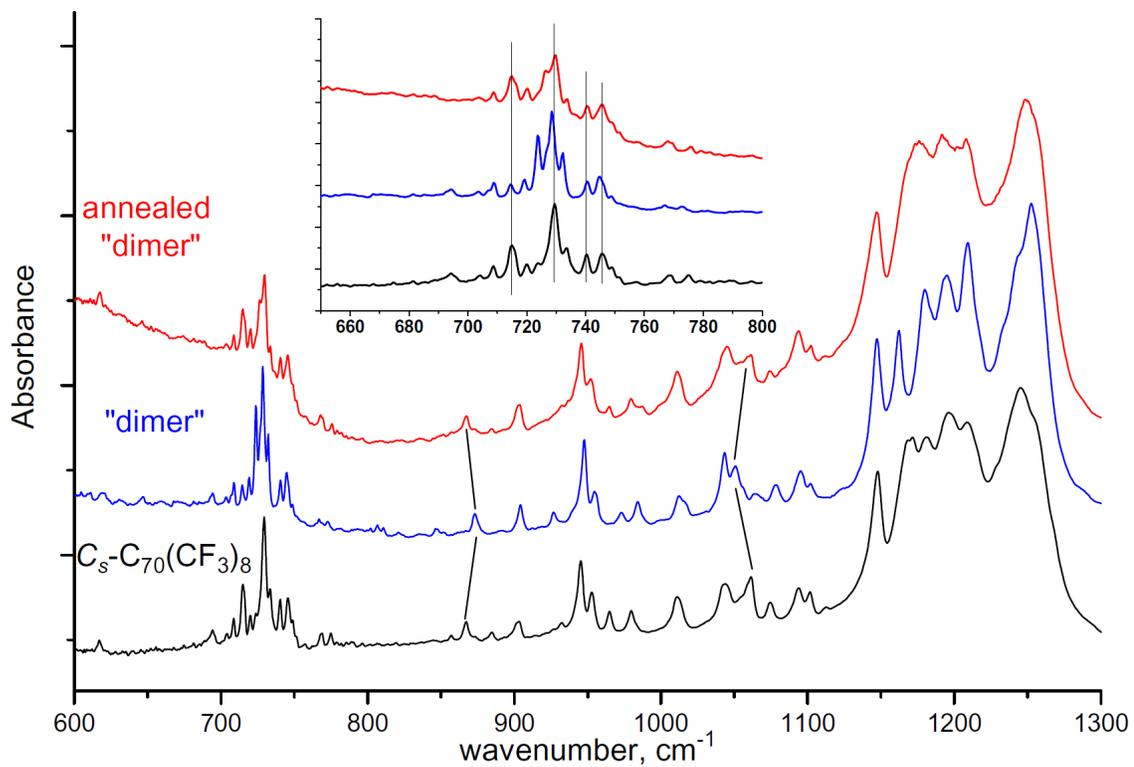
**Figure IV.2.** Experimental IR spectra of monomeric  $C_s$ - $C_{70}(\text{CF}_3)_8$ ,  $[\text{C}_{70}(\text{CF}_3)_8]_2$ ,  $[\text{C}_{70}(\text{CF}_3)_8]_2$  sample after annealing (from bottom to top) showing the changes in the IR signatures of the compounds.
