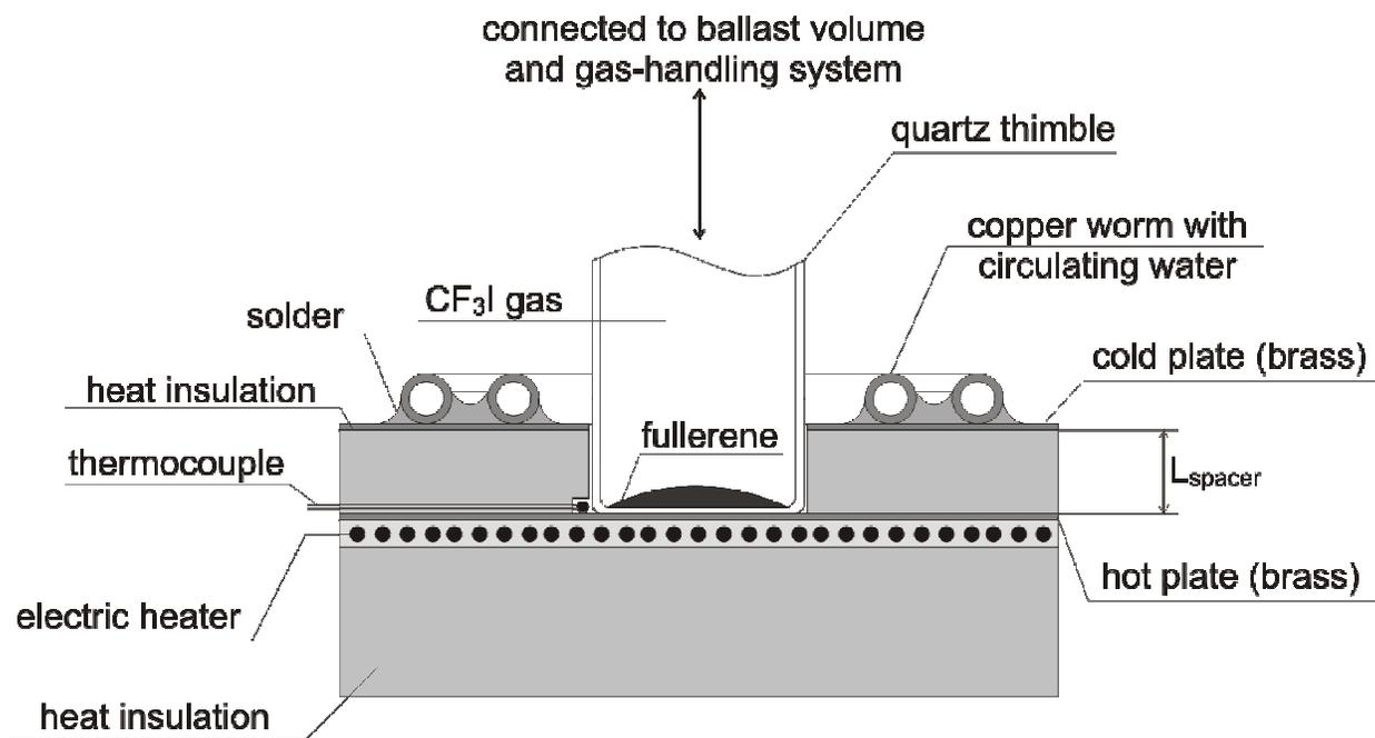
I. Hot-plate reactor (basic configuration)
