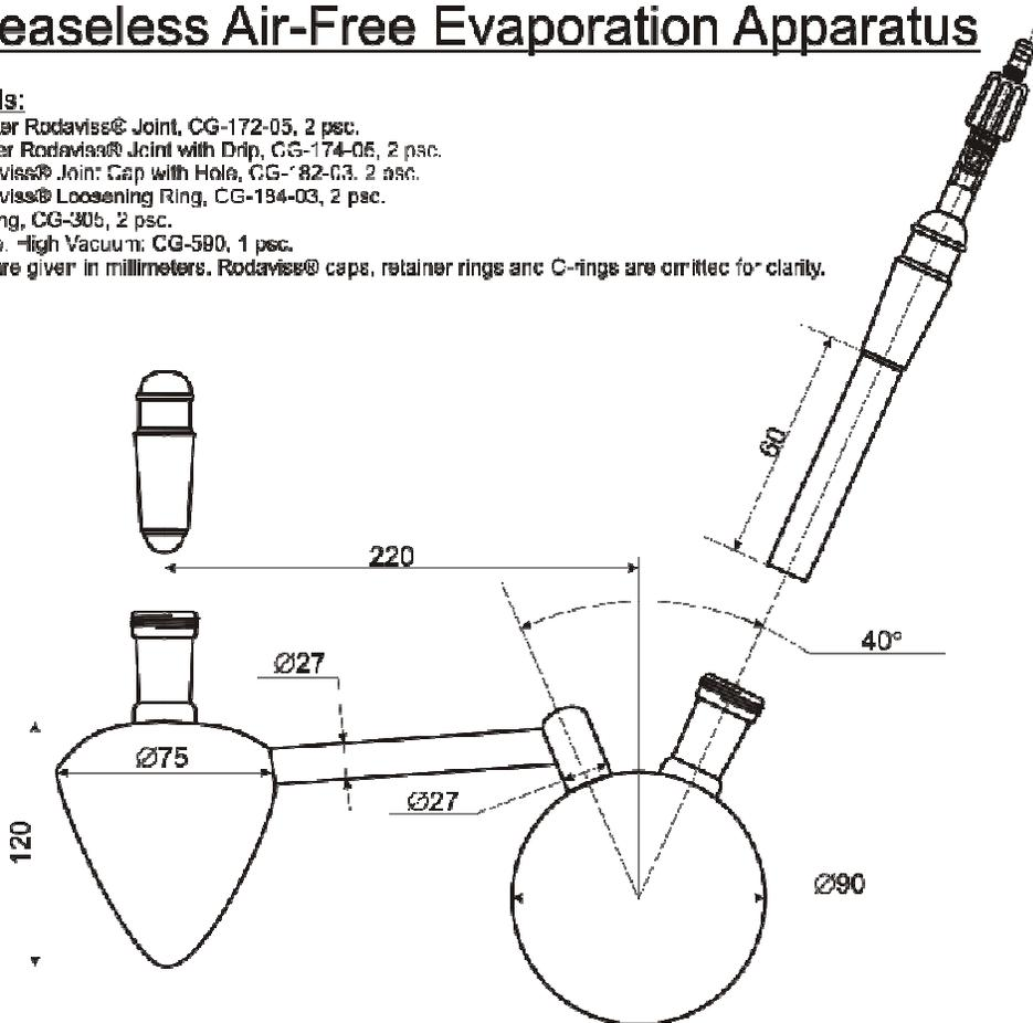
**Figure II.19.** Small-scale greaseless evaporation apparatus.
