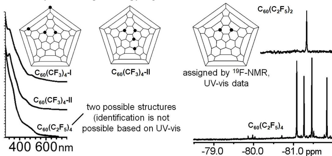
Figure VI.4. Analysis and likely addition patterns of  $C_{60}(C_2F_5)_2$  and  $C_{60}(C_2F_5)_4$ .
