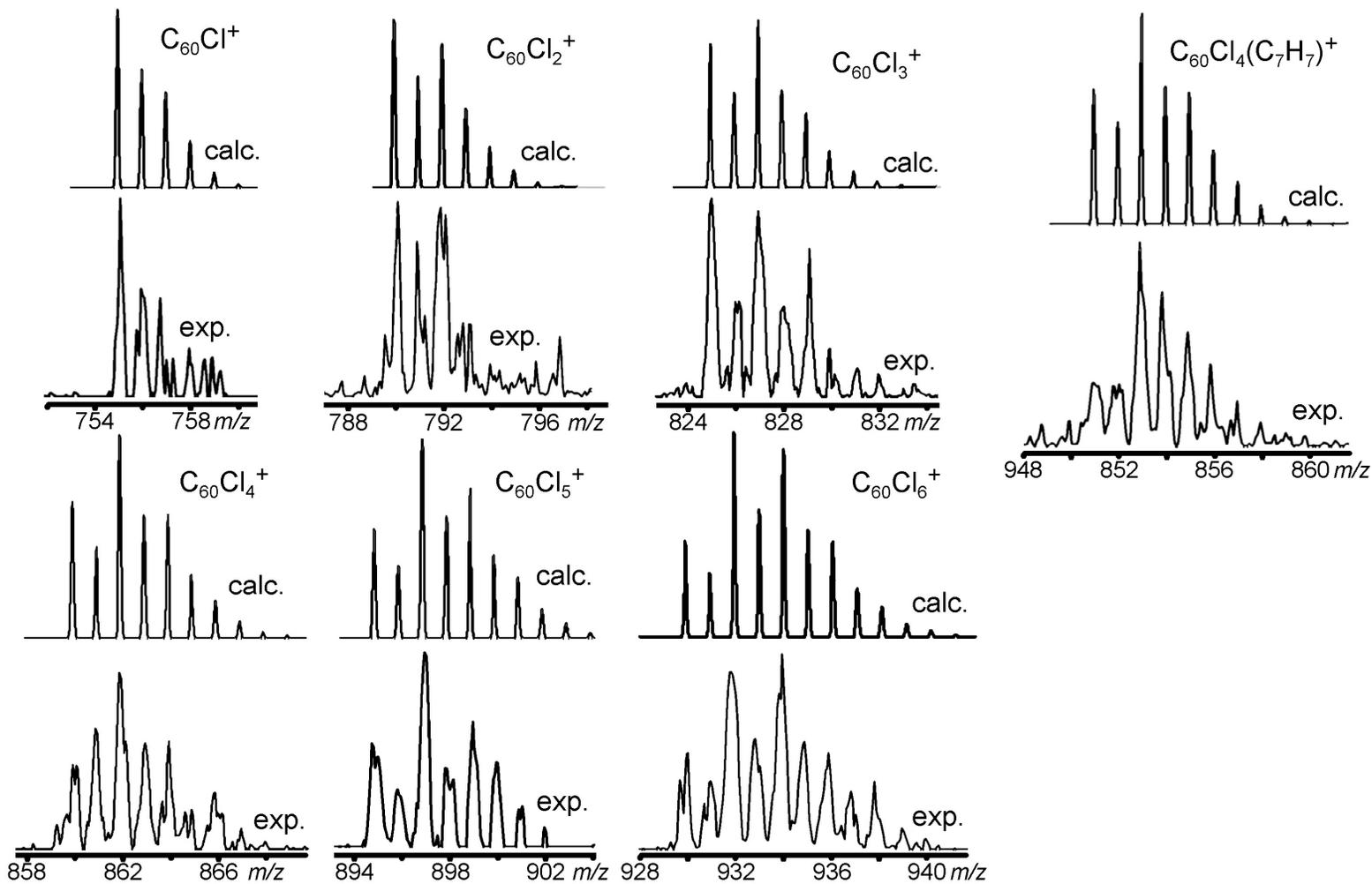
**Figure A.9.** Expansions of the experimental PI-APCI-MS of lower CFs (*o*- $C_{60}Cl_2$ , *p*- $C_{60}Cl_2$ ,  $C_{60}Cl_4$ ,  $C_{60}Cl_6$ ) and calculated isotopic distributions of the corresponding ions.
