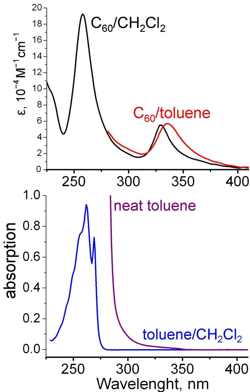
**Figure A.4.** Plots of  $\epsilon(\text{C}_{60})$  vs.  $\lambda$  measured in toluene and  $\text{CH}_2\text{Cl}_2$  versus wavelength (upper figure); UV-vis spectra of neat toluene and toluene solution in  $\text{CH}_2\text{Cl}_2$  (lower figure).
