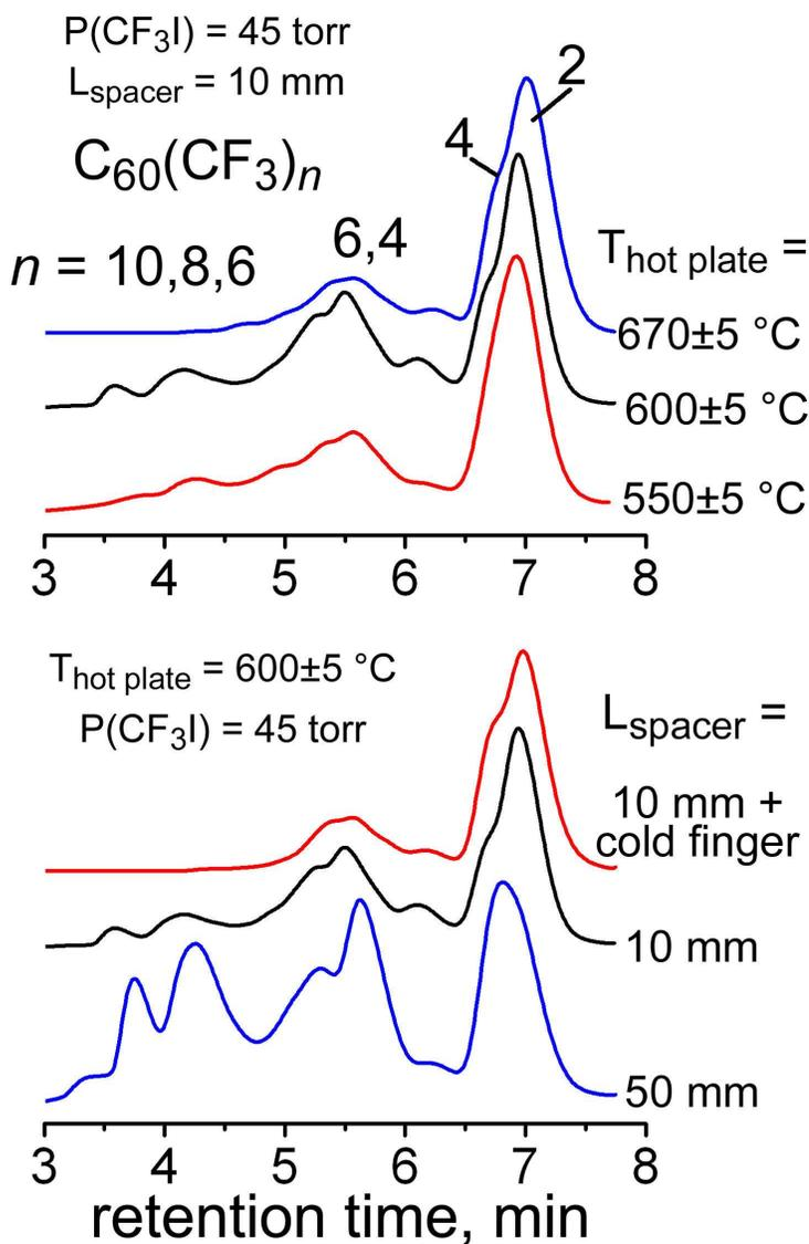
**Figure VII.5.** Comparison of the trifluoromethylation experiments performed at 45 torr of  $\text{CF}_3\text{I}$  at different temperatures (top figure) and different sizes of the hot zones (bottom figure).
