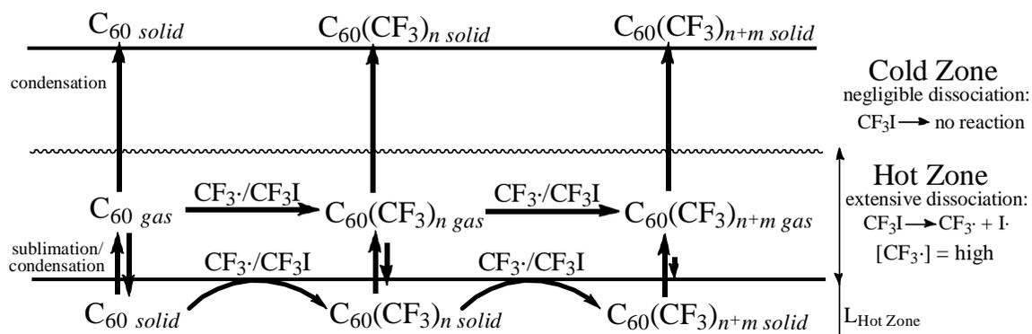
**Scheme VII.1.** The simplified description of the heterogeneous reaction of  $C_{60}$  with gaseous  $CF_3I$  at elevated temperature (without restricting the generality). The formation of molecular iodine and its condensation in the cold zone is not shown.
