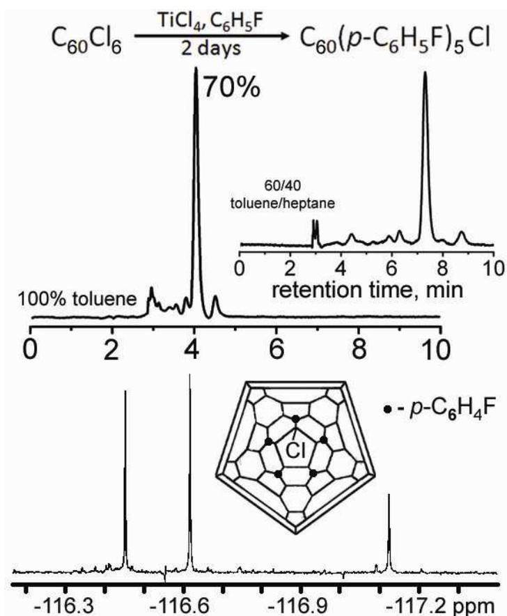
**Figure V.6.** The synthesis, HPLC analysis and  $\{^1\text{H}\}\text{-}^{19}\text{F}$ -NMR spectrum of  $C_{60}(p\text{-C}_6\text{H}_4\text{F})_5\text{Cl}$ .
