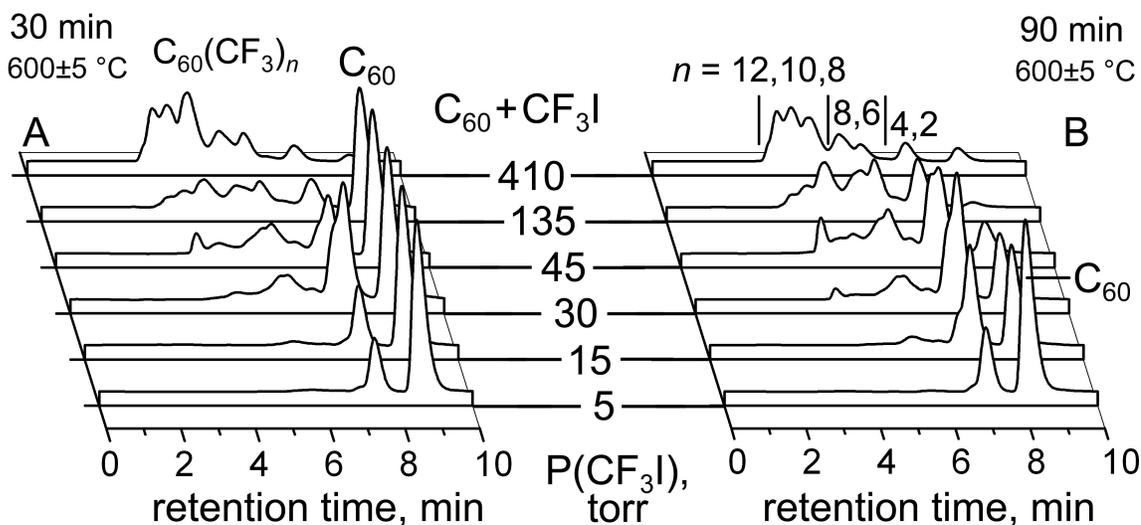
**Figure VII.3.** 3D waterfall plots of the normalized HPLC traces of the products of  $C_{60}$  trifluoromethylation in hot-plate reactor under different pressure of  $CF_3I$ . Sets A and B were performed under the same conditions (see Table VI-1) except for the reaction time (30 min for experiments A and 90 min for experiments B).
