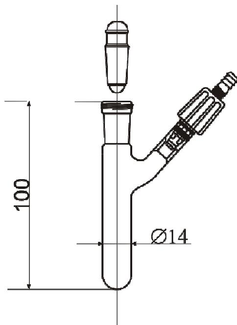
**Figure II.31.** Small-scale greaseless air-free reactor.
