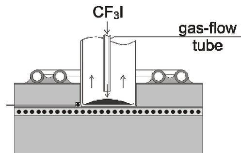
III. Reactor equipped with a flow tube
