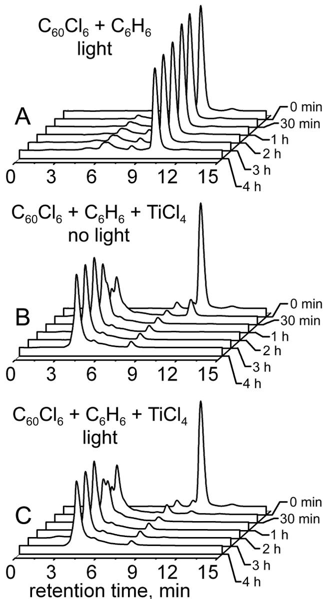
**Figure V.4.** Dynamic HPLC monitoring of  $C_{60}Cl_6$  phenylation in benzene solution in the presence of  $TiCl_4$  catalyst. The reaction mixtures A, B, and C were kept at the same distance from the light source to ensure that their temperatures are the same. The flask containing reaction mixture B was shielded from light by aluminum foil wrap.
