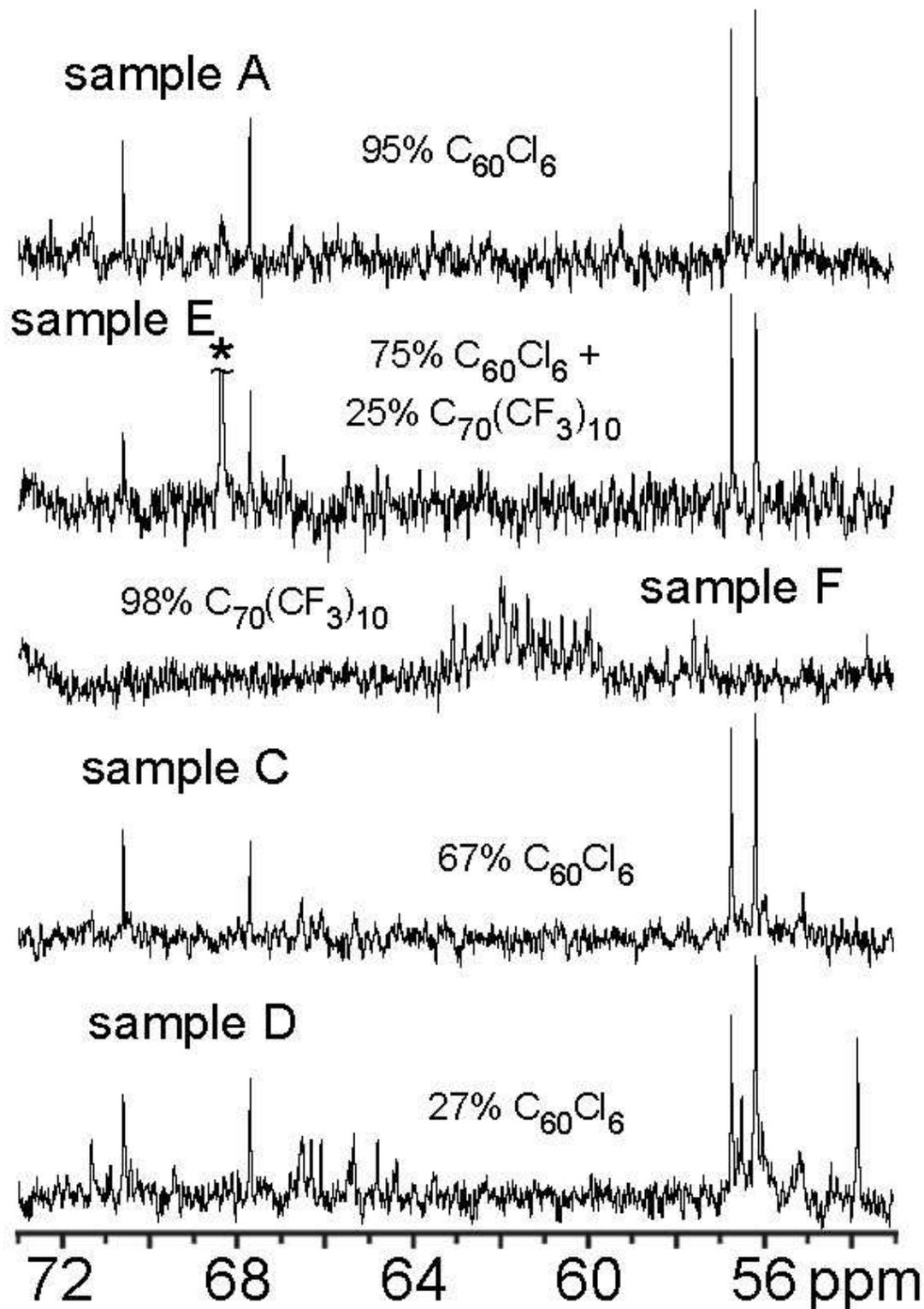
**Figure A.6.**  $^{13}C$  NMR spectra of  $C_{60}Cl_6$  samples A, C, D, E, and  $C_{70}(CF_3)_{10}$  sample F. Peak marked with an asterisk is due to unidentified impurity.
