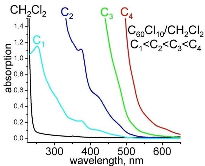
**Figure A.2.** UV-vis spectra of 98%  $C_{60}Cl_{10}$  in  $CH_2Cl_2$  ( $C_1 < C_2 < C_3 < C_4$  are concentrations of  $C_{60}Cl_{10}$  in  $CH_2Cl_2$ ). See Table A.4 for numerical data.
