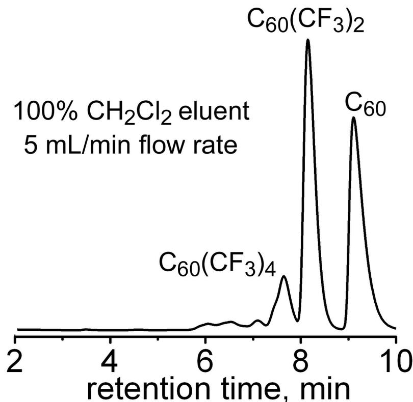
**Figure VII.7.** Large-scale selective synthesis of  $C_{60}(CF_3)_2$  (100 mg  $C_{60}$  sample was used).
