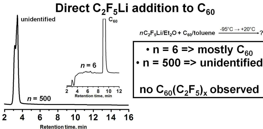
**Figure VI.2.** Direct addition of C<sub>2</sub>F<sub>5</sub>Li to C<sub>60</sub>. HPLC traces of the corresponding crude products are shown.
