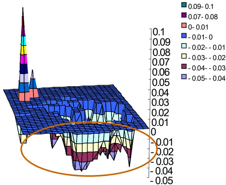
Figure 6. Distributed Source-Sink term ( $\text{m.d}^{-1}$ ) on 15<sup>th</sup> of April 1993, excessive pumping at the beginning of irrigation season caused severe water shortage
