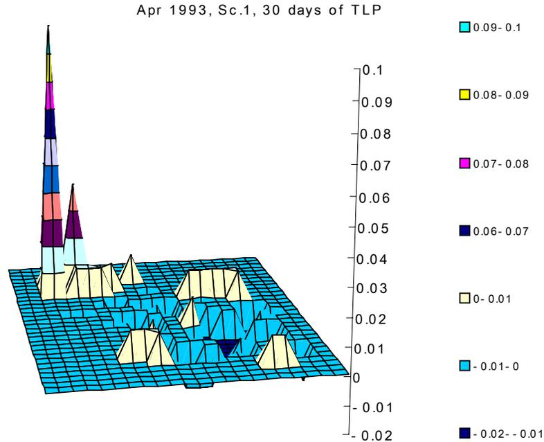
Figure 7. Simulated distributed Source-Sink term ( $m.d^{-1}$ ) on 15<sup>th</sup> of April 1993, using a period of 30 days for transplanting and land preparations
