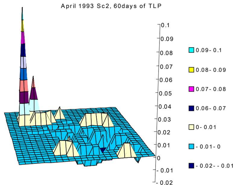
Figure 8. Simulated distributed Source-Sink term ( $\text{m.d}^{-1}$ ) on 15<sup>th</sup> of April 1993, using a period of 60 days for transplanting and land preparations
