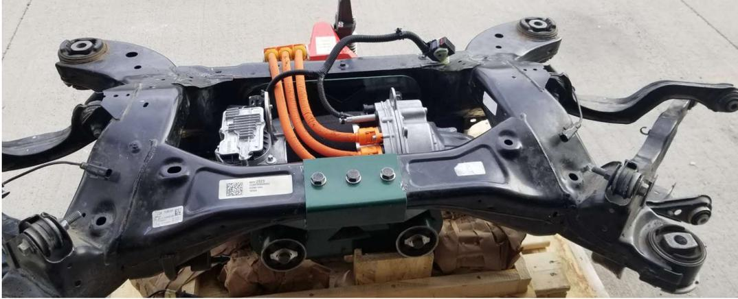
*Figure 20: Blazer rear subframe with Magna eRAD installed*
