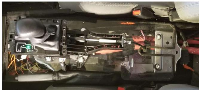
*Figure 30: Transmission tunnel hole with acrylic cover*
