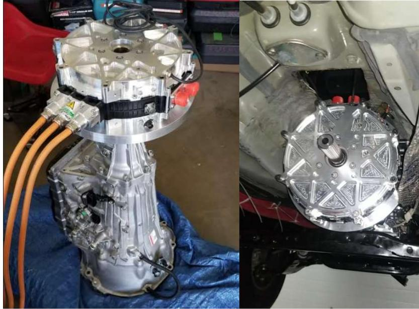
*Figure 21: YASA P400 Installed on the Tacoma Transmission (left) and Transmission/ EM System Installed on Vehicle (right)*
