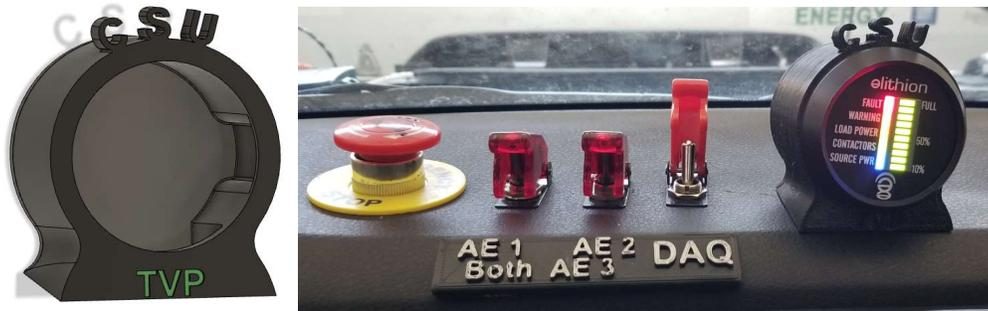
*Figure 25: CAD model of the battery gauge (left) and 3D printed part with the battery gauge installed on the dashboard along with the PAE switches, EDS, and gateway power switch(right)*
