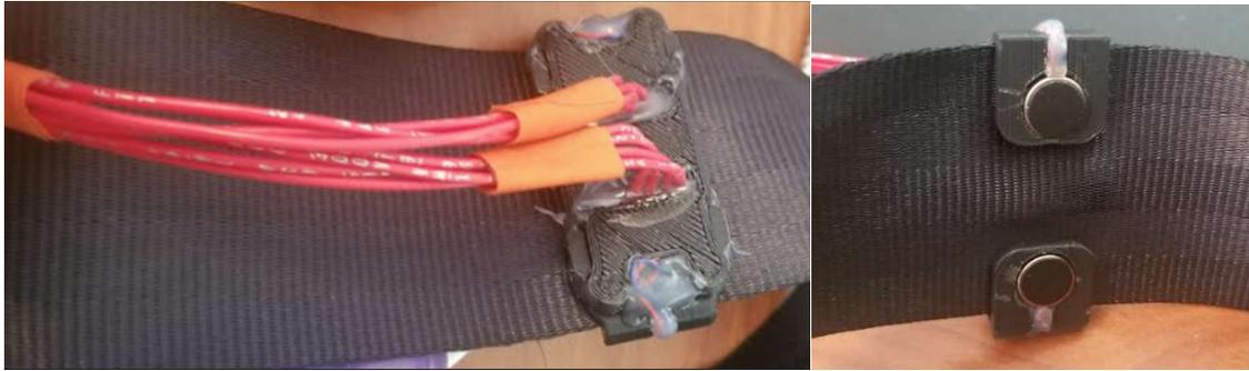
*Figure 24: Haptic feedback system shown installed on the seatbelt with the top view (left) showing the connecting wires and the bottom view (right) showing the haptic motors*
