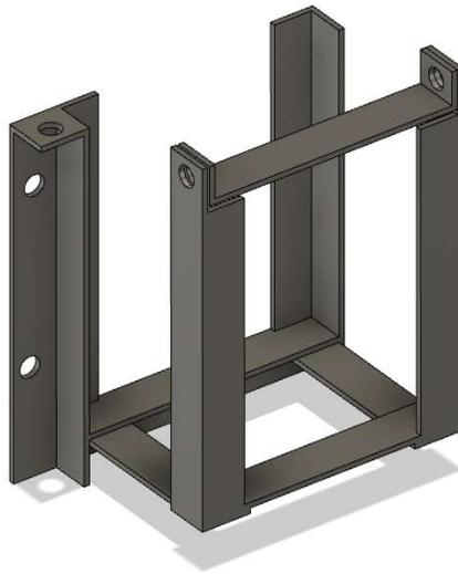
*Figure 28: TVP antifreeze reservoir mount with battery box rear mounting holes shown*
