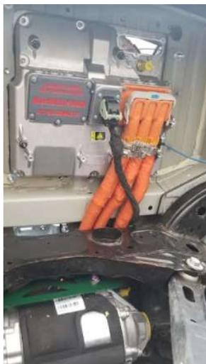
*Figure 6: Inverter installed into the rear spare tire well of the Blazer as seen from the underside of the vehicle*
