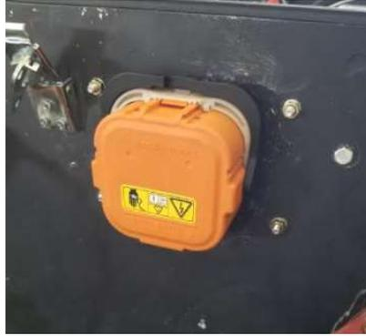
*Figure 8: Manual Service Disconnect inserted into the receptacle on the TVP*
