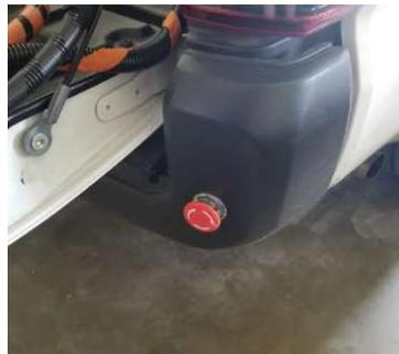
*Figure 19: Emergency disconnect switch installed on the rear bumper*
