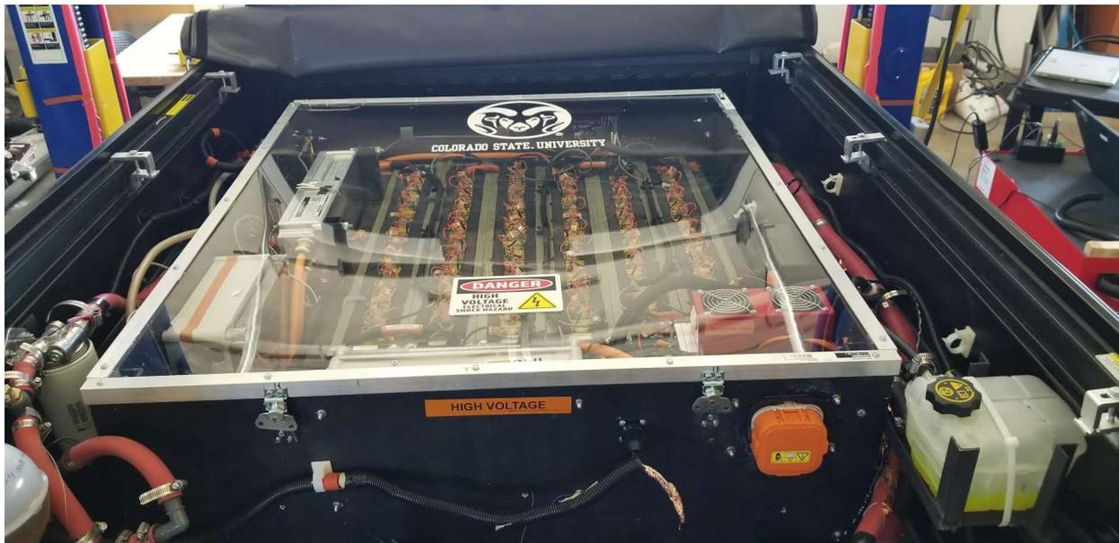
*Figure 11: Battery box installed in the bed of the Tacoma with the protective plastic lid shut*
