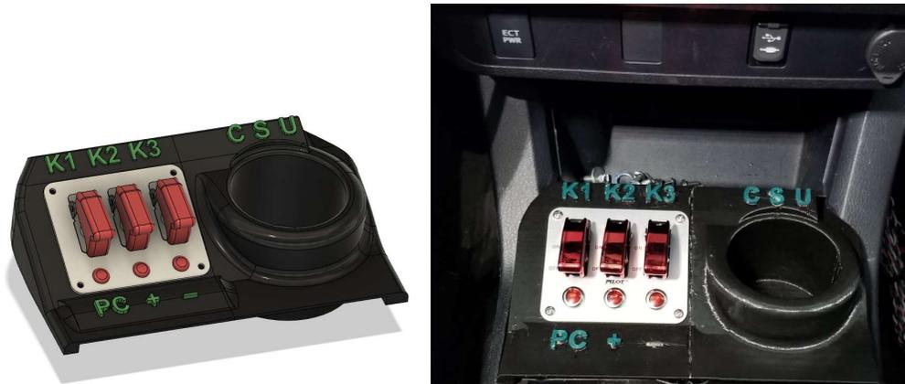
*Figure 26: Contactor control switches CAD model mount (left) and 3D printed part installed in the vehicle*
