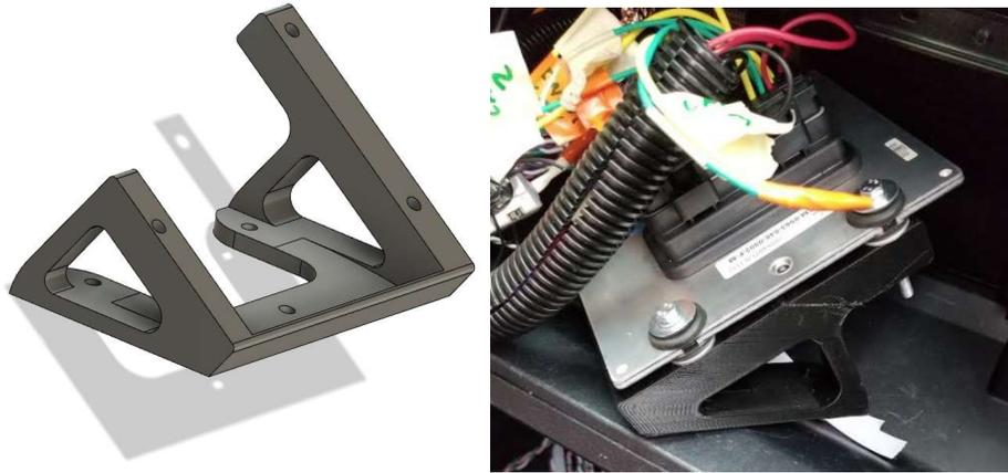
*Figure 29: CAN gateway mount CAD (left) and 3D printed part with the gateway installed (right)*
