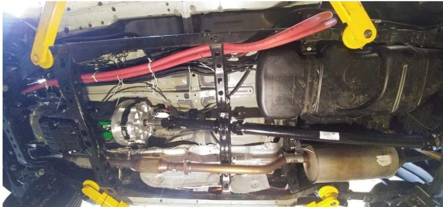
*Figure 22: Electric motor, transmission, and propulsion shaft installed in vehicle*
