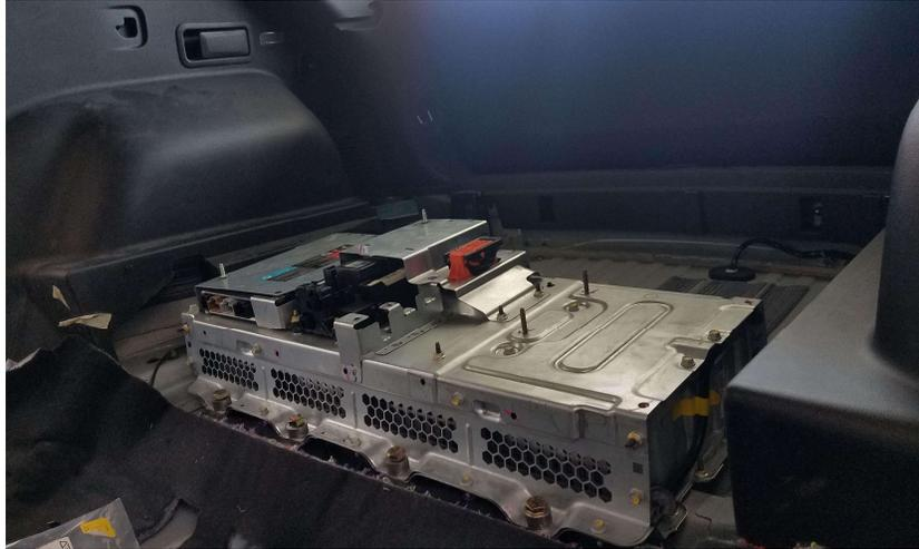
*Figure 5: HEV 4 installed in the rear spare tire well of the Blazer (APM not shown)*
