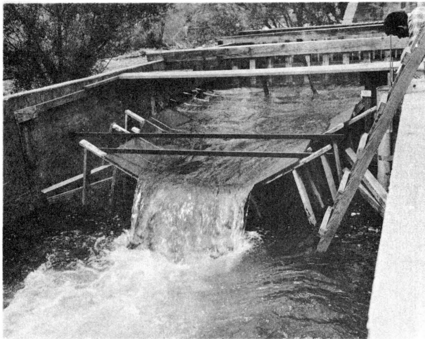
Fig. 5. Model with 120^{\circ} V-notch Weir on Downstream End. Lower View Prototype Discharge 98 cfs.
