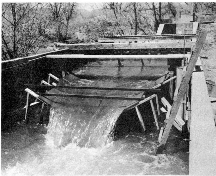
Fig. 4. 1:2 Model of the Forest Service Flume Model Discharge 29.0 cfs, Prototype Discharge 164 cfs.
