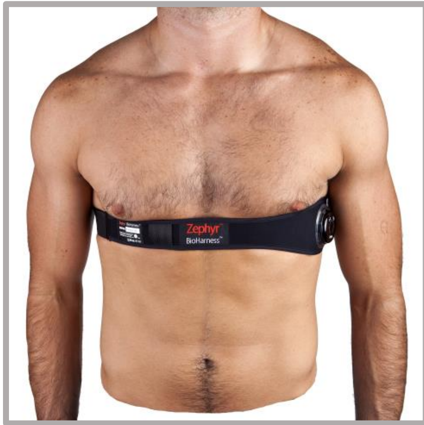
Figure 1. Placement of the Zephyr BioHarness (modules are placed over the left ribs)
