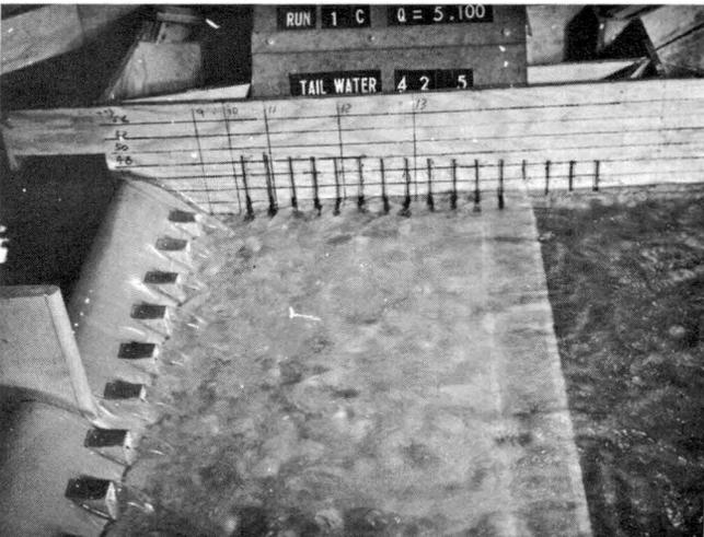
Figure 10a. Photograph of modified stilling basin (apron length reduced 10 ft.),  $Q = 5,100$  cfs, tailwater elevation = 42.5
