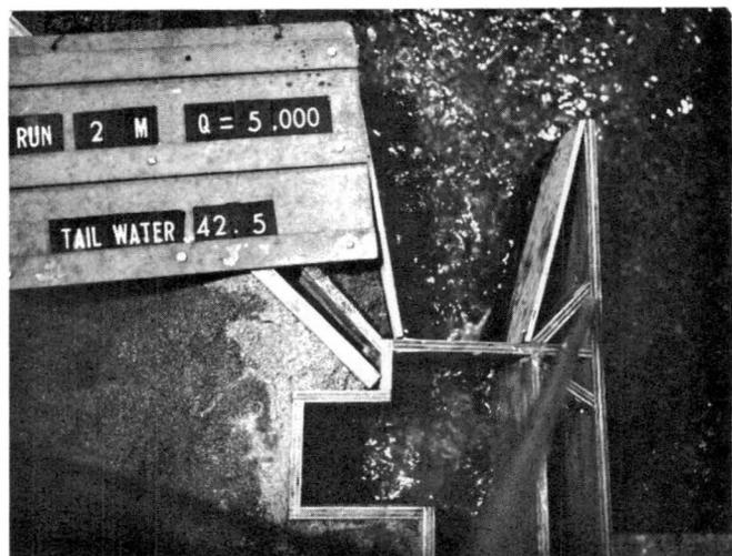
Figure 18. Fish trap outlet with  $20^\circ$  flared walls,  $Q = 5,000$  cfs, tailwater elevation = 42.5
