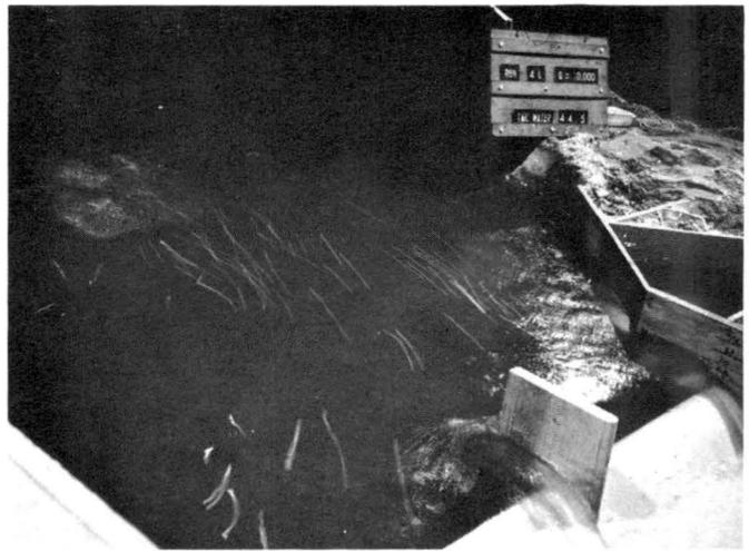
Figure 15b. Approach flow patterns with spillway axis skewed,  $Q = 10,000$  cfs, skew angle =  $20^\circ$
