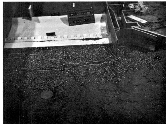
Figure 22c. Scour downstream from stilling basin with apron length reduced 12 ft. and dentated end sill #2 installed,  $Q = 15,000$  cfs, tailwater elevation = 45.5
