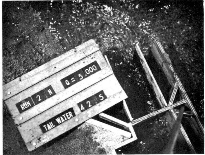
Figure 17. Fish trap outlet with parallel walls,  $Q = 5,000$  cfs, tailwater elevation = 42.5
