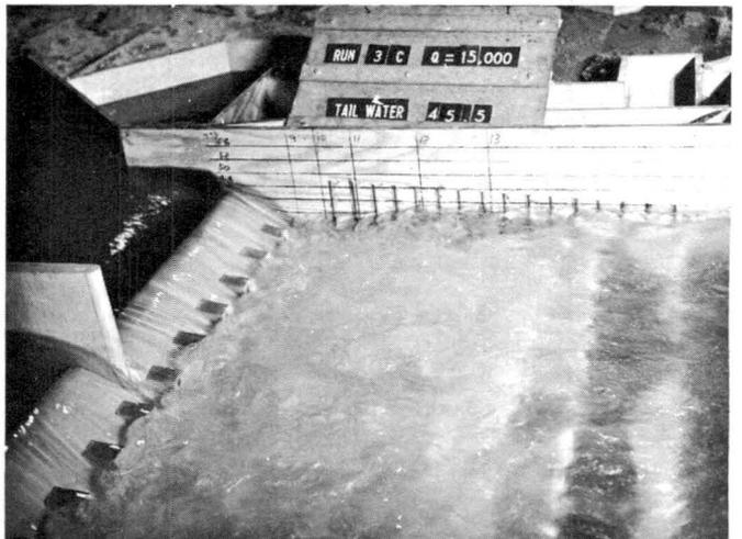
Figure 10b. Photograph of modified stilling basin (apron length reduced 10 ft.),  $Q = 15,000$  cfs, tailwater elevation = 45.8
