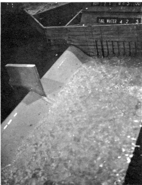
Figure 12a. Photograph of modified stilling basin (apron length reduced 12 ft. and chute blocks removed),  $Q = 5,100$  cfs, tail-water elevation = 42.5
