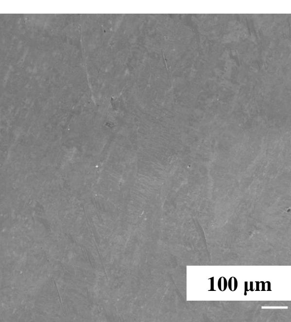
The atomic composition & morphology of Pt foil remained unchanged after N<sub>2</sub>O plasma exposure.
