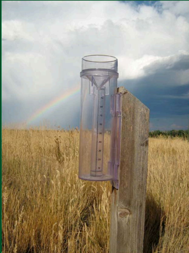
4-inch diameter High capacity rain gauges
