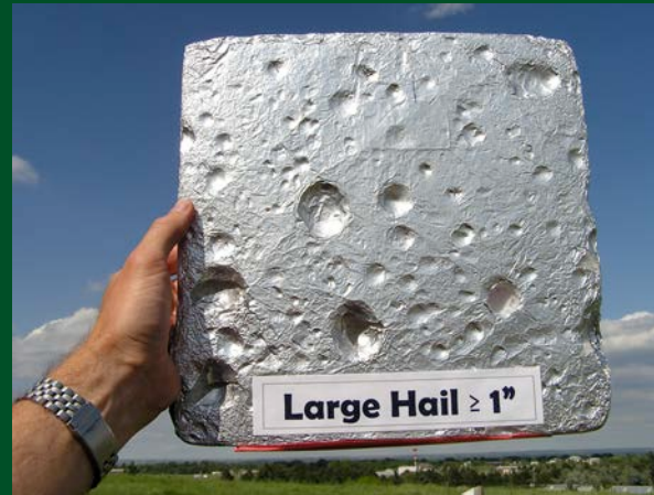
Aluminum foil-wrapped Styrofoam hail pads
