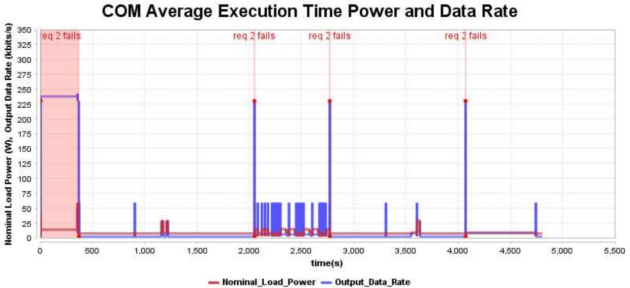
**FIGURE 58. MBSE EXAMPLE OF COM OUTPUT DATA RATE FAILING REQUIREMENT WITH AN ARTIFICIALLY INCREASED OUTWARD VISION SYSTEM OUTPUT DATA RATE TO DEMONSTRATE AUTOMATIC REQUIREMENTS VERIFICATION USING THE MBSE TOOL. THE SHADED REGIONS OF THE PLOT LABELED “REQ 2 FAILS” INDICATES WHEN THE COM OUTPUT DATA RATE REQUIREMENT (REQUIREMENT ID “2”) WAS NOT MET DURING THE SIMULATION.**
