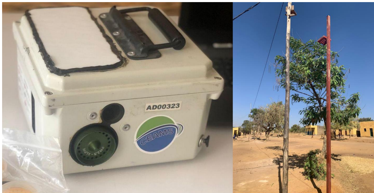
Figure 2.6: AMOD and Sampling Location. On the left is an image of one of the modified AMODs (with the AOD turret covered) used for ambient PM 2.5 monitoring. The dark-green circle at the front of the unit is the size-selective ( d_p < 2.5 \mu\text{m} ) cyclone inlet that sits in front of the PTFE filter for collecting gravimetric samples. The black inlet on the left face of the unit is the real-time PM 2.5 light scattering sensor port. The right side of the figure shows one of the original wooden sampling poles and its replacement metal pole used to hold the units ~4 m above the ground while sampling. The AMODs were set up on wooden poles for the first 5 months of the study before getting replaced by metal ones to ensure greater longevity for the remainder of the 3-year study.
