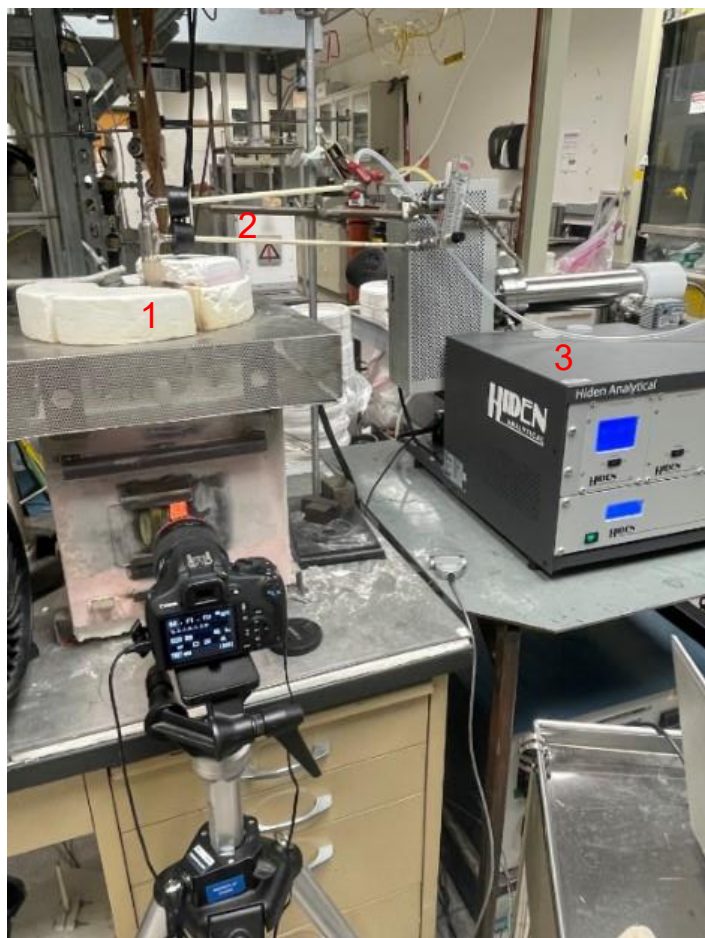
Figure 8: EGA setup 1) Furnace, 2) non-heated transfer line, 3) EGA instrument
