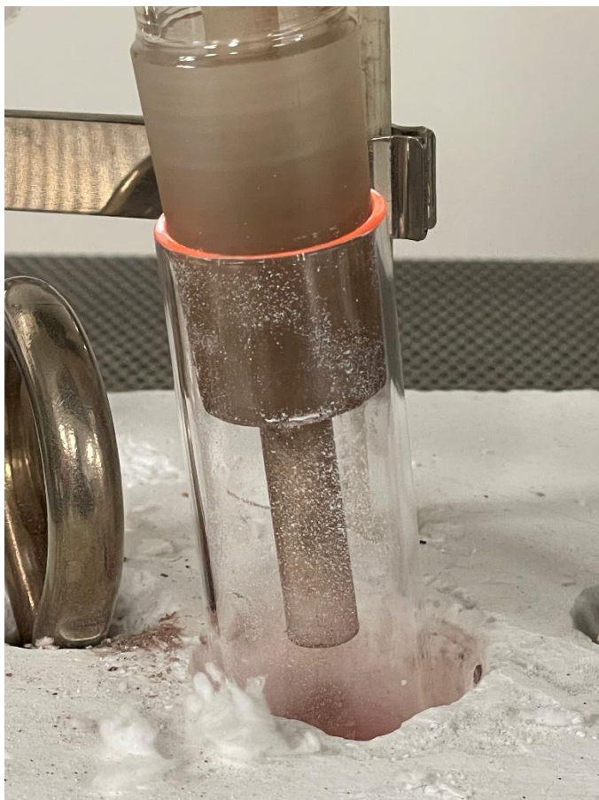
Figure 27: Recondensed salt on the air exposed quartz tube prior to reaching the heated capillary line.
