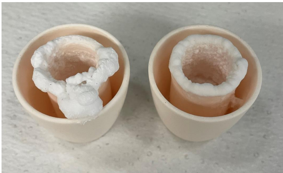
Figure 37: Resulting \text{KMgCl}_6931 after benchtop geometric pycnometry experiment.
